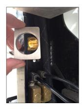
This aluminum spacer is designed to level the bulkhead fitting to the same level as the additional support plate found behind the 1 1/8" hole you drilled. On some installations, it may not be needed.
