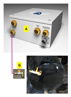
For the "AIR" connection, run 3/8" DOT tubing from the Main Box (A) to a DOT fitting installed into the secondary air tank on the vehicle. An air loss limit valve (not included) may be used to limit air loss in the unexpected the tube gets torn off. The air valve on the main Control Box (A) should stay in the OFF position. The air valve is used only for winterization purposes to blow out the supply lines.
