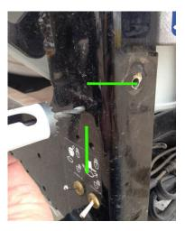
Carefully drill the hole using a 1 1/8" hole saw. Notice above- the hole is closer to the front edge than the center to avoid the additional support plate inside. Also, it is low enough to avoid interfering with the bolt hole which holds the cover plate in place.
