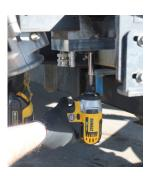
Remove the existing two bolts holding in the Grease port to the bottom of the Auto-wind block. Insert the new aluminum block included with the Vanguard System with the Grease port back in place. Secure the new block with the two new bolts included. The new bolts are 1" longer than the ones removed to accommodate block thickness.
