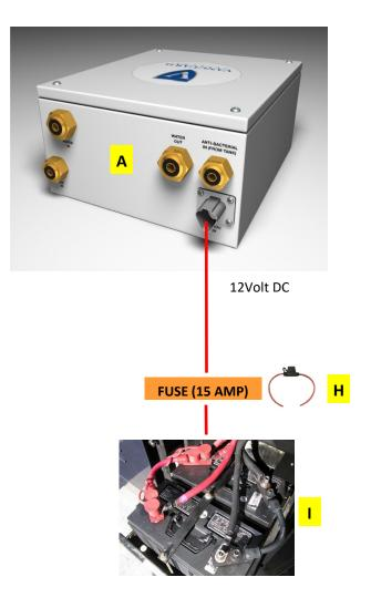
The Electrical input is for 12V DC only. Some models have a automatic heat element which automatically turns on in freezing conditions to protect the main water pump. The system must be wired in such a way (battery direct) for the heat to be activated automatically.
