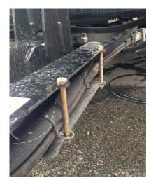
Install the 1/2" tube (with the covering already installed) following the main hose bundle along the same path under the truck chassis. This allows for free movement of the newly installed components. Secure it along this path with the included zip ties. Attach this end to the NEW Valve assembly fitting installed.
