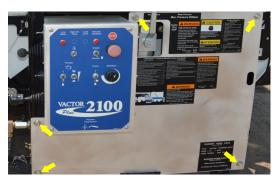
Start by removing the 5 bolts which hold the front aluminum cover in place.
