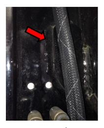
IMPORTANT NOTE: After removing the front cover find the THICK support plate and internal fittings. You don't want to drill your hole into either of them.
