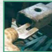
*Six point helical test for weld integrity*
