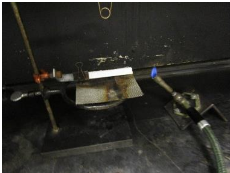
Photo No. 2 ASTM D635 Test Setup, Pre-Test
