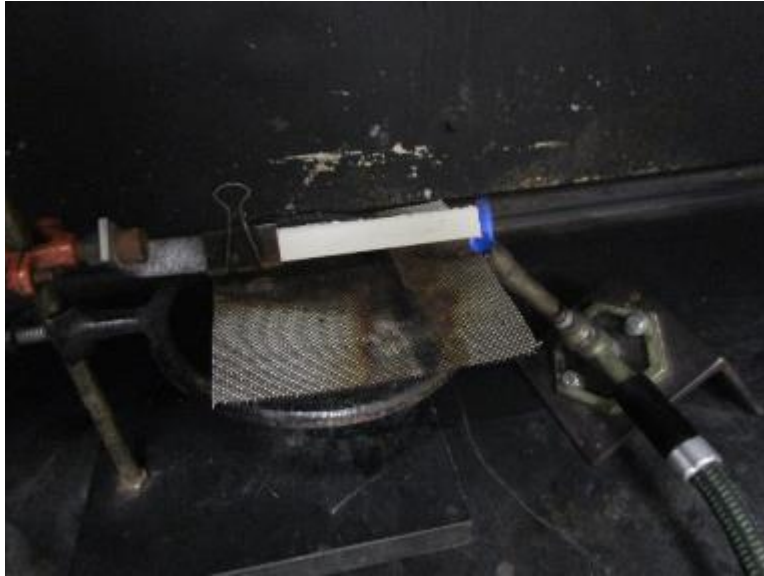
Photo No. 3 ASTM D635 Rate of Burn, Testing
