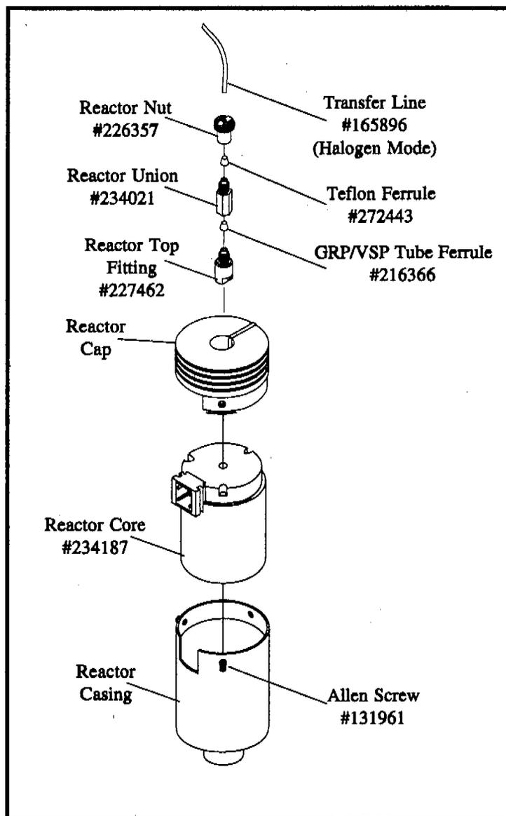
Figure 5.1. Reactor Assembly
