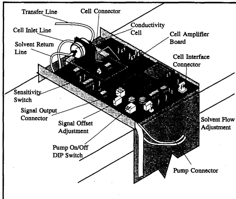
Figure 2.3. Cell/Solvent Assembly - Top View
