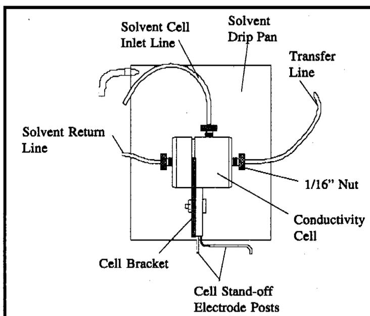
Figure 5.4. Conductivity Cell Assembly
