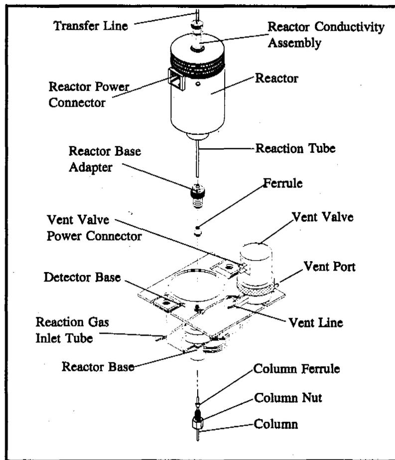
Figure 2.5. Reactor Assembly
