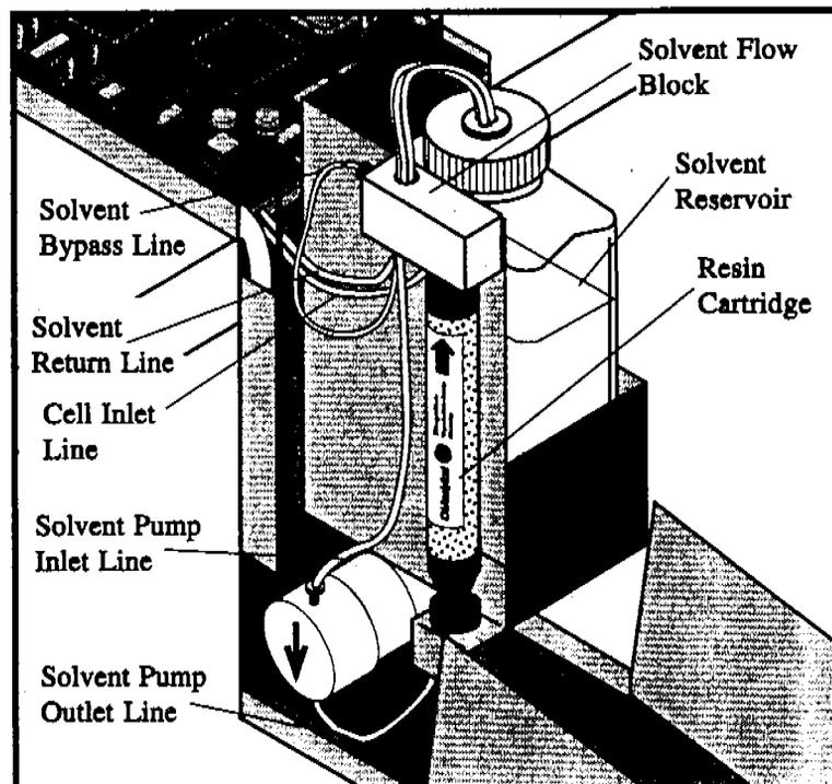
Figure 2.4. Cell/Solvent Assembly - Side View
