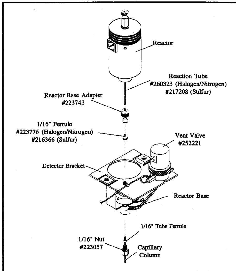
Figure 5.3. Reactor Base Assembly
