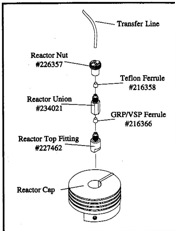
Figure 3.2. Reactor Conductivity Assembly
