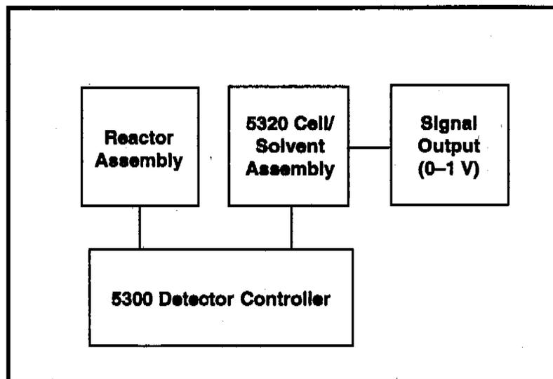
Figure 1.1. Model 5320 ELCD Principal Components
