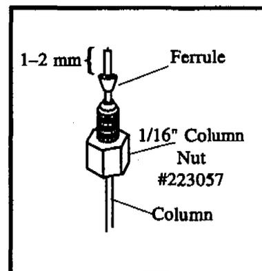
Figure 3.3. Capillary Column
