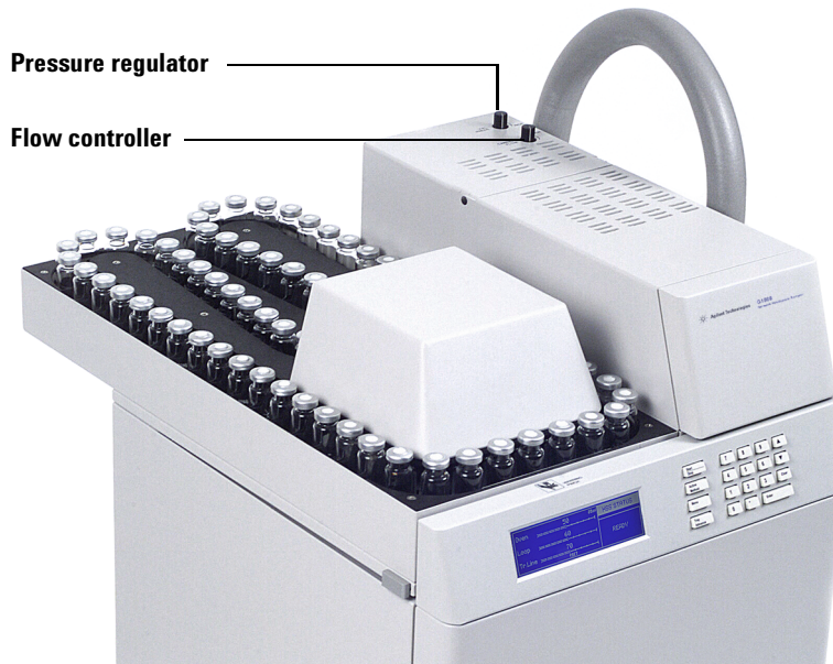
Figure 17 Location of flow controller and pressure regulator
