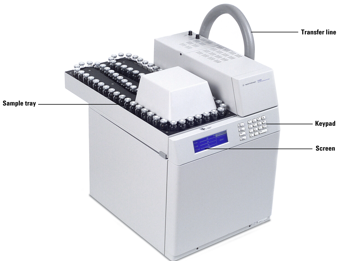
Figure 1 Overview of the G1888 Network Headspace Sampler (from the front of the instrument)
