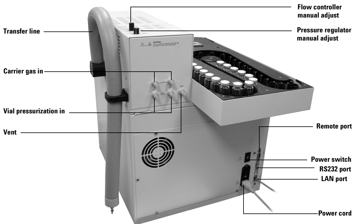
Figure 2 Overview of the G1888 Network Headspace Sampler (from the back of the instrument)
