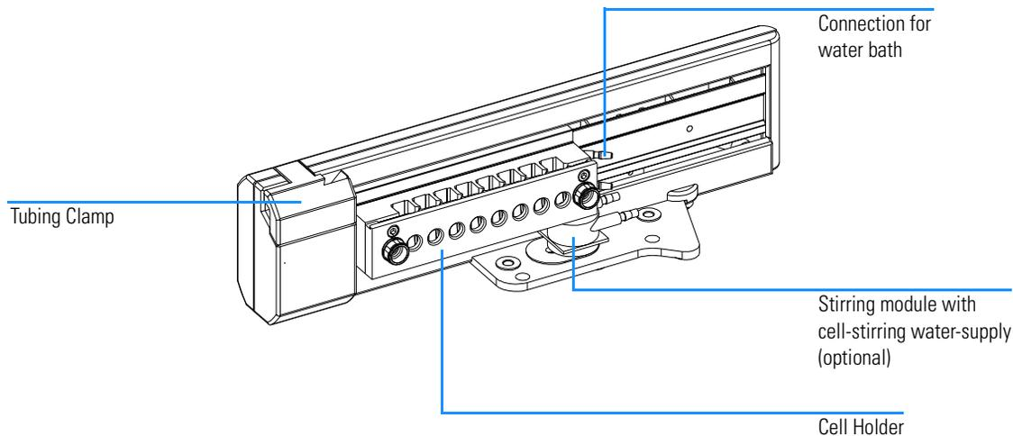
The holder is attached to the multicell transport base which contains a stepper motor to move the designated cell into the optical path. A water-driven magnetic stirrer can be fitted under the holder in one of two positions—either under the cell in the optical path or under the cell to the left of the cell in the optical path.
