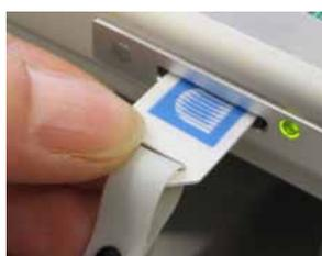
Fig. 40: Inserting a memory chip card in a memory card slot
