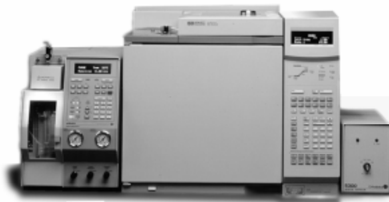
OI Analytical Purge and Trap and Detectors Combine with the HP 6890 Plus GC in the Pesticides Analysis System
