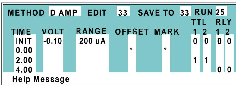
Figure C-14. Method Screen—DC Amperometry
