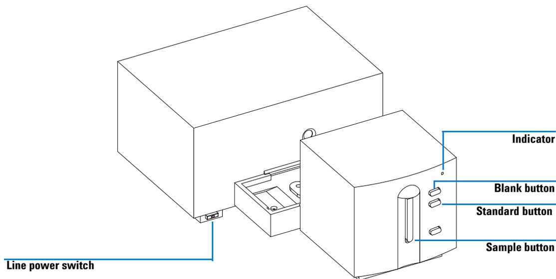
**Figure 15** Front View and Keys of the Spectrophotometer
