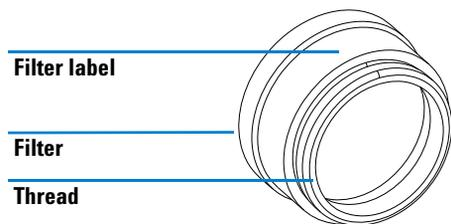
**Figure 34** Threaded Filter Ring for Multicell Transport
