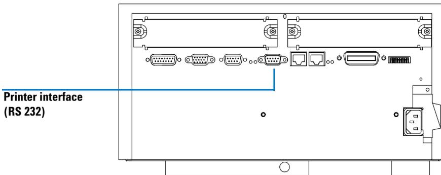
**Figure 4** Connecting the Printer Cable to the Agilent 8453 Spectrophotometer
