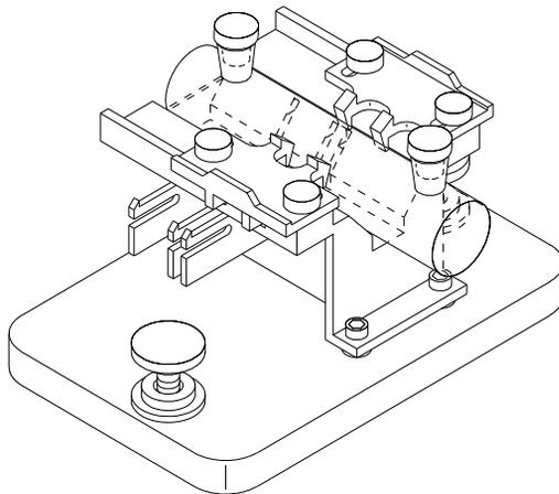
**Figure 26** Installed 10-cm Cylindrical Cell in the Long Path Cell Holder
