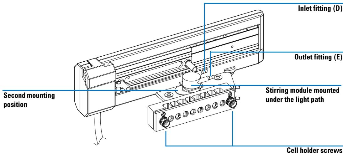
**Figure 33** Mounting the Stirring Assembly
