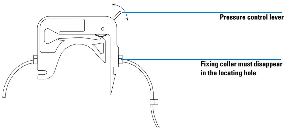
**Figure 40** Tubing Cassette with Pump Tubing
