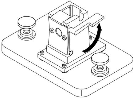
2 Insert the sample cell, making sure you orient it correctly. The frosted (non-clear) sides of the sample cell *should not* be in the path of the light beam.
