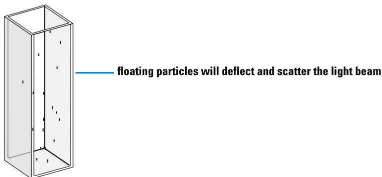
**Figure 10** Floating Particles in a Cell
