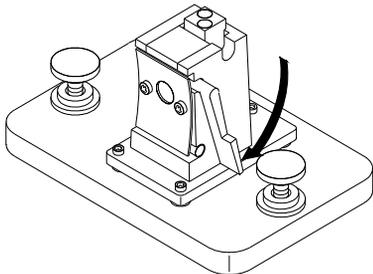
Small volume flow cells and particularly any cells with less than a 2 mm aperture may require use of the optional adjustable cell holder. The adjustable cell holder helps you ensure the cells are properly centered in the light path.
