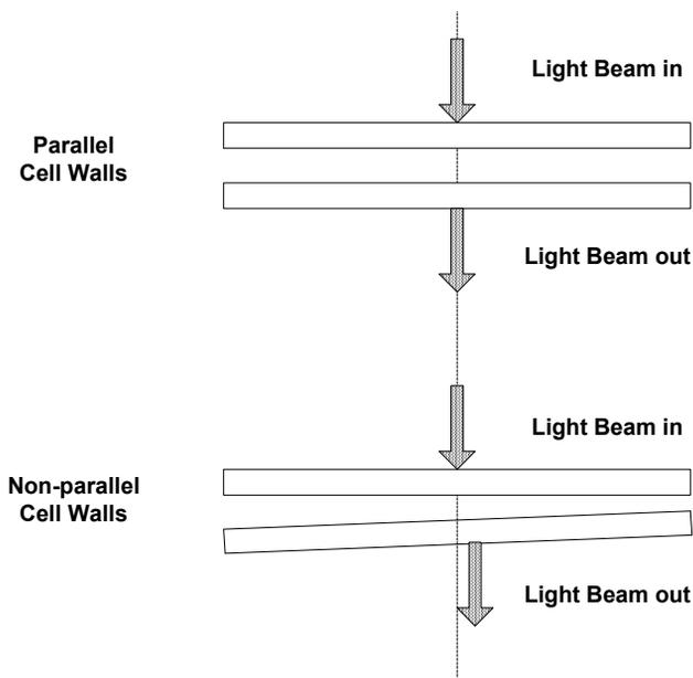
**Figure 7** Shift of the Instrument Light Beam due to non Parallel Cell Walls
