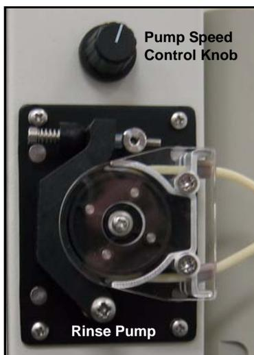
*Figure 3-2. Rinse Pump Speed Control Knob*
