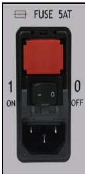
The power entry incorporates the AS-HV main power switch and the fuse compartment.
