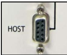
The **HOST** port provides a connection from the AS-HV to a serial port on the Chromeleon PC. The AS-HV Ship Kit (P/N 064051) includes an RS-232 cable (P/N 060683) for this connection.
