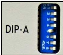
The DIP switches are numbered 1 to 8 (from top to bottom). SW5 sets the baud rate (the only communication parameter that can be set on the AS-HV).
