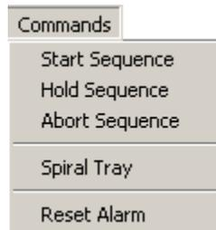
Consists of four functions that control the Model 1010’s analytical progression. These functions also can be performed by clicking on the **Start**, **Hold**, **Abort** and **Spiral Tray** buttons on the Status screen.
