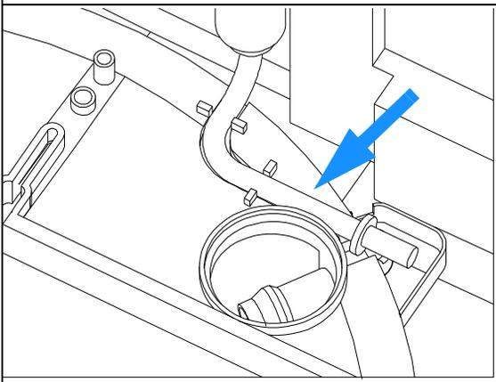
**14** Replace the heat exchanger assemblies, see “Installing the Heat Exchanger Assemblies” on page 90.
