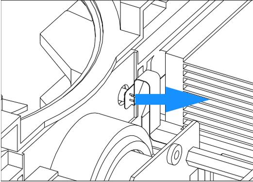
**7** Pull the top plastic panel together with the Z-panel completely out of the guide.
