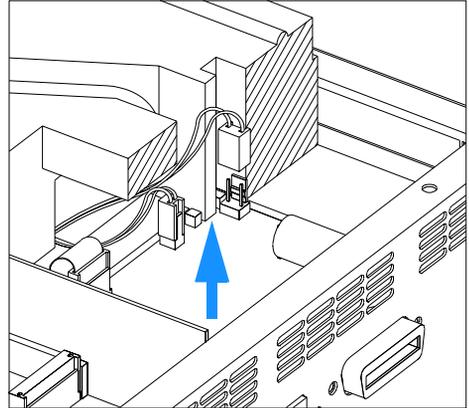
**5** Place the top plate on the foam and slide it towards the rear and fix the screws at the rear of the top plate.
