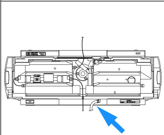
**7** Route tubings from modules above through the openings in the funnel holder (top) and the plastic bottom part. Remove small plastic plugs first.
