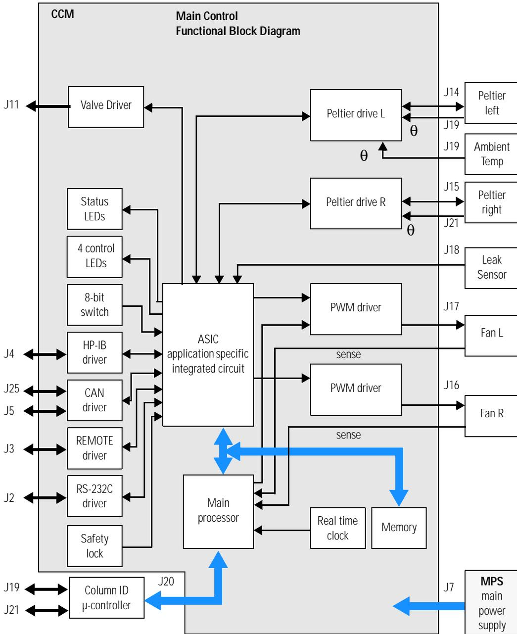
**Figure 29 Interconnection Diagram Column Compartment Main Board**
