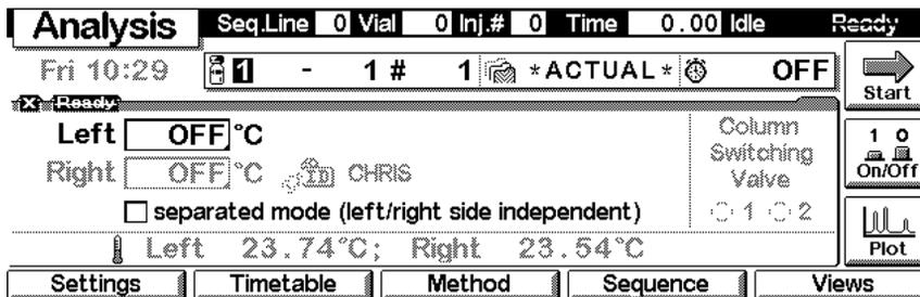
The **m**-key allows access to the context sensitive menu. **Setup view** leads you to add sections for additional HP 1100 modules. **Restart** re-boots the control module.
