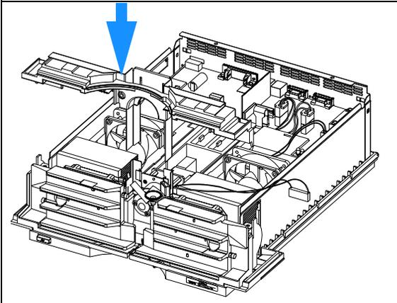
**4** Carefully plug the ambient temperature sensor into the rear of the top plastic panel.
