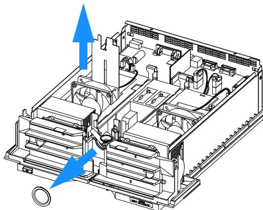
Repairing the Column Compartment
