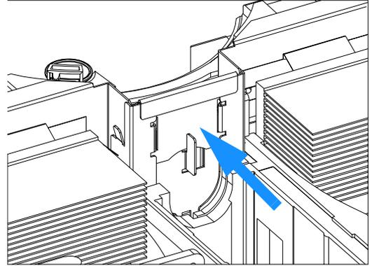
**4** Lift the Z-panel together with the top plastic panel half-way out of the guide.
