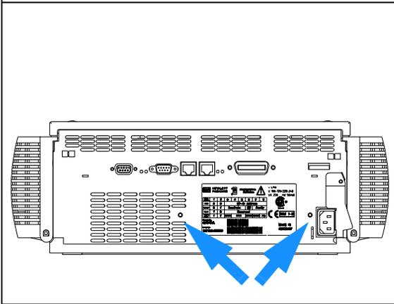
**20** Press down and clip in the power switch light pipe into the power supply.
