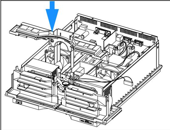
**4** Carefully plug the temperature sensor into the rear of the top plastic panel.
