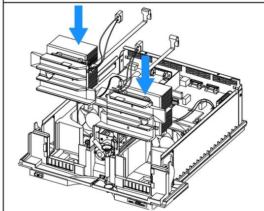
Repairing the Column Compartment
