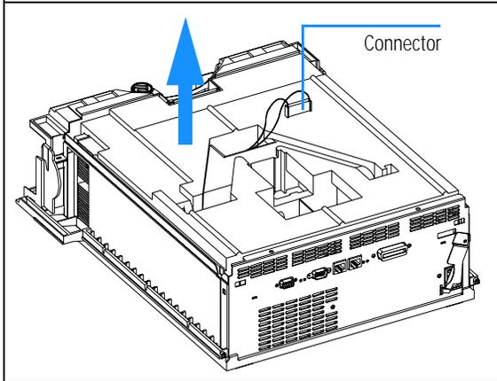
**Do not connect a power plug to the column compartment after removing the top covers.**
