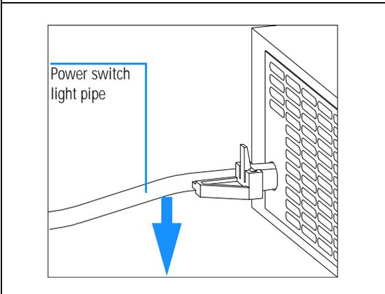
**18** Remove the power supply completely.
