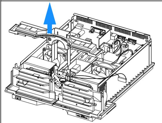
**9** Remove the heat exchanger assembly.
