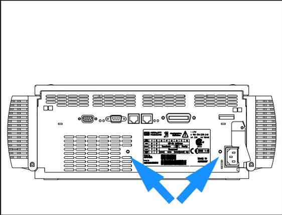
**17** Press down the power switch light pipe to remove it from the coupler.
