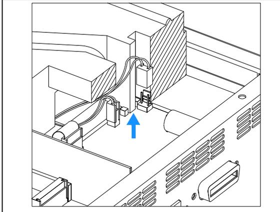
**8** Position of safety light switch on the main board when removing the foam.
