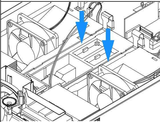
**10** Replace the foam section, the top cover and front cover, see “Installing the Foam and the Top Cover” on page 102.
