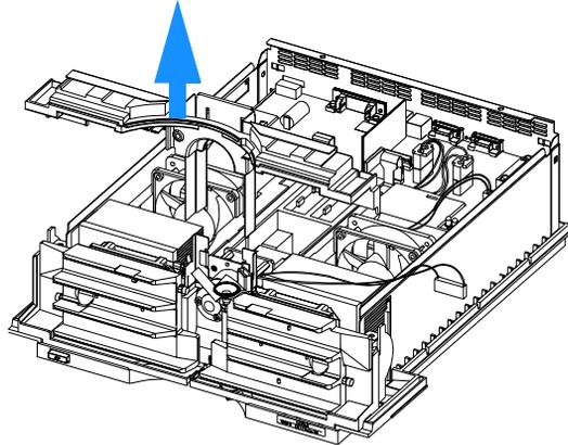
**8** Remove the Valve from its location.
