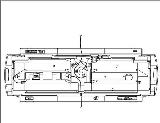
**2** Loosen each fixing stator screws two turns at a time. Remove bolts from head.
