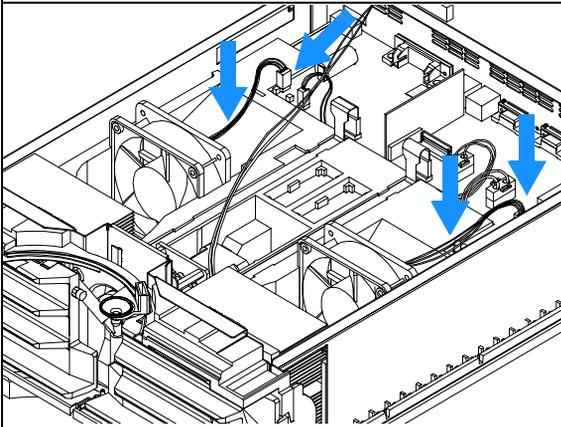
**5** Replace the foam section, the top cover and front cover, see “Installing the Foam and the Top Cover” on page 102.
