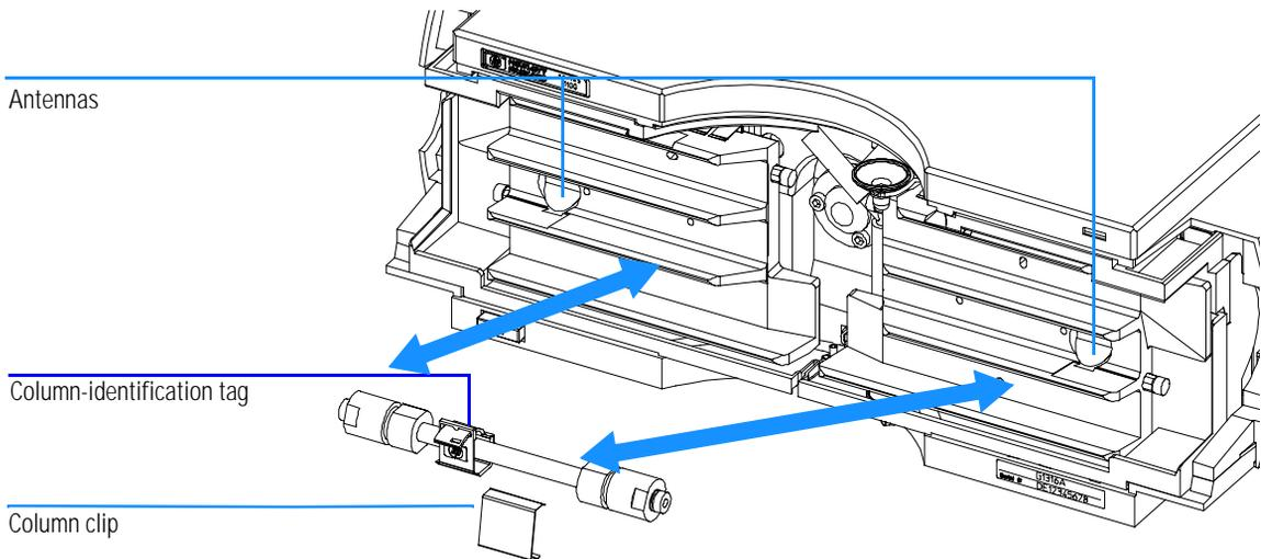
When correctly placed on the heat exchanger, the distance between tag and antenna is 1–2 mm. This is the optimum distance for proper function. The identification tag can be easily removed from the column.
