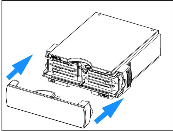
**9** Replace the column compartment into the stack.
