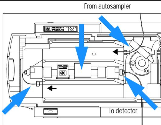
**4** Or place the column on the right heat exchanger assembly and connect the capillaries to the column.
