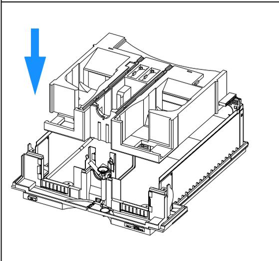
**22** Reinstall the processor board, see “Exchanging the Column Compartment Main (CCM) Board” on page 80.
