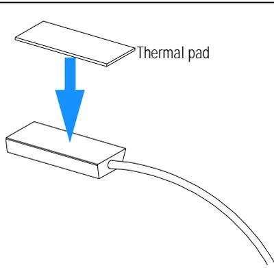
**2** Insert the temperature sensor into the spring. Ensure the face of the thermal pad faces downwards.
