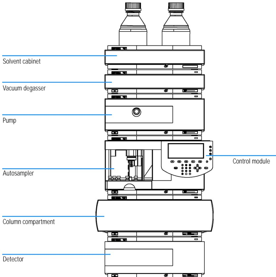
Installing the Column Compartment
