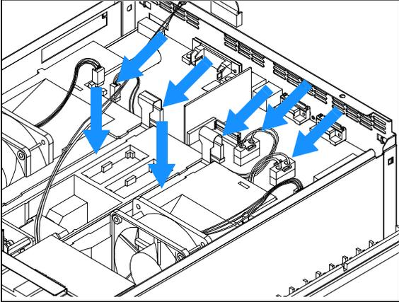
**16** Replace the foam section, the top cover and front cover, see “Installing the Foam and the Top Cover” on page 102.
