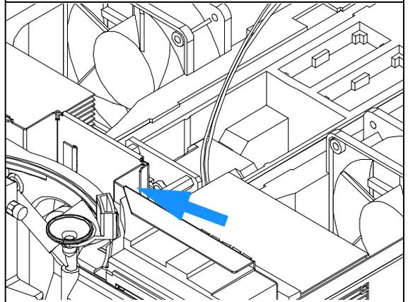
**9** Replace the foam section, the top cover and front cover, see “Installing the Foam and the Top Cover” on page 102.
