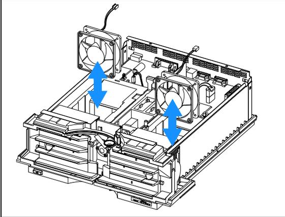
**3** The arrow on the fan should correspond with the direction of air flow which is from the front to the rear of the column compartment.
