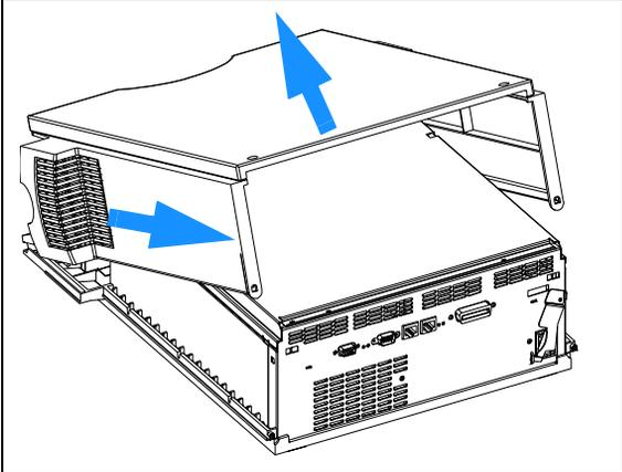
**5** Unscrew the screws at the rear of the top plate, slide the plate towards the front and remove it.
