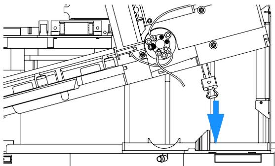
**4** Place the sampling unit and tray base into the autosampler.
