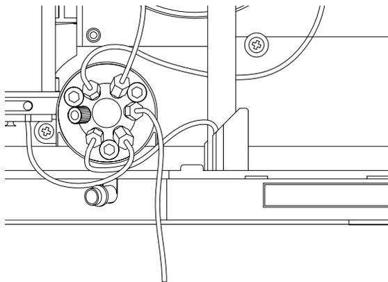
Slide the waste tube into the waste holder in the leak tray.
