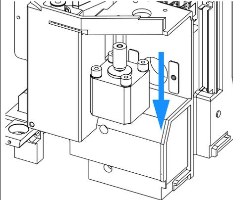
**5** Feed the motor cable through to the SUD board. Connect the cable to the connector, labelled “Needle M”.
