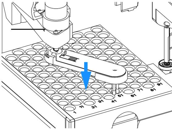
**6** Replace the gripper arm by holding the paper clip in place, pushing the gripper arm into the holder and rotating the gripper arm to the left.
