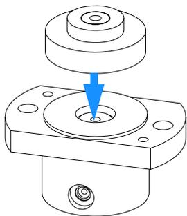
**8** Reassemble the metering head assembly. Carefully insert the plunger into the base. The closed side of the metering head must be on the same side as the lower one of the two capillary drillings.
