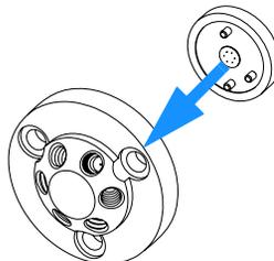
**5** Install stator head and stator face. Tighten the bolts alternately two turns at a time until the stator head is secure.
