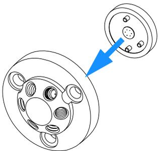
**8** Install stator head and stator face. Tighten the bolts alternately two turns at a time until the stator head is secure.
