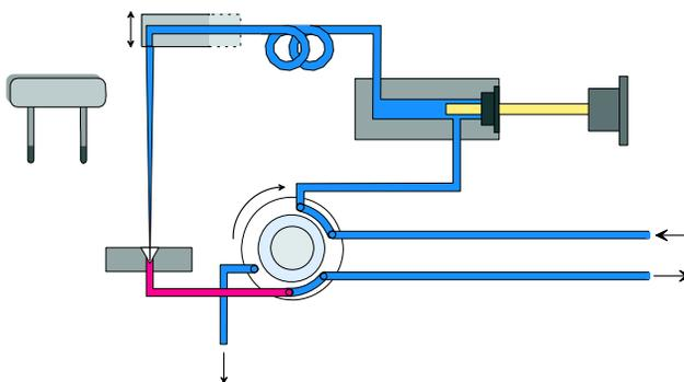
**Figure 32** Mainpass Position (Sample Injection)
