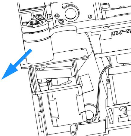
**4** Feed the cable of the new valve through to the SUD board).
