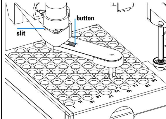
2 Rotate the arm approximately 2.5cm (1 inch) to the left and insert the straightened paper clip into the slit.
