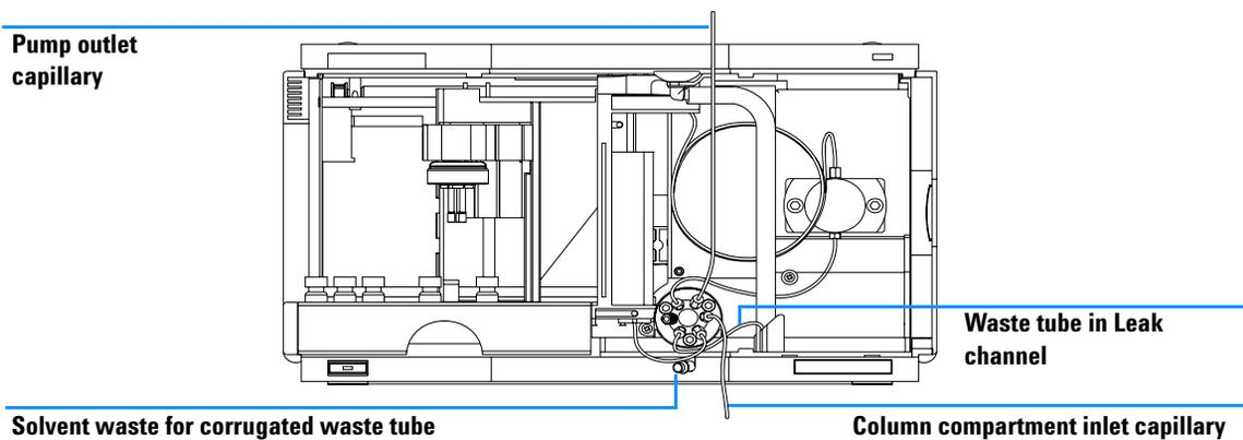
**Figure 10** Hydraulic Connections
