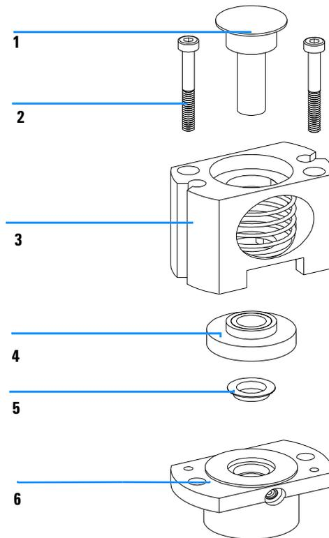
**Figure 20** Analytical-Head Assembly
