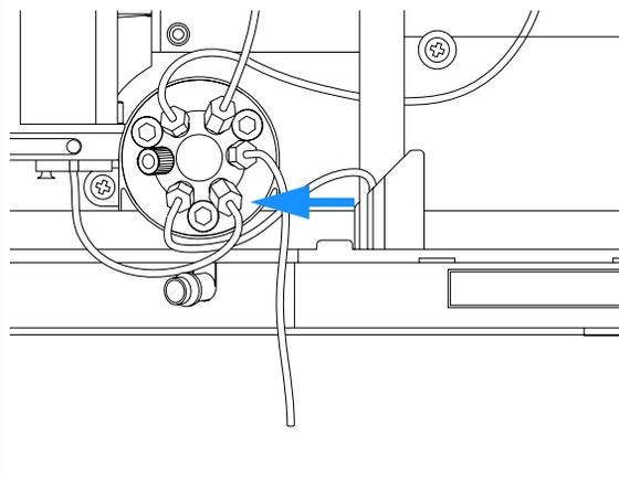
**5** Use "Down" to position the needle approximately 2 mm above the seat
