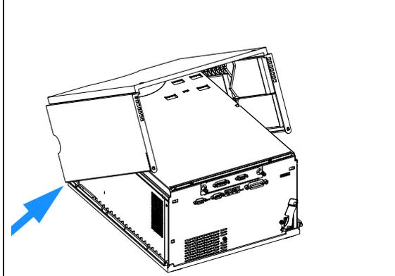
**5** Lower the cover into place. Ensure the clips close firmly.
