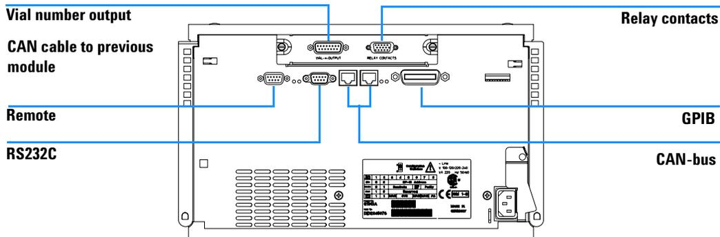
**Figure 6** Cable Connections
