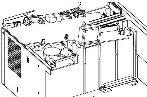
**4** Install new board. Ensure ribbon cables are positioned in the slot in the board.
