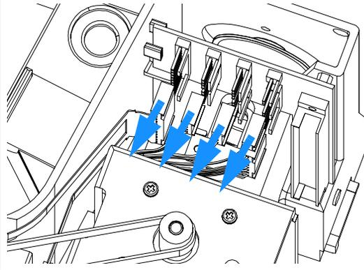
**2** Remove the two fixing screws, and lift out the board.
