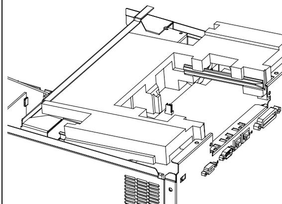
2 Engage the slot on the top plate onto the side plate.
