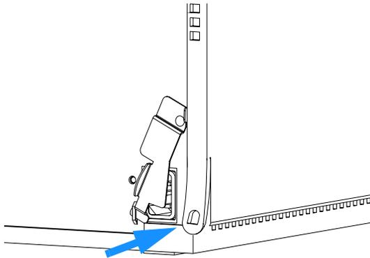
**6** Slide the power lock to the right, and install the power cable.
