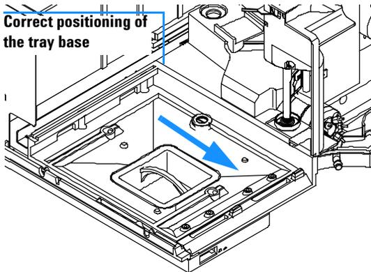
2 Tighten the locking screw ¼-turn clockwise.
