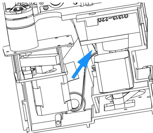
**5** Connect the valve cable to the connector (labelled "Valve Assy").
