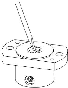
**6** Install the new seal. Press the seal firmly into position.
