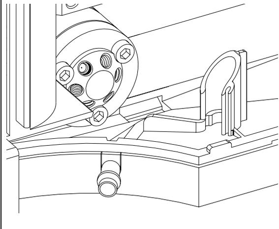
2 Loosen each fixing bolt two turns at a time. Remove the bolts from the head.
