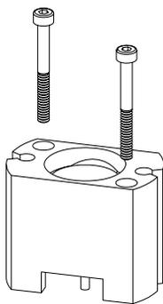
**10** Install the metering head assembly in the autosampler. Ensure the large hole in the metering head is facing downwards.
