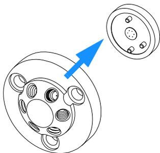
**4** Place the stator face in place on the stator head. Ensure the pins on the stator engage in the holes in the stator head.
