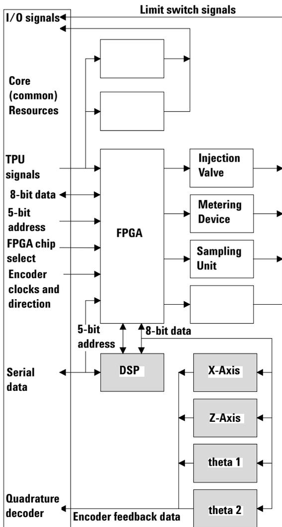
Figure 38 Autosampler block diagram
