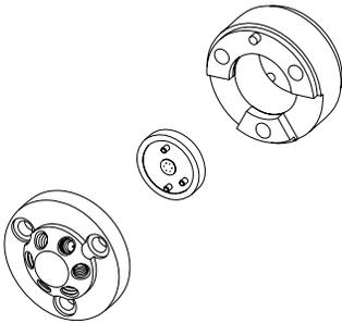
**4** Remove the rotor seal and isolation seal.
