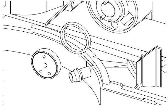
**5** Install the new rotor seal and isolation seal. Ensure the metal spring inside the isolation seal faces towards the valve body.
