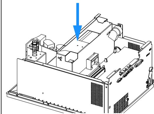
2 Ensure the slot on the top of the transport assembly engages with the stud on the sampling unit.
