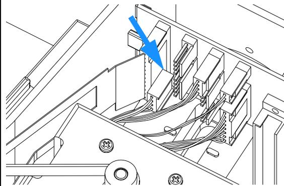
**2** Remove the four fixing screws.
