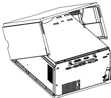
**5** Unscrew the three screws on the top plate. Remove the top plate.
