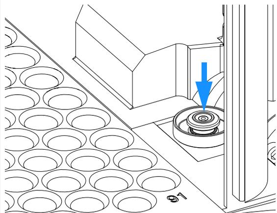
**4** Connect the seat-capillary fitting to port 5 of the injection valve.
