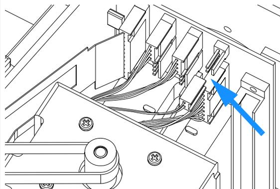
**2** Feed the cable of the new sensor through the base of the sampling unit to the SUD board.
