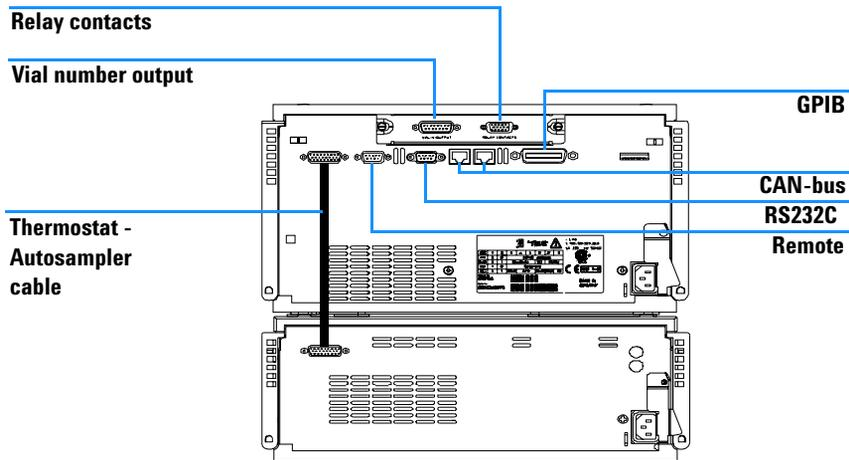
**Figure 9** Cable Connections
