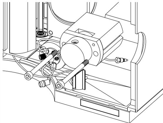
**11 Reinstall the capillaries.**
