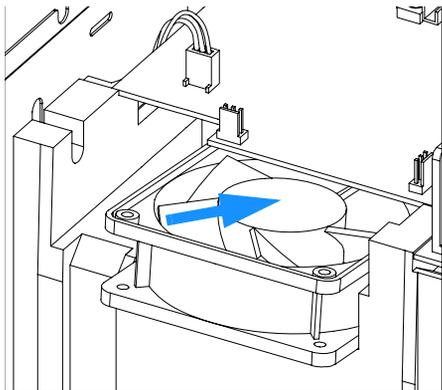
**4** Connect the fan connector to the ASM board.
