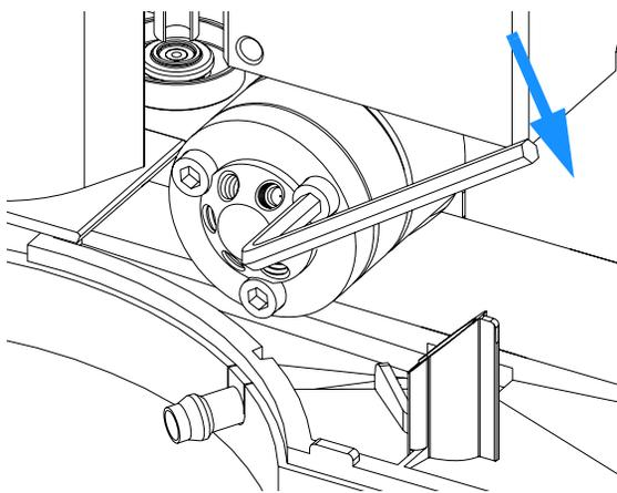
**6** Reconnect the pump capillaries to the valve ports (see [“Hydraulic Connections”](#) on page 35).
