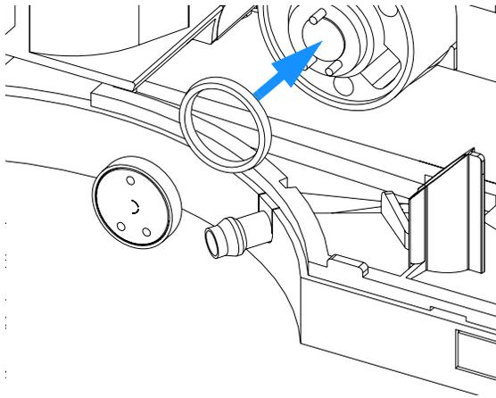
**6** Install the stator ring with the short of the two pins facing towards you at the 12 O'Clock position. Ensure the ring sits flat on the valve body.
