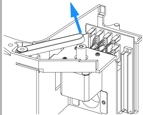
2 Disconnect the motor connector from the SUD board (labelled "Needle M").
