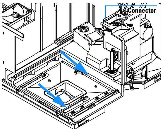
**6** Install the pump and column thermostat capillaries (ports 1 and 6) in the injection valve.
