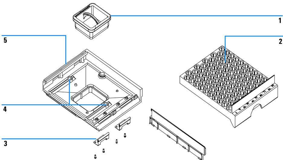
**Figure 27** Thermostatted Autosampler Vial Trays and Tray Base
