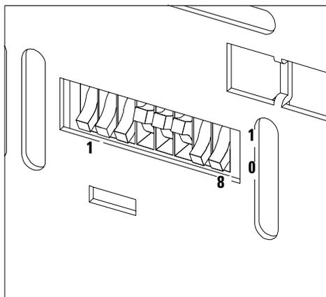
**Figure 42** 8-bit Configuration Switch
