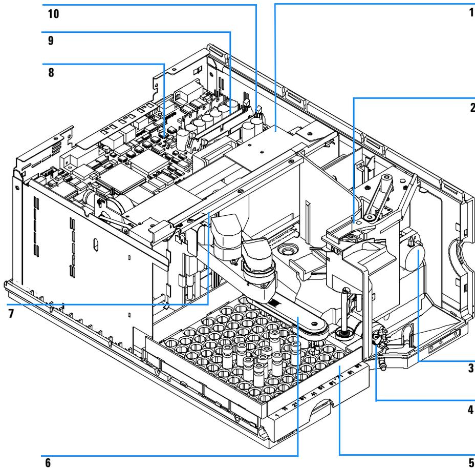
**Figure 18** Autosampler Main Assemblies
