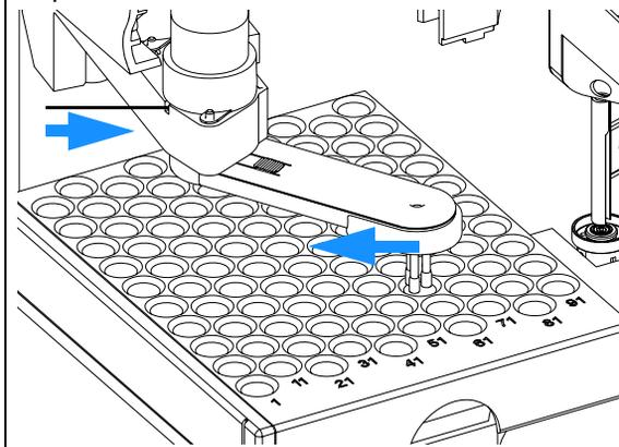
**3** Rotate the gripper arm slowly from left to right and apply a gentle pressure to the paper clip. The clip will engage on an internal catch and the rotation of the arm will be blocked.
