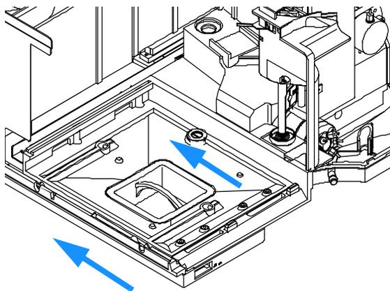
**4** Lift the sampling unit and tray base approximately 10 cm. Slide the leak sensor out of the leak plane.
