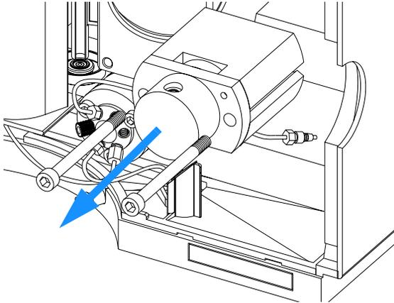
**4** Remove the four fixing screws, and remove the motor.
