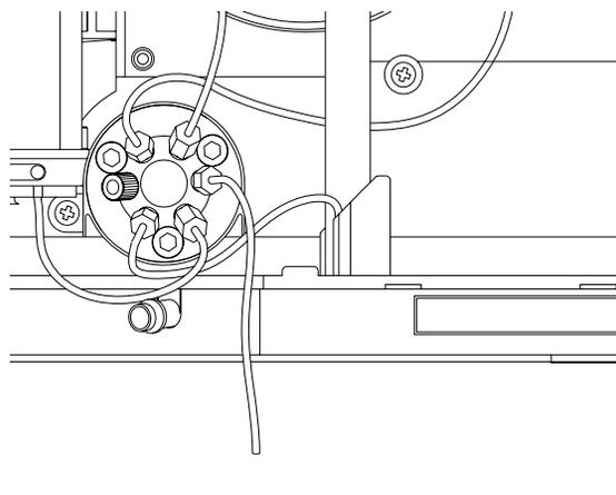
7 Slide the waste tube into the waste holder in the leak tray.
