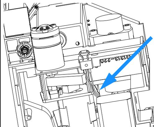
**3** Connect the connector to the connector (labelled “leak sensor”).
