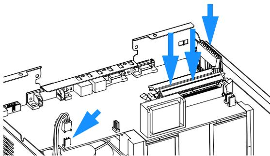
**6** Replace GPIB and RS232 connector screws.
