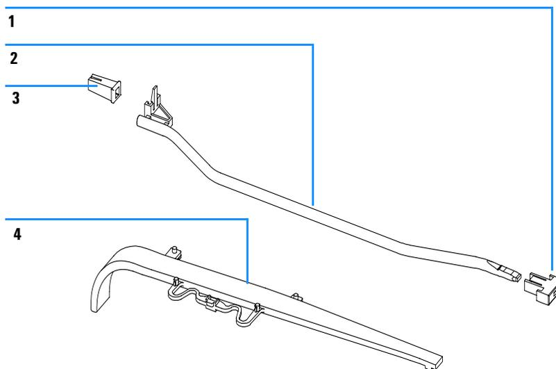
**Figure 25** Power and Status Light Pipes
