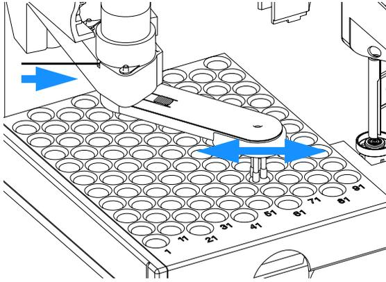
**4** Hold the paper clip in place, press the gripper release button and rotate the gripper arm to the right.
