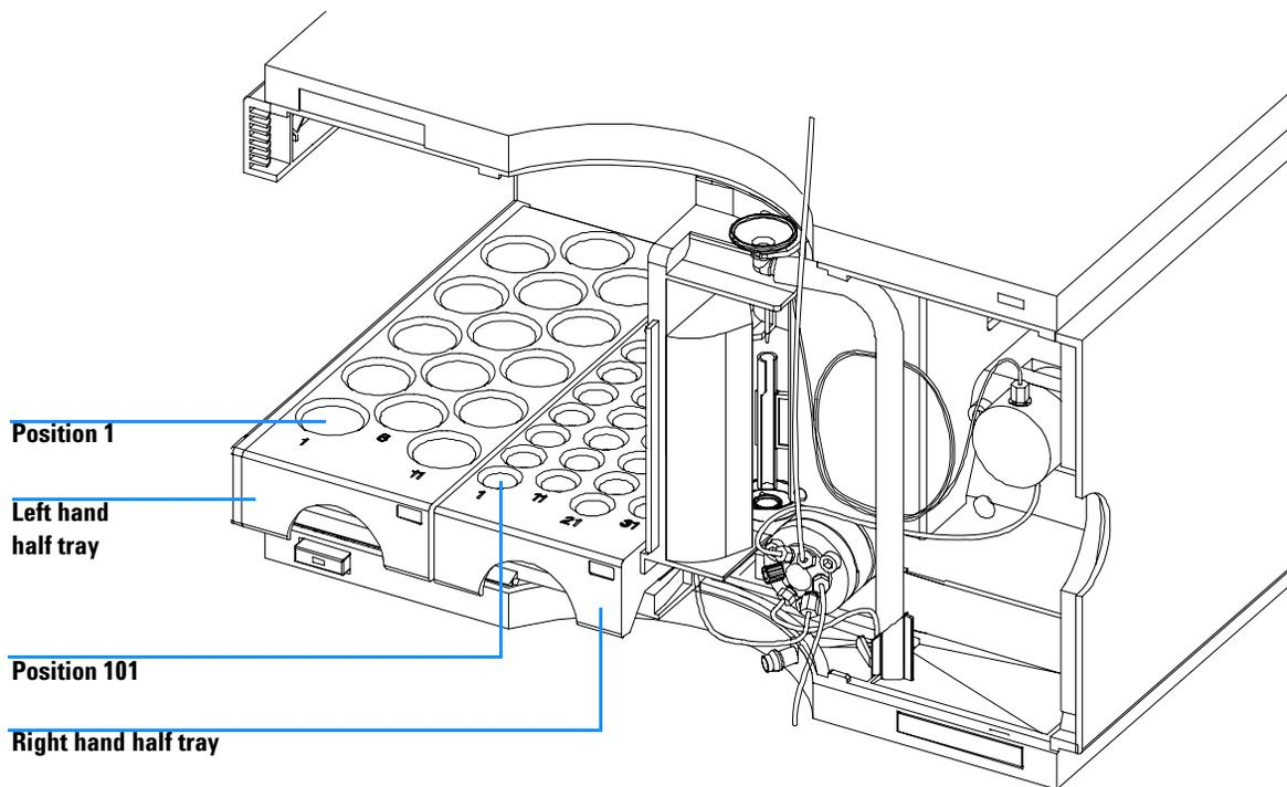
**Figure 12** Numbering of Tray Positions
