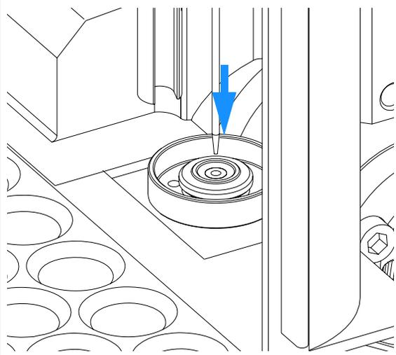
**6** Ensure the needle is aligned with the seat. If required, bend the needle slightly until the needle is aligned correctly.
