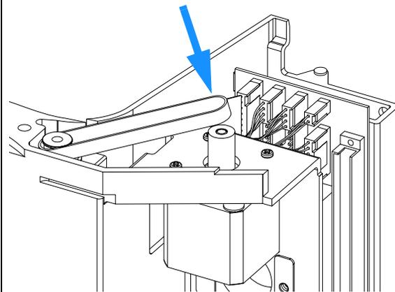
8 Install the metering-head assembly (see “Gripper Arm” on page 74).
