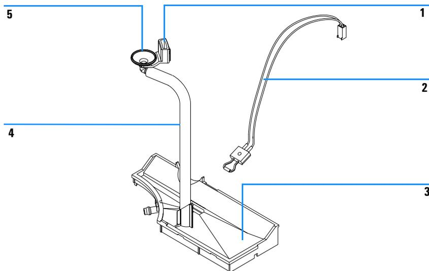
**Figure 26** Leak System Parts
