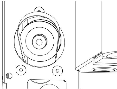
**6** Feed the motor cable through to the SUD board. Connect the cable to (labelled "Metering M").
