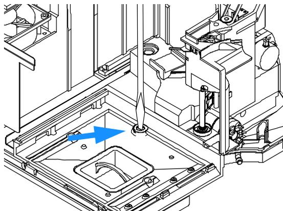
7 Slide the tray base back to disengage the tray base from the sampling unit.
