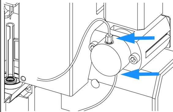
**2** Remove the two fixing bolts, and pull the head assembly away from the sampler. Notice that the closed side of the metering head faces upwards.
