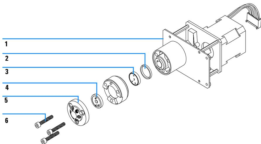
**Figure 21** Injection-Valve Assembly
