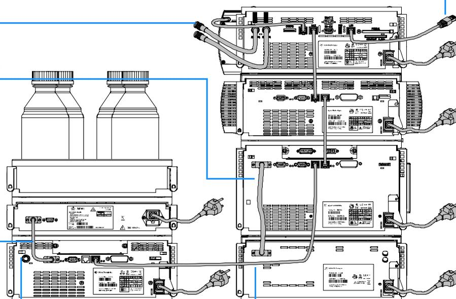
**Figure 4** Recommended Stack Configuration for a thermostatted ALS (Rear View)
