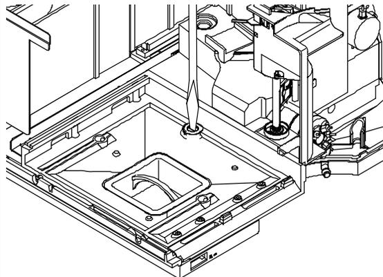
**3** While holding the sampling unit and tray base, slide the leak sensor into the holder in the leak plane.
