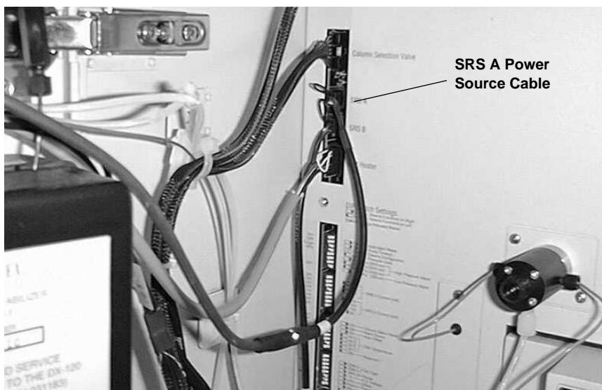
*Figure 104. The DX-120 SRS A Power Source Cable*
