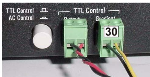
Figure 64. RFC TTL Connections
