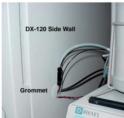
6. Connect the cable to the 2-pin connector on the DX-120 adapter cable (see Figure 65).
