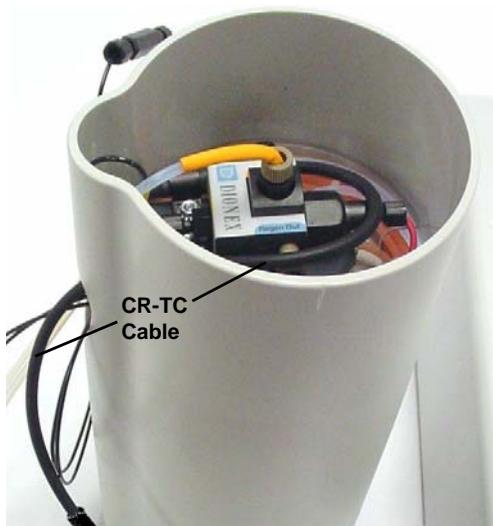
Figure 89. Installing the CR-TC
