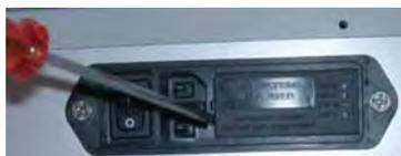
Fig. 5: Fuse cartridge
