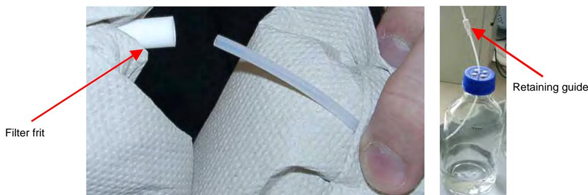
Fig. 13: Connecting the solvent lines to the reservoir
