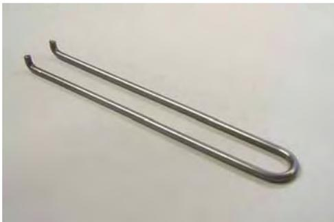
Fig. 60: Extractor for bushing with draining device
