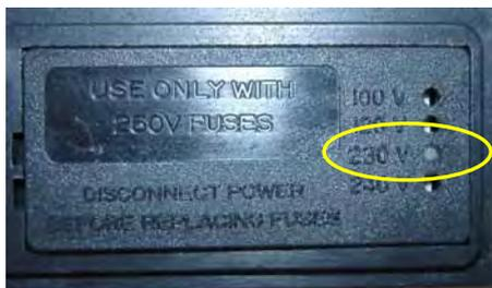
Fig. 4: Factory-set voltage selection, here: 230V
