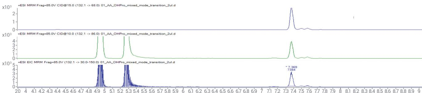
Low and high collision energy product ion and MRM scan for a mixed-mode acquisition showing isobars (leucine and isoleucine), as well as an MRM for an 'unknown' analyte (hydroxyproline).
