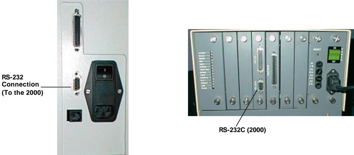
Figure 8-1: Electronic Communication Cable connection (SOLATek 72 to 2000)
