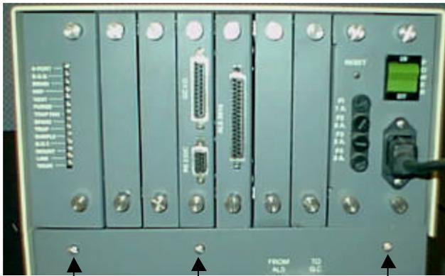
Figure 4-3: Screws that hold the top section of the 2000
