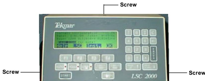
Figure 3-2: Removing the 2000 Front Panel
