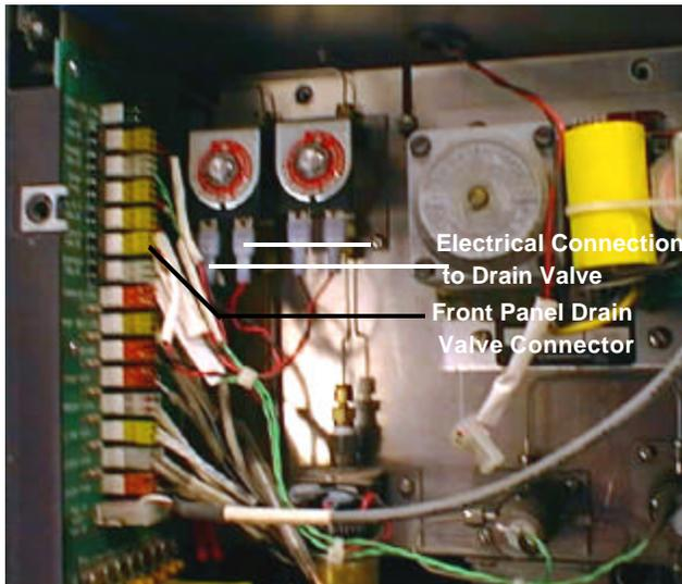
Figure 7-1: Disconnecting the Drain Valve on the 2000
