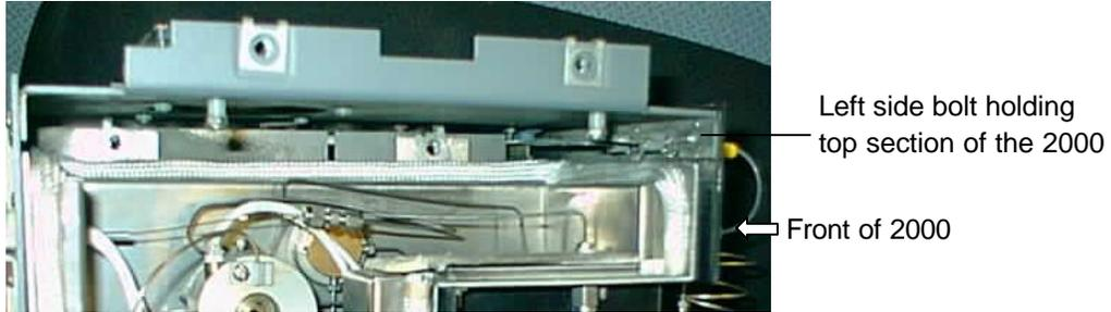
Figure 4-2: Removing the Top Section of the 2000
