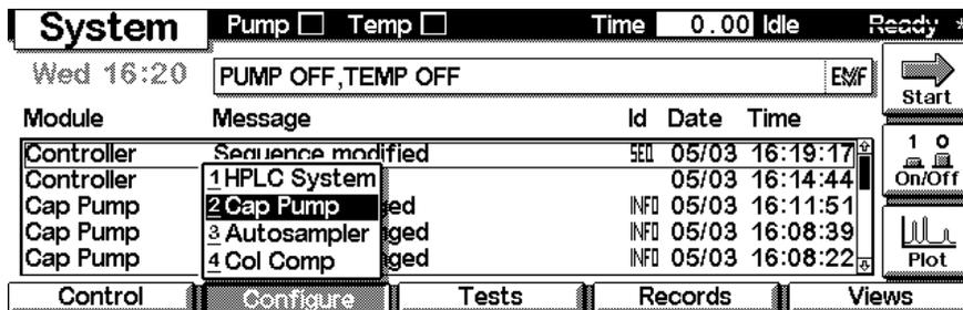
This screen gives you information about installed options and allows you to configure your pump to the filter and mixer type that is actually installed in the pump. Changes must be activated with **F6 (Done)**.
