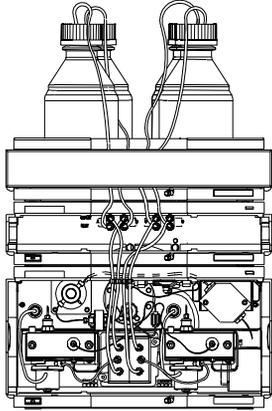
**10** Replace the front covers and reconnect the power cable to the nano pump.
