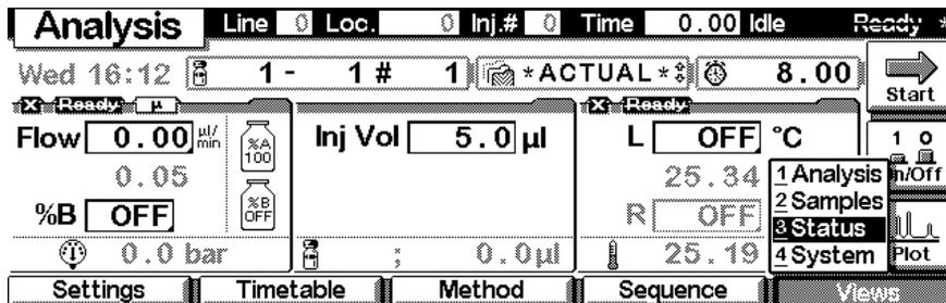
**Status** This is an example if an Agilent 1100 pump is configured standalone. Information on the actual flow rate, mobile phase composition, pressure and %-Ripple, elapsed run time and the pressure plot are shown. Press key **F8** (Start) to start a run, key **F7** (Rescale) to maximize the signal.
