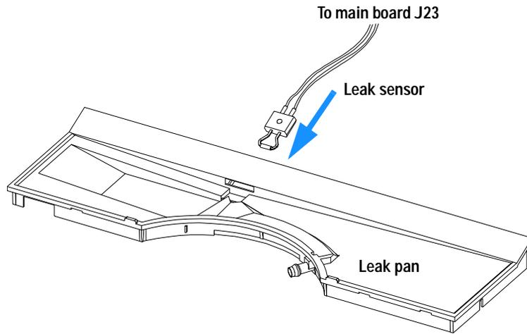
**Figure 24** Exchanging the Leak Sensor
