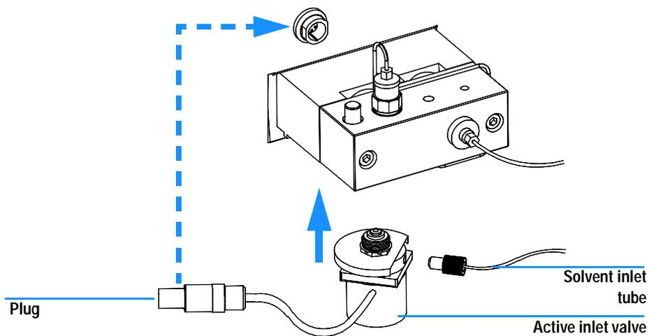
Figure 15 Exchanging the Active Inlet Valve
