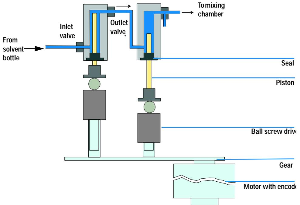
**Figure 39** Operating Principle of the pump head
