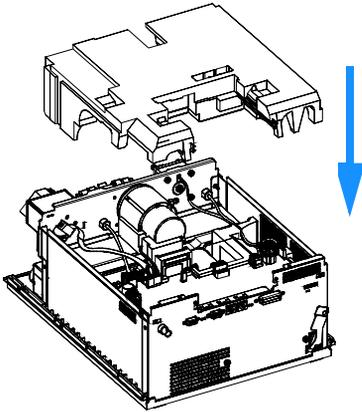
2 Make sure that the foam is installed correctly and is located in the safety light switch.
