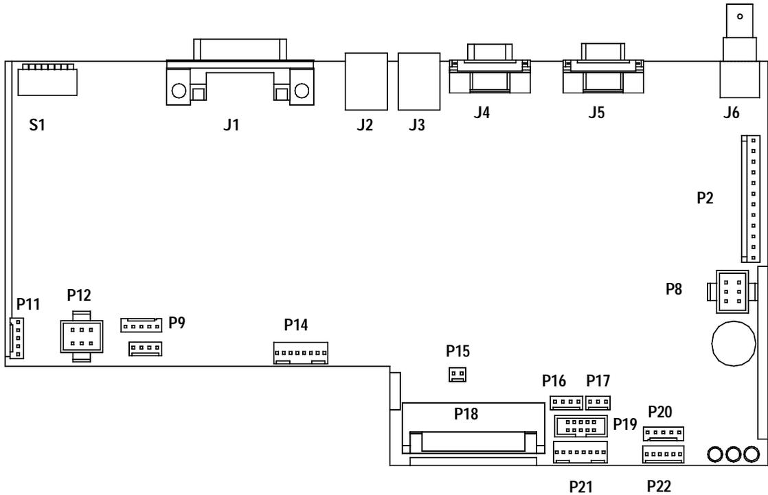
Figure 22 Board Layout of the NPM Board
