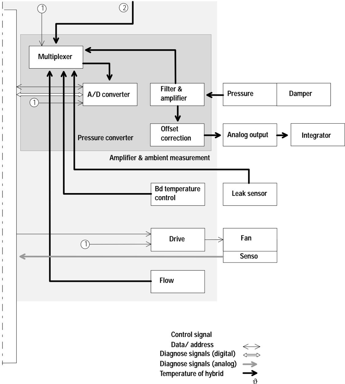
Figure 42 Block Diagram Pump Controller Board
