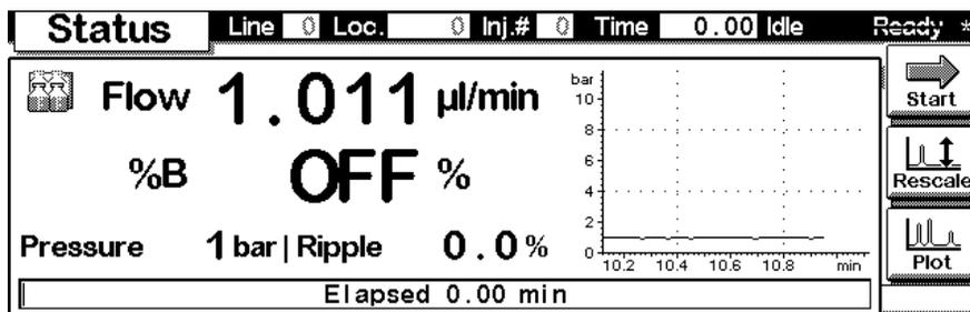
**Signal plot** Press **F6**-key (Plot) to enter the plot screen (available also from all other views). Here you can observe online signal(s). If more than one signal is configured, use the 1-2-3 numeric keys to switch between the signals.
