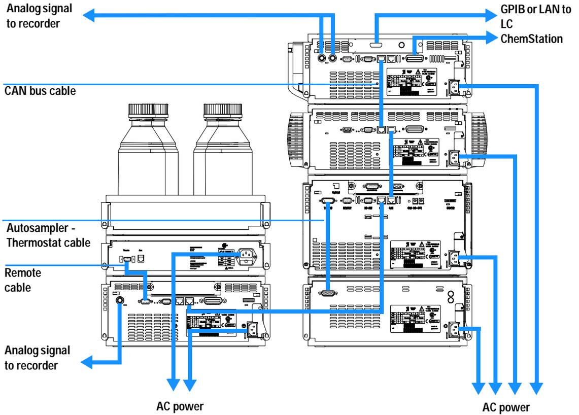
Figure 4 Recommended stack configuration (rear view)
