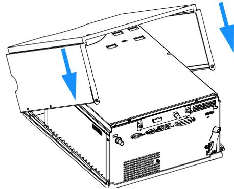
7 Ensure clips are seated correctly, move lever back.
