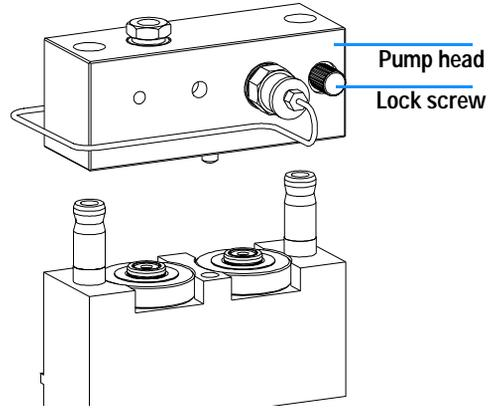
4 Remove the support rings from the plunger housing and lift the housing away from the plungers.
