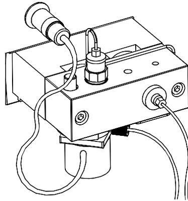
**2** Using one of the plungers carefully remove the seal from the pump head (be careful, not to break the plunger). Remove wear retainers, if still present.
