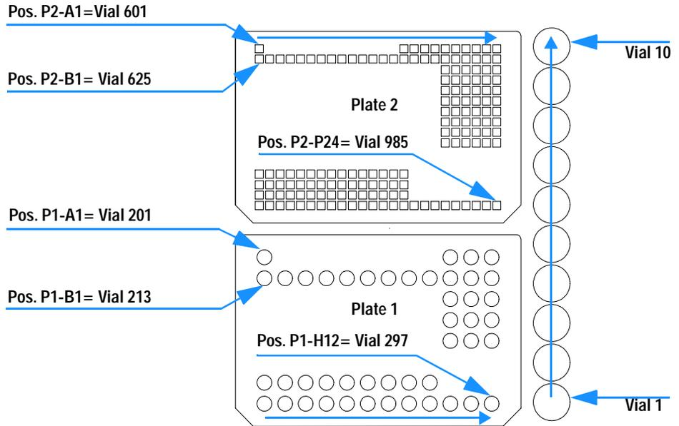
Figure 45 BCD output for the well plates
