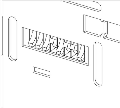
**Figure 48** 8-bit Configuration Switch
