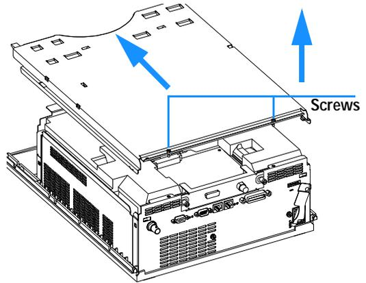
5 If an optional interface board is installed, remove it from the nano pump.
