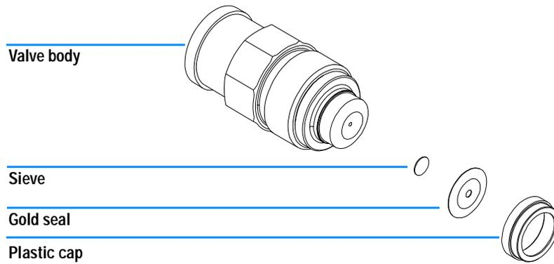
**Figure 16** Outlet Ball Valve Parts
