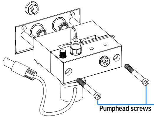
3 Place the pump head on a flat surface. Loosen the lock screw (two revolutions). While holding the lower half of the assembly, carefully pull the pump head away from the plunger housing.
