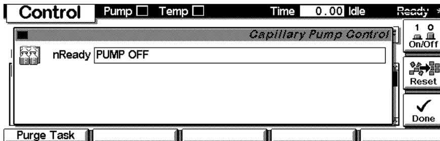
Use **F1 (Purge Task)** to access the pump's Purge Task. After selecting a channel, you can edit its **Purge Time** and **Flow Rate**. Use **F8 (Purge)** to start/stop the Purge Task as defined or define the settings for the next Purge Task. Changes must be activated with **F6 (Done)**.
