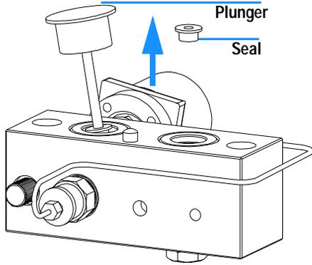
**3** Clean the pump chambers with lint free cloth. Ensure all particulate matter is removed. Best cleaning results will be achieved by removing all valves (see pages 109, 112) and the capillary. Inject solvent into each chamber.
