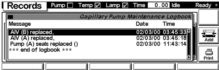
Use the **F7**-key (**Add**) to add new maintenance activities. You can add a comment to the activity into the line 'Add' using the control modules alphanumeric keys. Changes must be activated with **F6** (**Done**).
