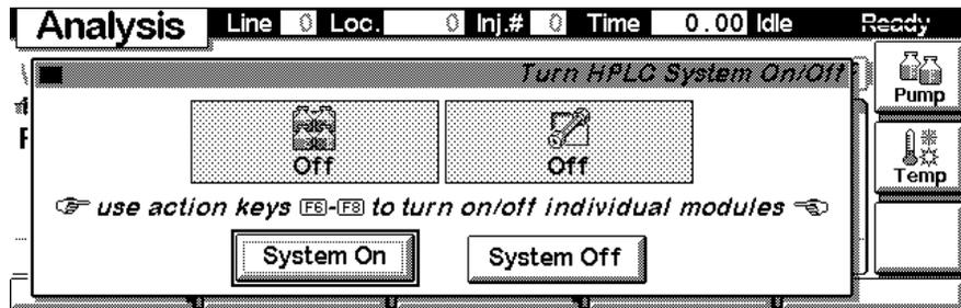
**Settings** With the F1-key (Settings) you open a pull-down menu where you can select the capillary pump module with the help of the selection or alphanumeric keys.
