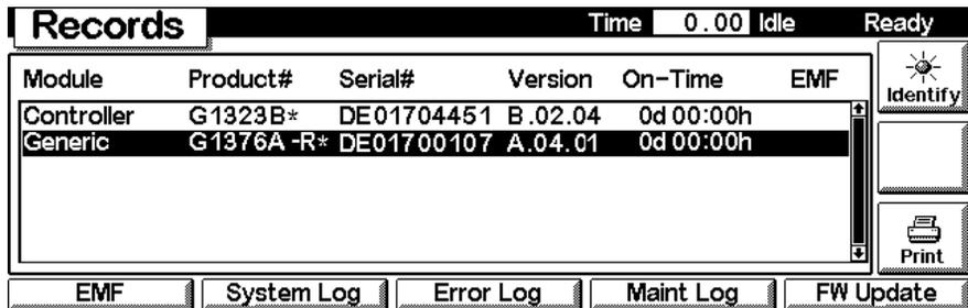
Use the **F5**-key (**FW Update**) to enter the Update section. Select the a file from the PCMCIA card (1376nnnn.DLB) and press execute. When the update has finished, press **F7**-key (**Transfer**) to return the module into the normal mode (LED on module should stay yellow).
