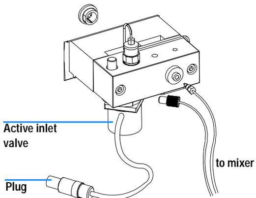
2 Using a 4-mm hexagonal key step wise loosen and remove the two pump head screws and remove the pump head from the pump drive.
