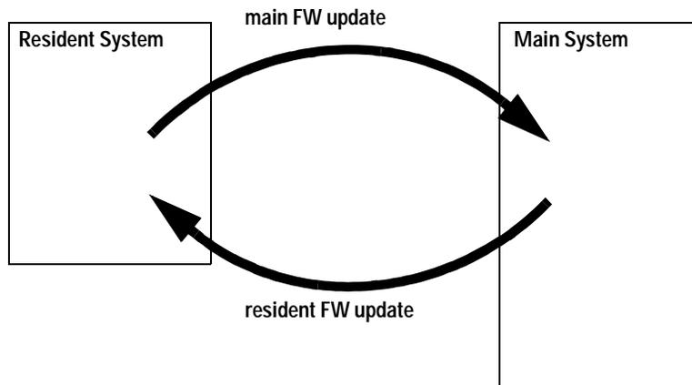
Figure 44 Firmware Update Mechanism
