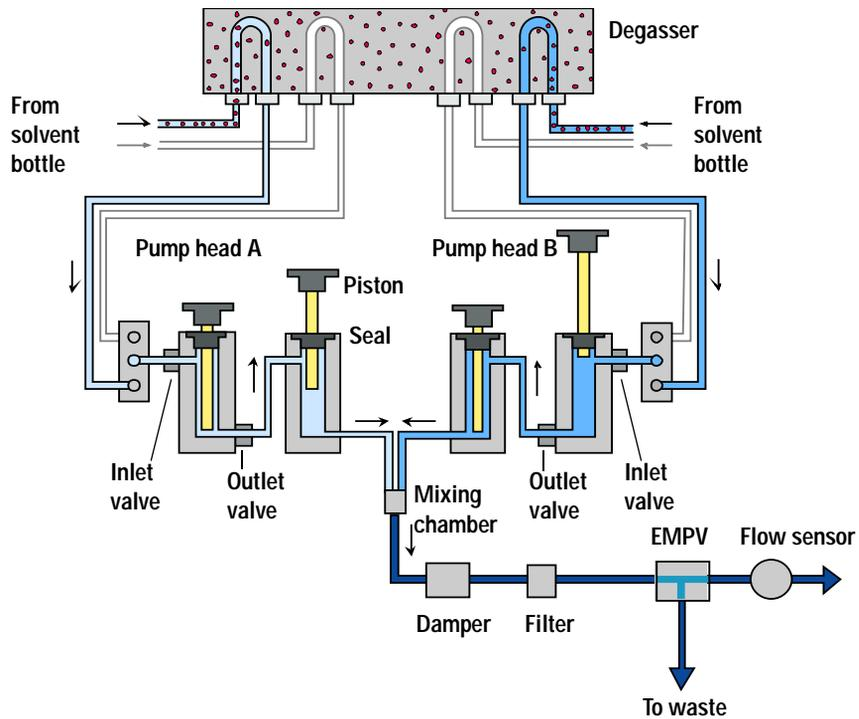
Figure 38 The Hydraulic Path
