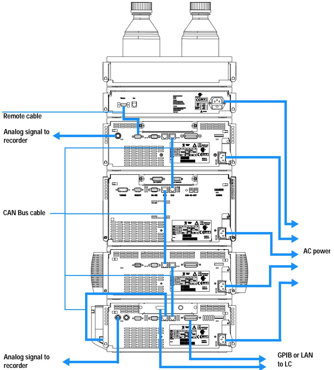
Figure 2 Recommended Stack Configuration (Rear View)
