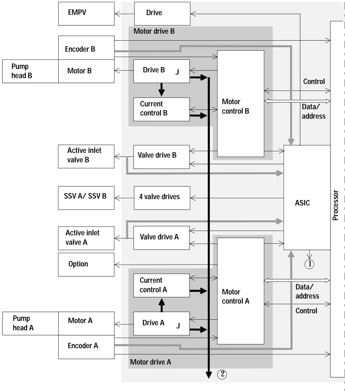
Figure 41 Block Diagram Pump Controller Board
