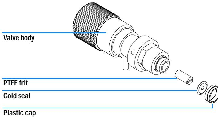
**Figure 19** Purge Valve Parts
