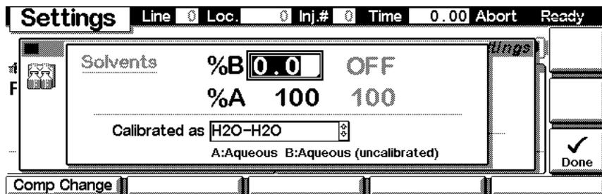
Select **Channel Selection** to choose one of the A-channels (1 or 2) and one of the B-channels (1 or 2) as the sources for solvent delivery. Changes must be activated with **F6 (Done)**.
