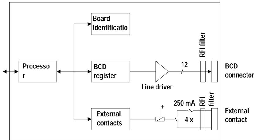
Figure 46 Block Diagram BCD Board
