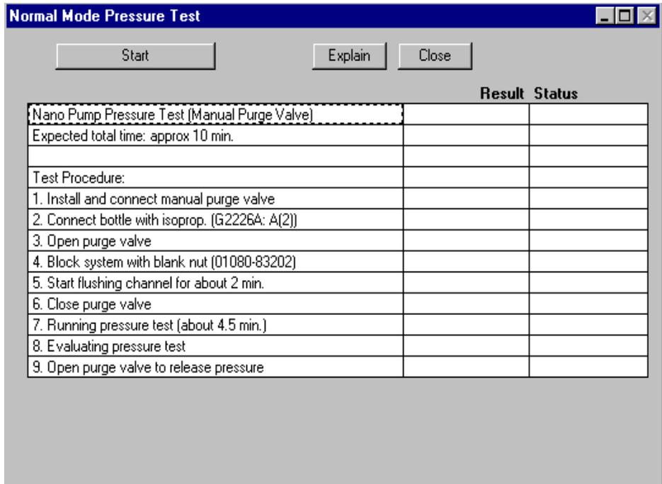
The slope and plateau is evaluated automatically. “Evaluating the Results” on page 71 describes the evaluation and interpretation of the pressure test results
