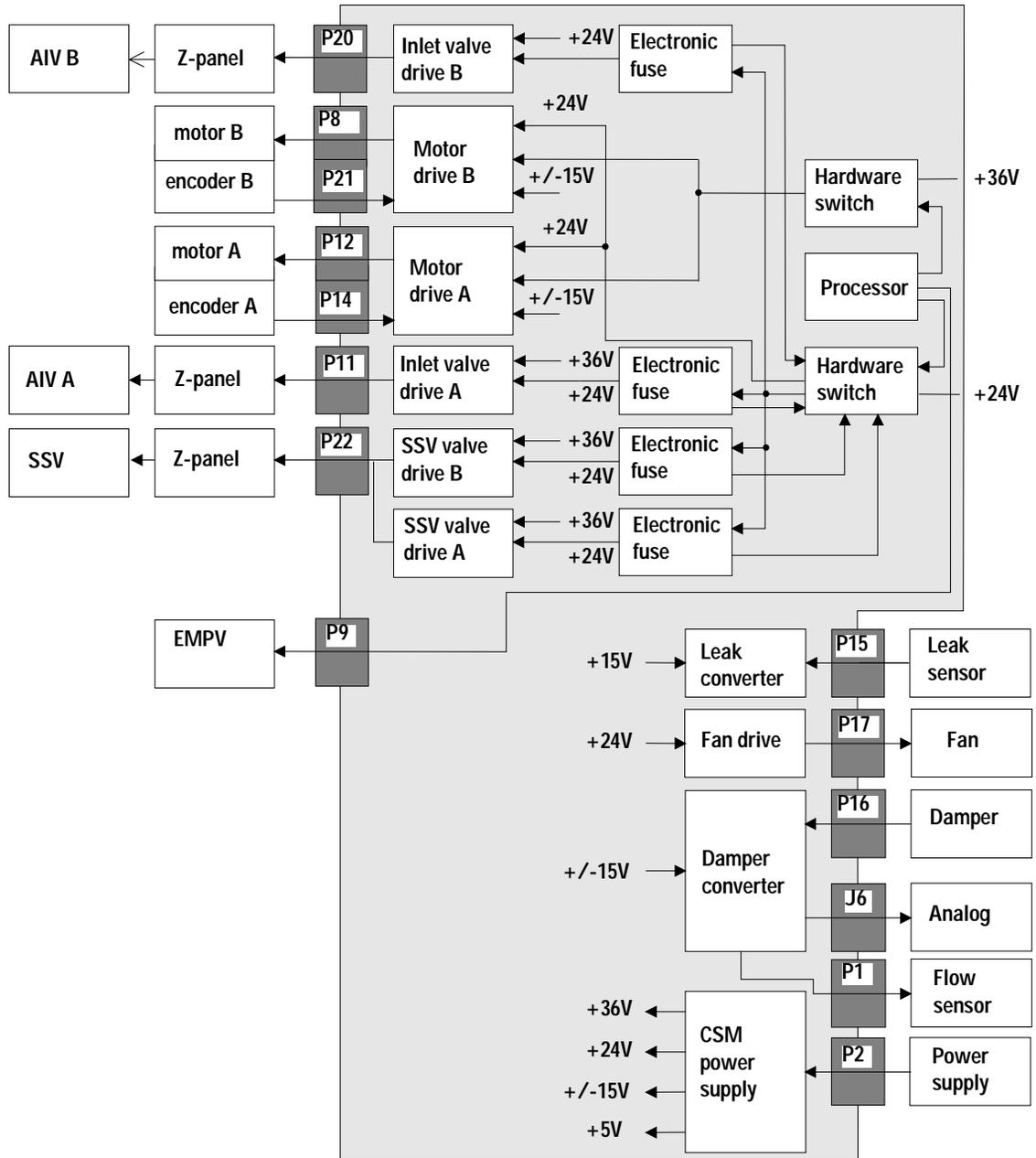
Figure 43 Interconnection Diagram NPM Board
