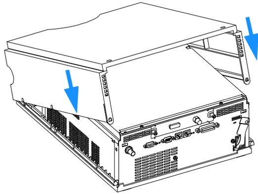
3 Replace the nano pump into the stack and reconnect the cables and capillaries.
