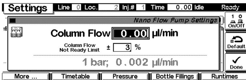
Use the **m**-key for the context sensitive menu. **Reset** will load the pump default parameters. The **Status** command pulls up the module specific setup screen.
