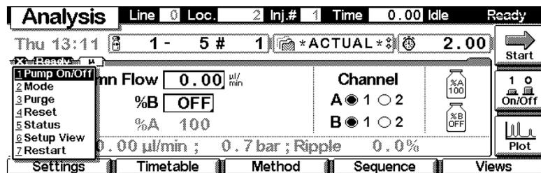
**Setup View** In the Setup view, modules can be added or removed to the analysis view. Select a module, you want to move, with the help of the **selection** keys. Use function keys **F7/F8 (Remove/Add)** to move the highlighted module. Changes must be activated with **Done (F6)**.
