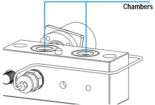
**4** Insert seals into the pump head and press firmly in position.
