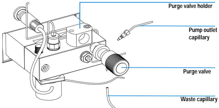
**Figure 18** Exchanging the Purge Valve Frit
