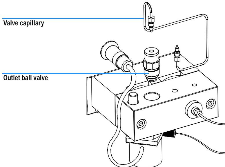
**Figure 17** Exchanging the Outlet Ball Valve
