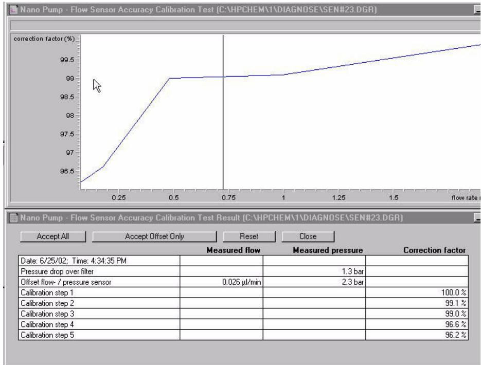
Figure 11 Flow sensor accuracy calibration test evaluation
