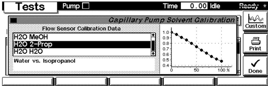
Press **Enter** once you have selected/highlighted a calibration curve to edit the individual data points of this curve. Editing the name of the curve and acknowledging the changes with **F6 (Done)** saves the new data curve with its new name. It is possible to store one individually created calibration curve with each method. Load/Save a calibration curve from/to the PCMCIA-Card by pressing **F8 (PC-Card)**.
