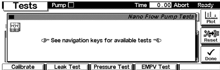
**Calibration** Press **F1 (Calibrate)** to access the pump's calibration screen. Select one of the calibration curves stored on the module with the help of the selection keys.
