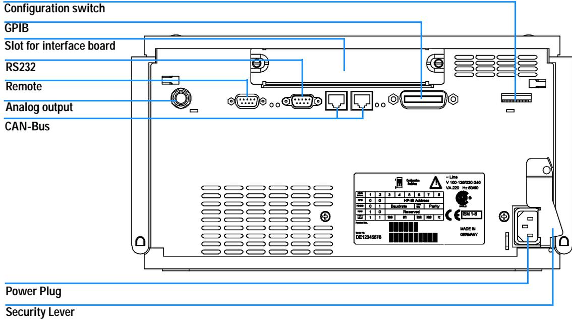
Figure 40 Electrical Connections to the Nano Pump
