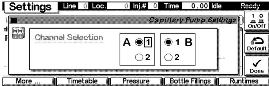
**Settings More...** Select **Auxiliary** to access the pumps performance optimization parameters (Compressibility and Minimum Strike) for each channel individually. Changes must be activated with **F6 (Done)**.
