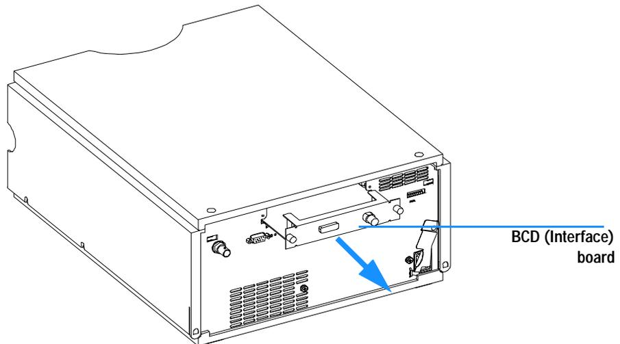
**Figure 21** Exchanging the Interface Board
