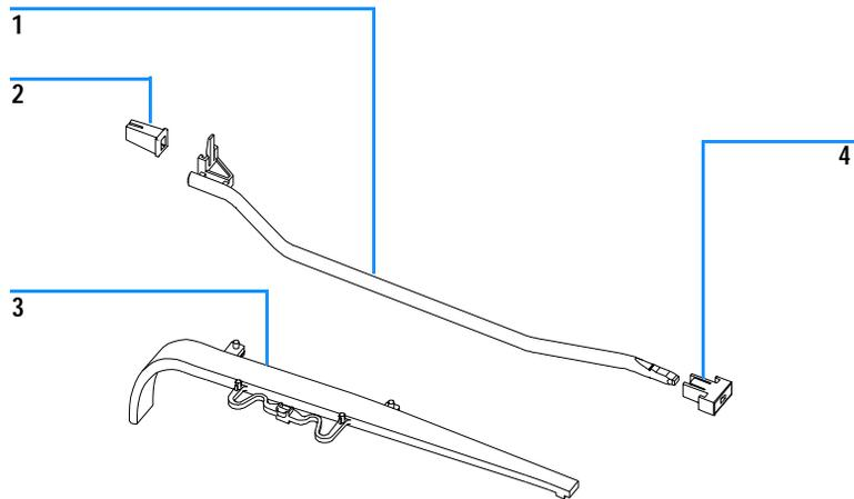
**Figure 31** Power and Status Light Pipes
