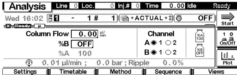
The **m**-key allows access to the context sensitive menus. **Date&Time** allows you to change time settings. **Print Screen** gives access to the print screen. **About** tells you the current firmware revision and the serial# of your control module. **Setup view** leads you to analysis view configuration for additional Agilent 1100 modules. **Restart** re-boots the control module.
