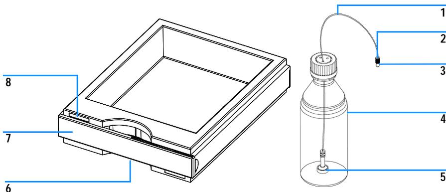
**Figure 26** Solvent cabinet and bottle head assembly
