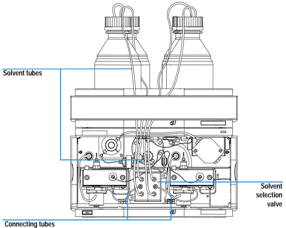
Figure 20 Exchanging the solvent selection valve
