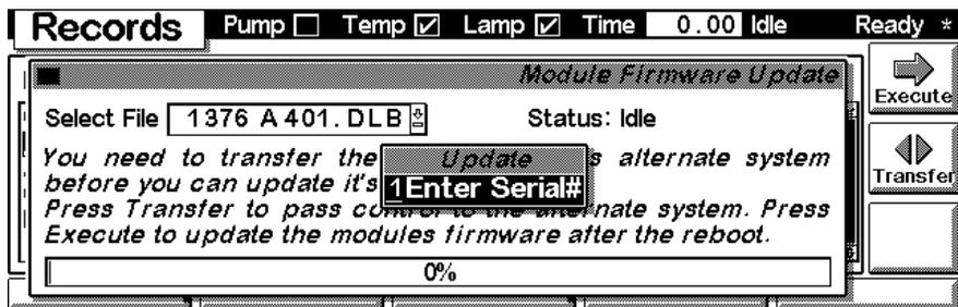
Type in the module's Serial# as indicated on the front or rear label of the module using the alphanumeric keys. Changes must be activated with **F6 (Done)**.
