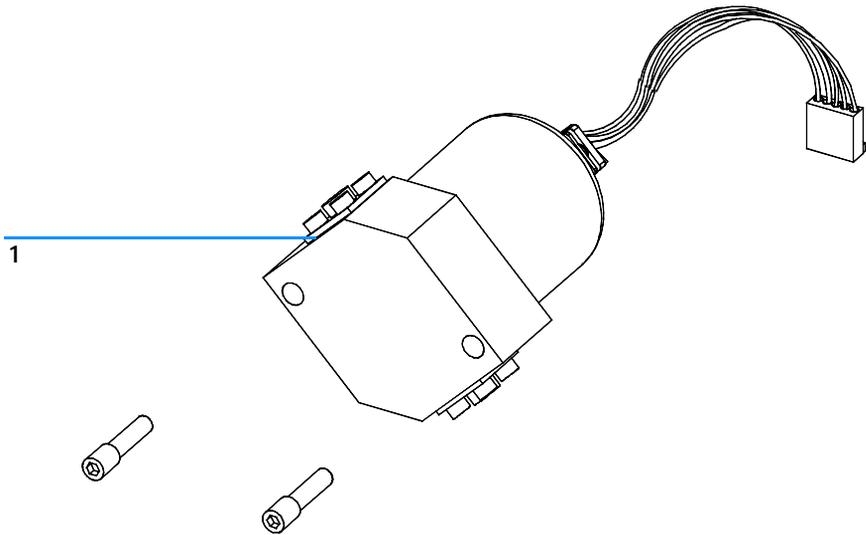
**Figure 30** Flow Sensor Assembly
