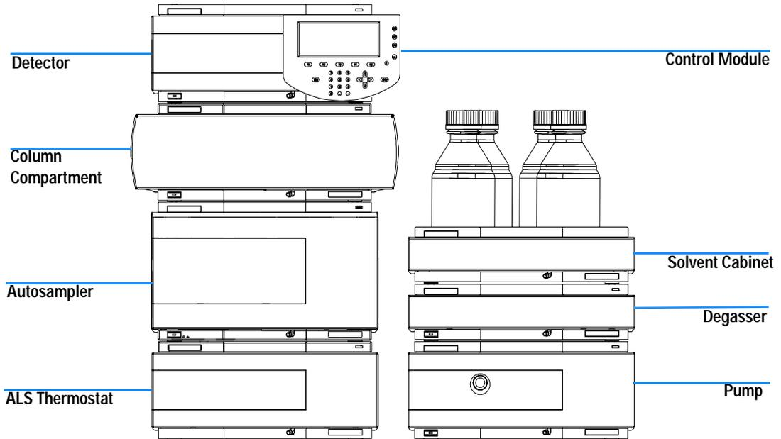
**Figure 3** Recommended stack configuration (front view)
