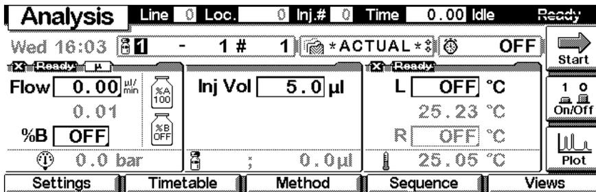
**On/Off** From the Analysis screen use the **F7**-key (**On/Off**) to proceed to the turn on screen. Press **F8 (On)** once to turn on the pump. If more than one module is available, select **F8 (Pump)** or turn on the entire system by selecting the **System On** button and pressing **Enter**.
