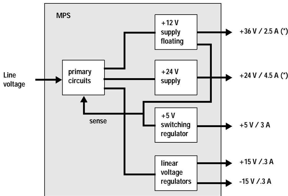
(\*) total power consumption on +36 V and +24 V must not exceed 107 watts.
