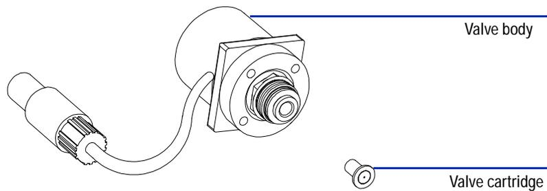
Figure 14 Active Inlet Valve Parts
