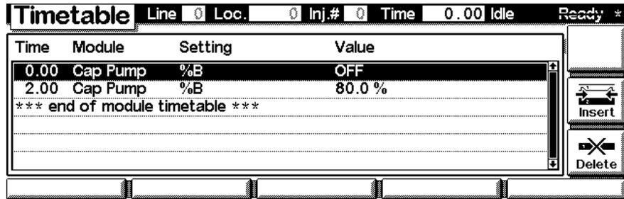
Edit the different sections of each timetable line. Use the pull-down menus, if available. Use the **F6**-key (**Done**) to view the entered lines of the timetable or **F7** (**Enter**) to acknowledge current settings.
