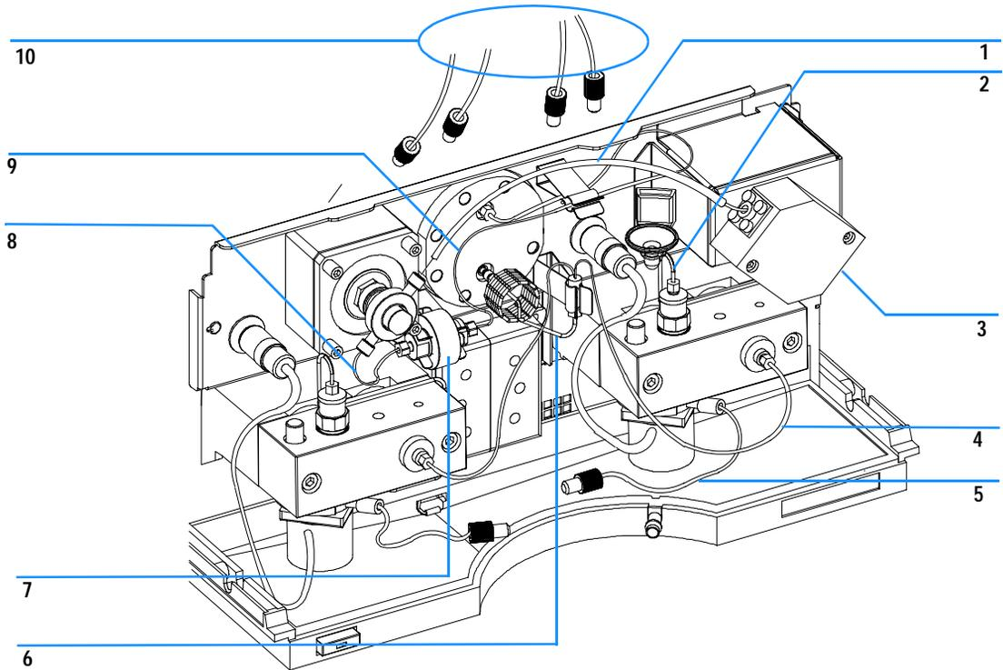
Figure 27 Nano pump hydraulic path
