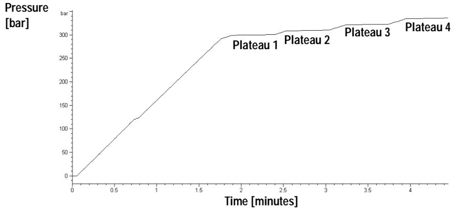
Figure 10 Leak Test Pressure Plot
