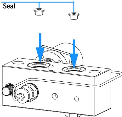
**5** Reassemble the pump head assembly (see "Reassembling the Pump Head Assembly" on page 127). Reset the seal wear counter and liquimeter as described in the User Interface documentation.
