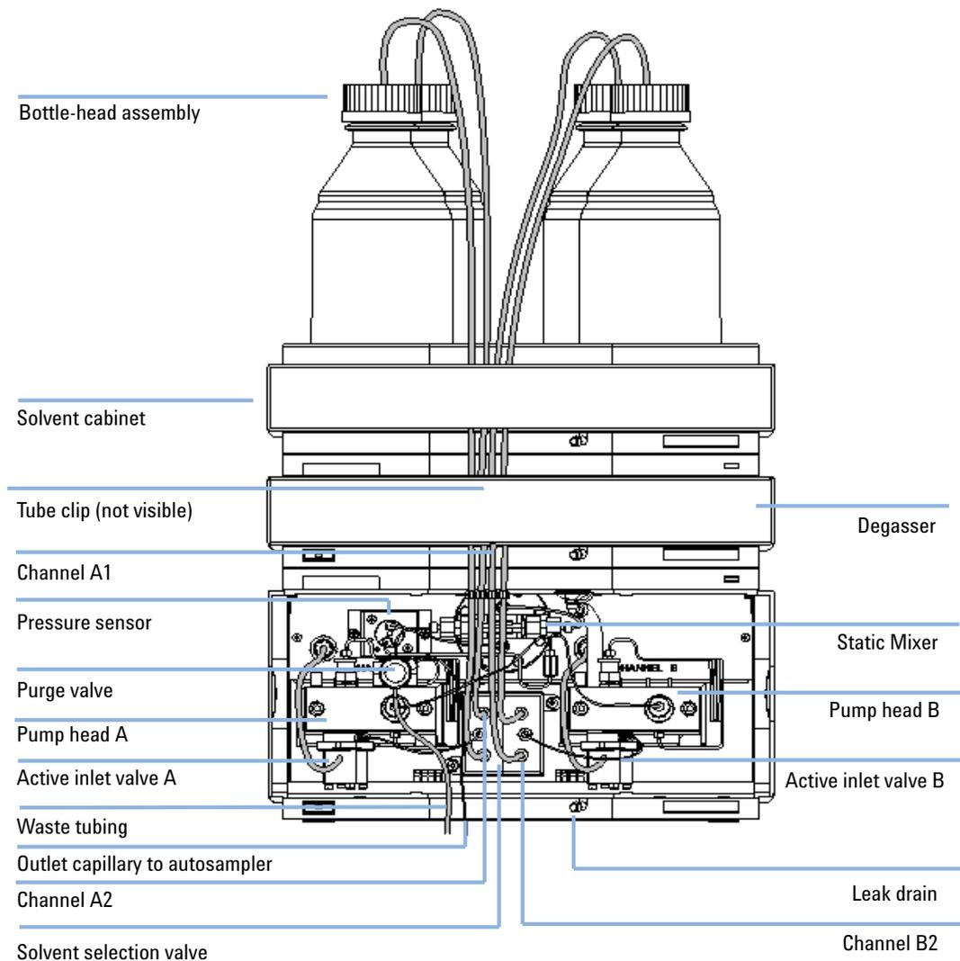
**Figure 13** Binary Pump SL with Solvent Selection Valve
