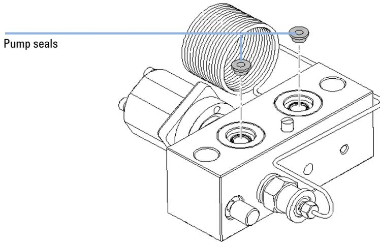
**Figure 29** Inserting of new Pump Seals
