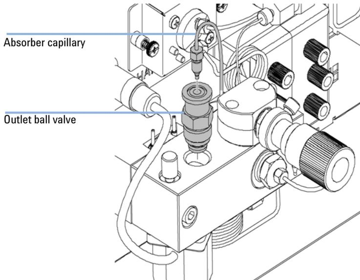
**Figure 36** Outlet Ball Valve Replacement
