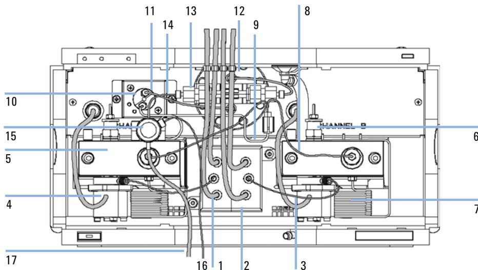
**Figure 40** Hydraulic Path with Solvent Selection Valve
