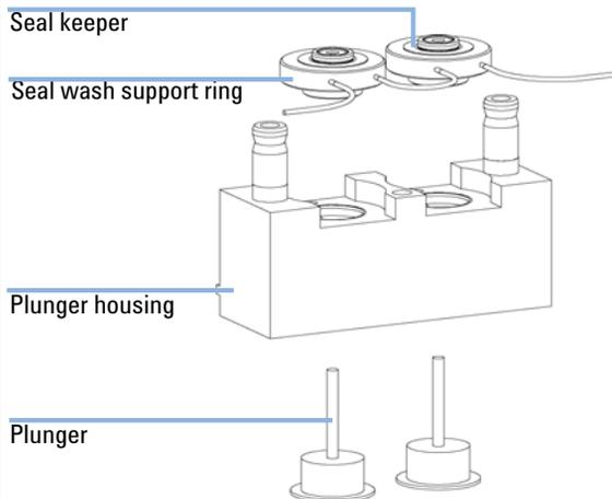
**2** Using the blade of a flat head screwdriver remove seal wash gasket and the secondary seal from the support ring.
