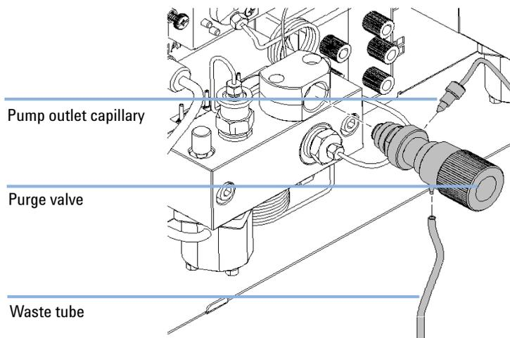
**Figure 26** Exchanging the Purge Valve
