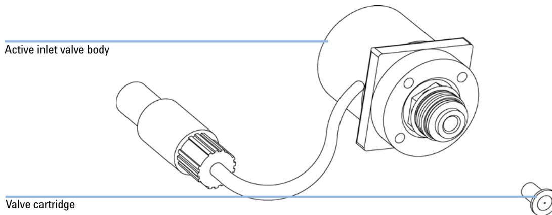
**Figure 32** Replacement of the Active Inlet Valve Cartridge
