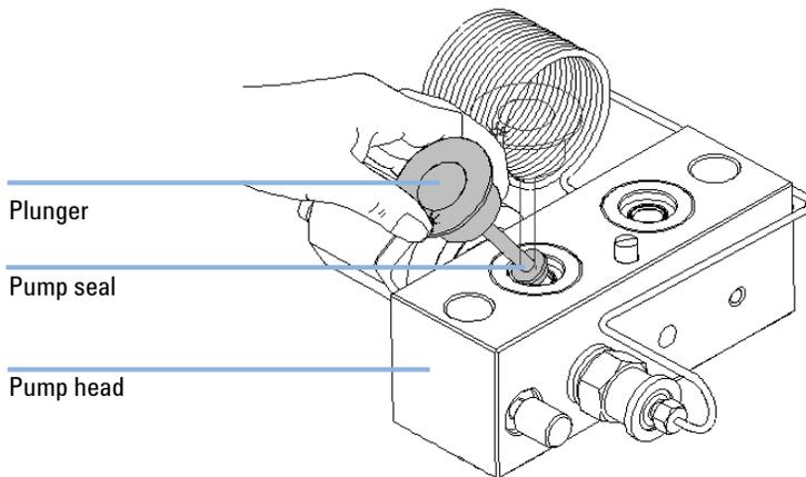
**Figure 28** Removing the Pump Seals from the Pump Head
