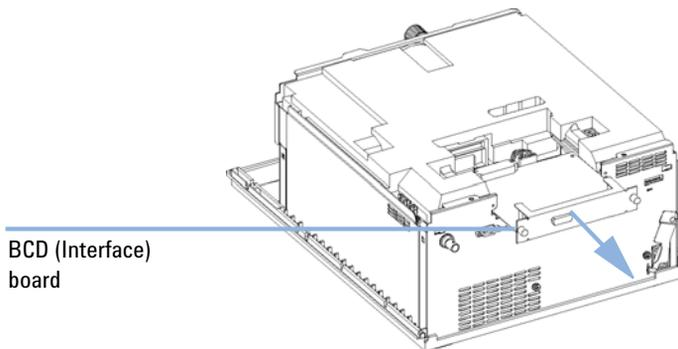
**Figure 38** Exchanging the Interface Board
