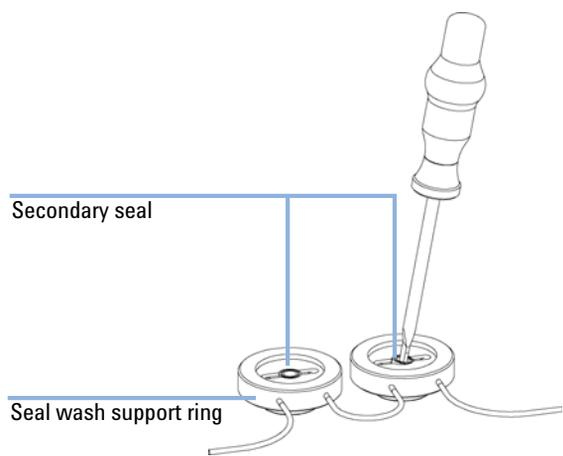
**3** Using the insert tool press the seal (spring pointing upwards) into the recess of the support ring. Place a seal wash gasket in the recess of the support ring and replace the seal keeper.
