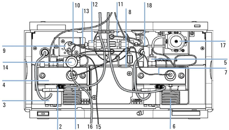
**Figure 41** Hydraulic Path with Solvent Selection Valve, with Active Seal Wash
