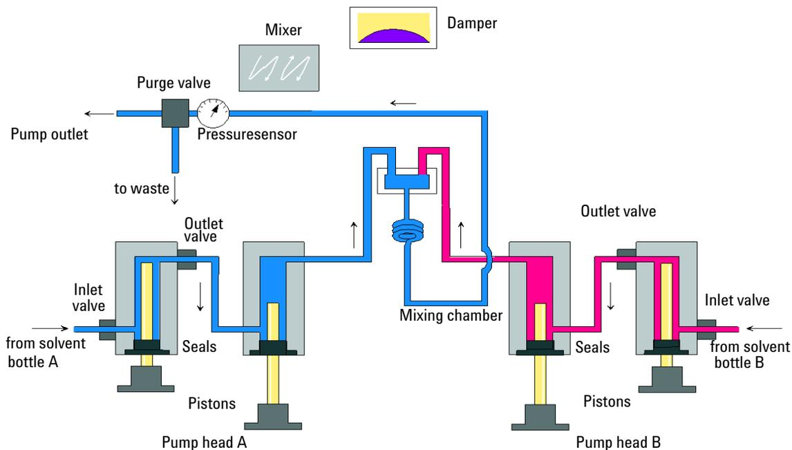
**Figure 2** The Hydraulic Path of the Binary Pump SL with bypassed Damper and Mixer
