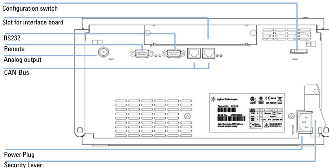
**Figure 11** Rear of the Binary Pump SL
