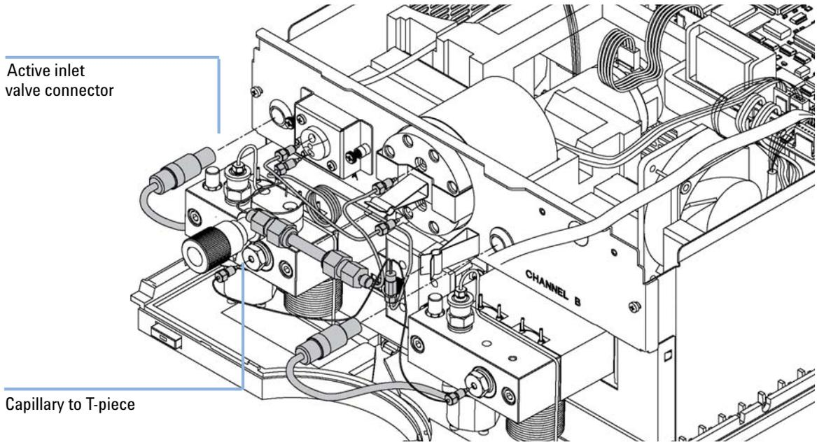
**Figure 31** Reinstallation of Pump head Capillaries and AIV Connector
