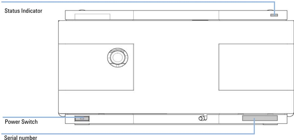
**Figure 10** Front of Binary Pump SL
