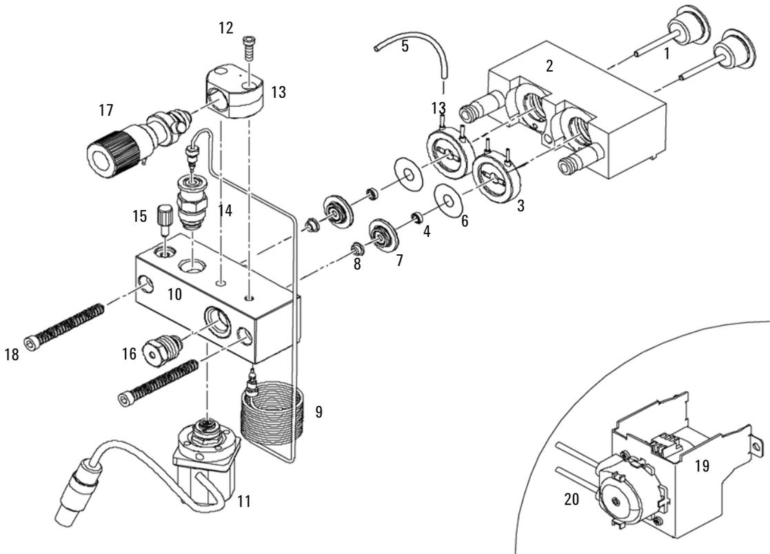
**Figure 42** Pump Head Assembly with Seal Wash Option
