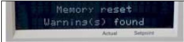
10. To clear the memory reset error, power cycle the GC.
