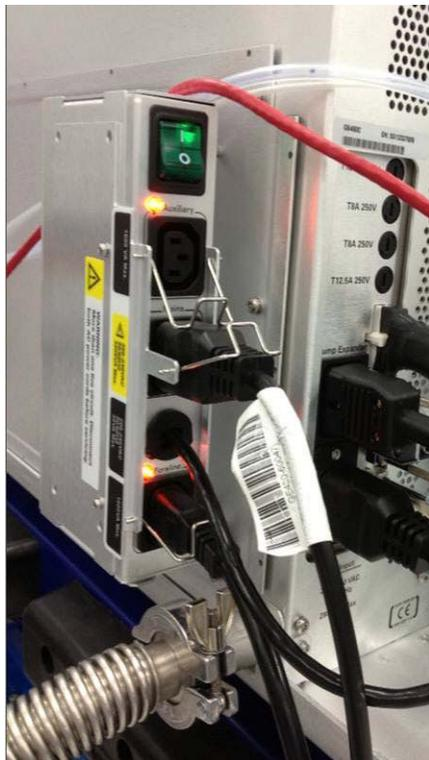
**Figure 13** Pump Expander Assembly box for K6460.
