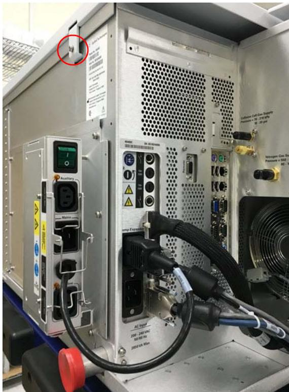
**Figure 4** Remove shipping screws from back of top panel. One of the screws to remove is circled in this picture.
