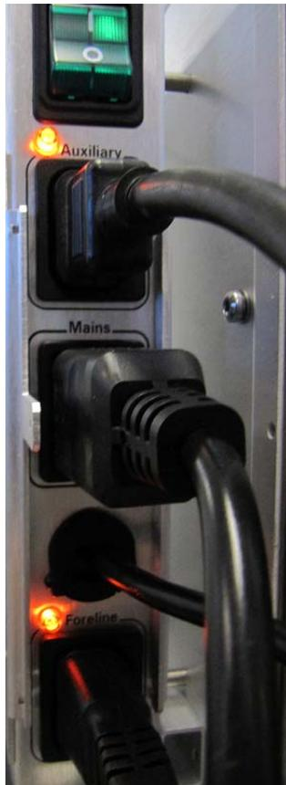
**Figure 7** Pump expander box ports for K6460
