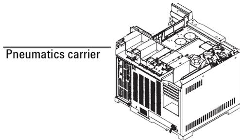
2. If you are installing an inlet in the back position and there is an inlet installed in the front position, unplug the ribbon cable from the pneumatic control board. Unlock the connector by pushing the tabs away from the center.
