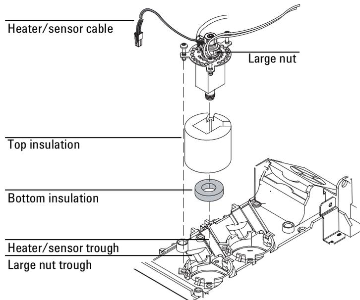
4. From the left side of the GC, locate the heater/sensor wire and its corresponding connector. Tuck the heater/sensor wire underneath the clip at the side of the GC and connect it to the nearest square connector.
