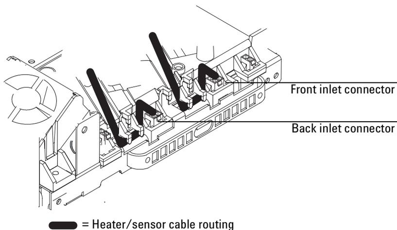
5. Place the trap in in the compartment at the end of the pneumatics carrier. Route the trap's copper tubing behind the fan bracket and to the inlet. Route the trap's stainless steel tubing behind the fan and to the flow manifold. Route the stainless steel tubing from the inlet to the flow manifold.
