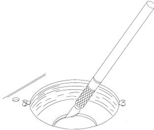
**Method 2:** Pierce the insulation with a screwdriver. Rotate the screwdriver around the scribed circle to remove excess insulation.
