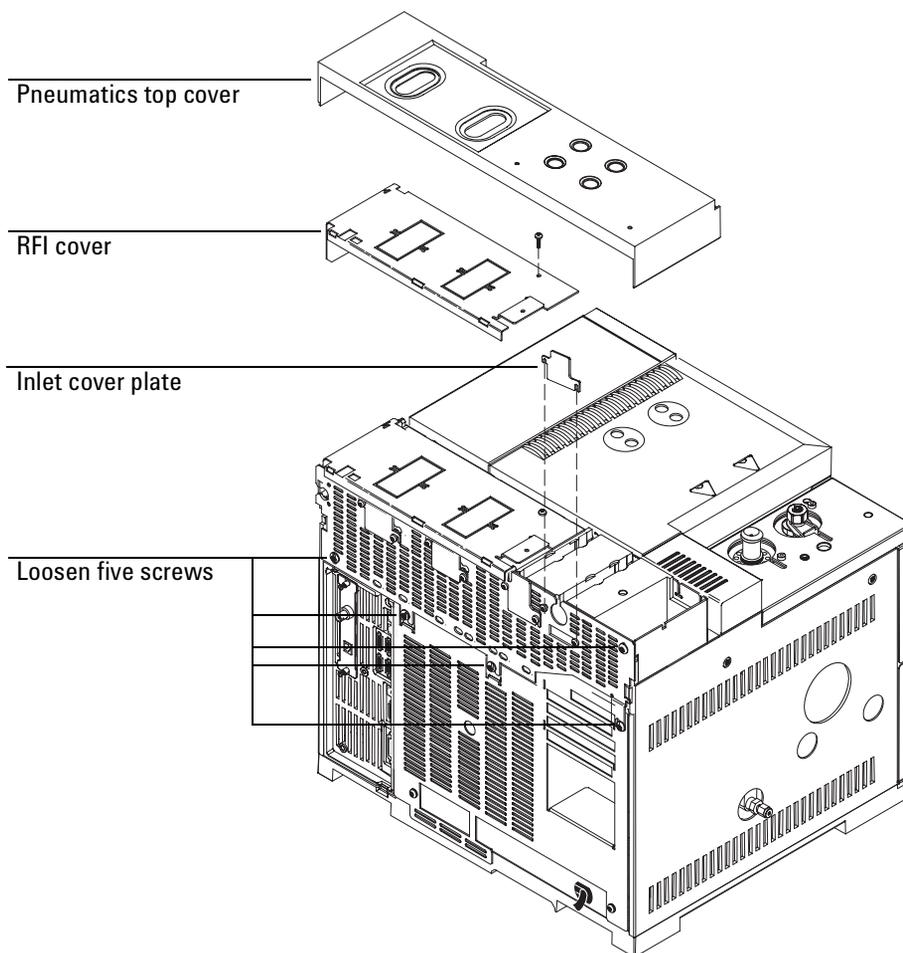
7. Raise the gray plastic top cover (with the holes and ventilation slots) to the vertical position. Examine the hinge in the right rear corner.
