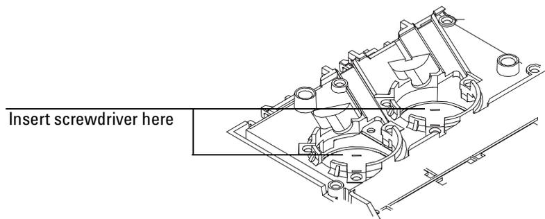
3. Remove the die-cut insulation plug from the front or back inlet position, if necessary.
