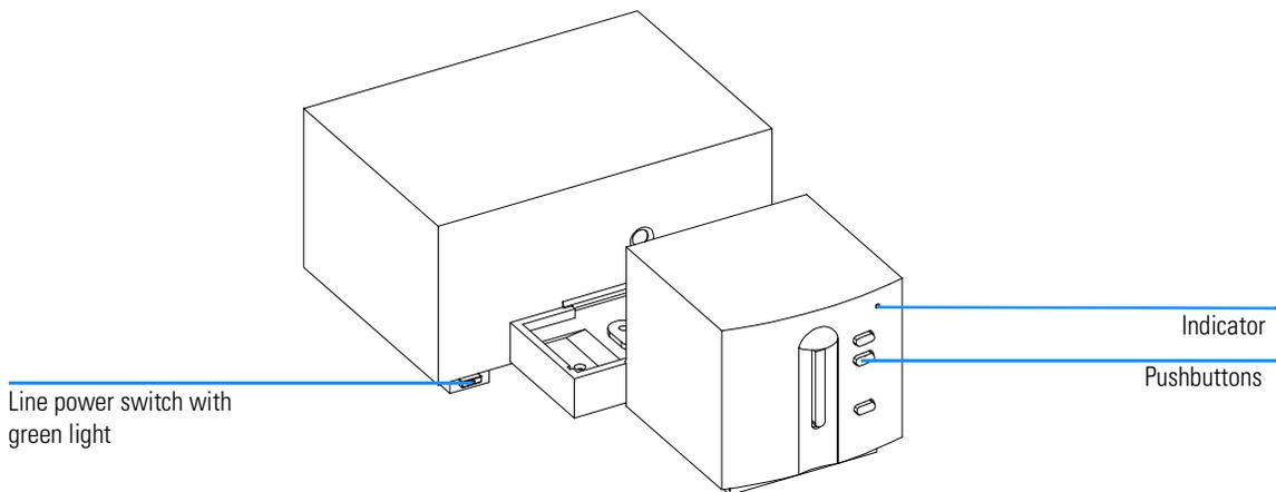
The line power switch is located at the lower-left part of the instrument. Pressing it in turns on the instrument. It stays pressed in and shows a green light when the instrument is turned on. When the line power switch stands out and the green light is off, the instrument is turned off.
