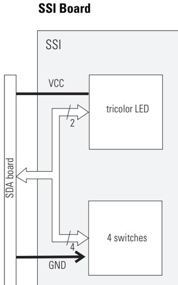
Switches are pulled to GND when pressed, and provide a signal to the SPM board through the low-pass filter on the SDA board. The LED is driven from the SPM board through the low-pass filter on the SDA board.
