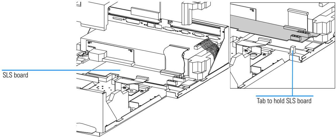
**Replacing the SLS Board**
