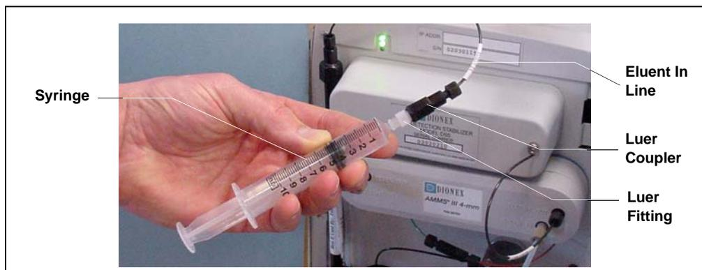
Figure B-22. Assembled Syringe and Luer Adapter
