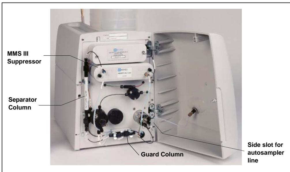
*Figure B-20. ICS-90 with Columns and Suppressor Installed*
