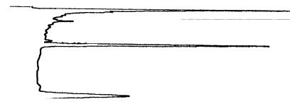
d. The resulting chromatogram should appear similar to that shown in the figure above. The following criteria indicate successful completion of ECD chemical checkout:
