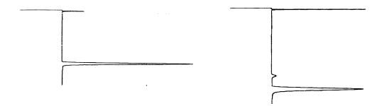
d. Depending upon whether the FPD is in Sulfur or Phosphorus mode, the resulting chromatogram and report should appear similar to one of those shown in Figure 2. The following criteria indicate successful completion of FPD chemical checkout:
