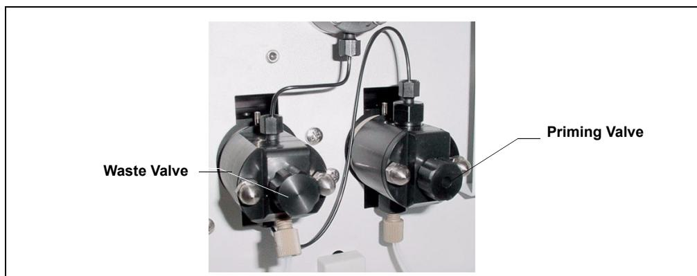
Figure 4-2. Waste and Priming Valves
