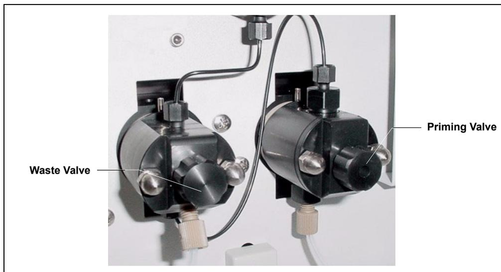
Figure 5-12. Waste and Priming Valves
