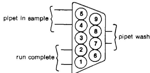
**Figure 2-8. Control Sequencer Output Signals**
