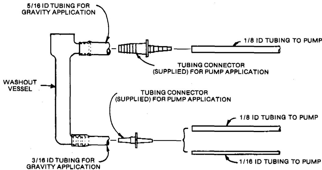
**Figure 5-6. Wash Vessel Tubing Installation**
