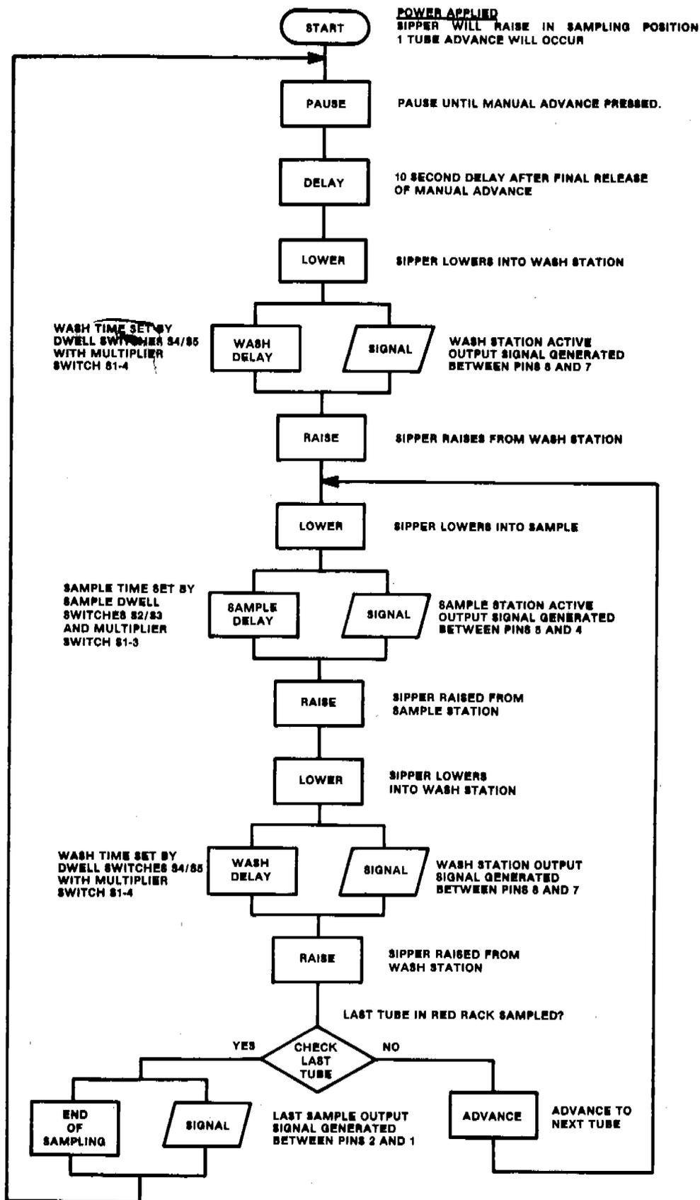
**Figure 3-1. Sequence for the Autosampler with Sequencer and Wash Station**
