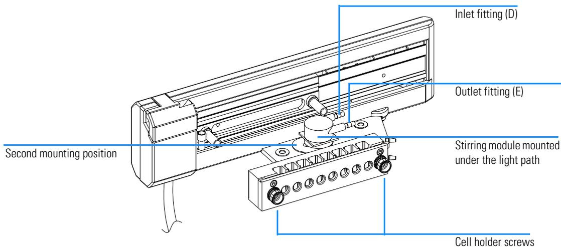
**Installing the Stirring Module**
