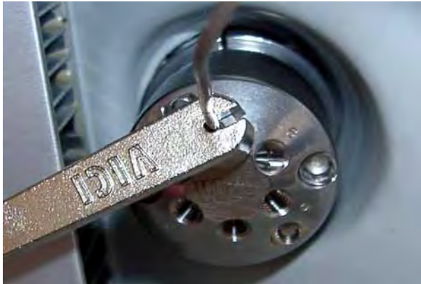
Tighten the fitting screws, using an appropriate tool.
