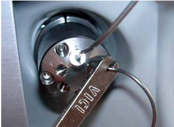
Connect the capillary from valve position 6 to the inlet of either a column or eluent preconditioner (here: to the eluent preconditioner installed in the bottom position in the column chamber.)
