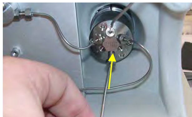
Connect the capillary to the detector inlet to valve position 4.
