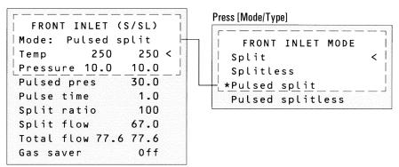
3. Press the [Prep Run] key (see page <u>285</u>) before injecting a sample manually.
