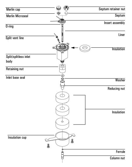
Figure 46 The split/splitless capillary inlet
