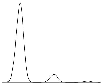
Test plot can be used to verify the operation of external data processing devices without having to perform repeated chromatographic runs. It may also be used as a stable signal to compare the results from different data processing devices.
