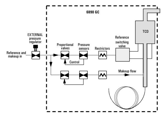
**Figure 8** Internal/external plumbing: TCD *with* EPC For more detail, see <u>"The Thermal Conductivity Detector"</u>.
