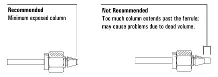
Use the following instructions to install new SWAGELOK nuts and ferrules onto 1/8-inch or 1/4-inch metal columns. If your column already has ferrules installed, proceed to the instructions on installing adapters (page <u>147</u>) or installing packed metal columns (page <u>148</u>).
