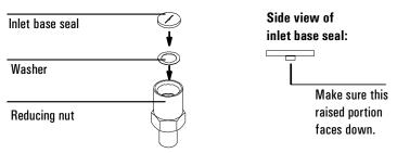
5. Replace the reducing nut. Use the 1/2-inch wrench to tighten the nut. Replace the column and the insulation cup. After the column is installed, you can restore normal operating conditions.
