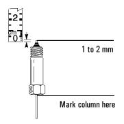
6. Push the column up 1 cm and guide it into the inlet liner. Slide the nut and ferrule up the column to the inlet liner. Adjust the column position so that the correction fluid mark on the column is even with the bottom of the column nut. Finger tighten the column nut until it starts to grab the column.
