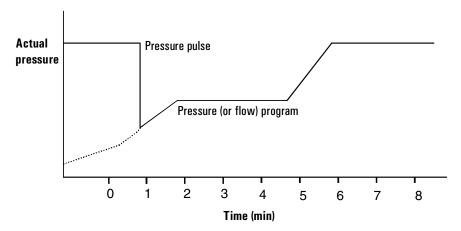
Figure 45 Pressure pulse and column flow or pressure
