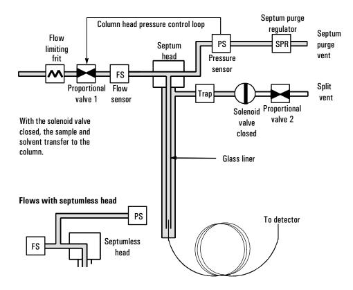
Figure 59 Stage 1. Sample injection
