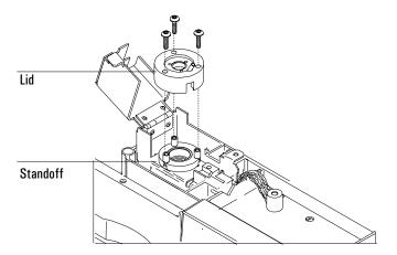
11. Slide the electrometer interconnect into the slot on the lid. Lower the electrometer into the mounting tray.
