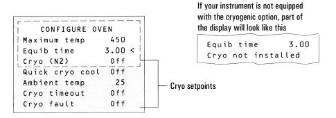
Cryo [ON] enables cryogenic cooling, [OFF] disables it.
