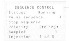
Sequence Control—diplays the current status of the sequence, shows which subsequence is currently active, current sample # or valve position, and which injection number of multiple runs is currently executing.
