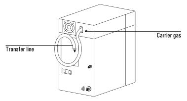
5. Slide the 1/16-inch male nut from step 2 and an appropriate Vespel/graphite ferrule onto the end of the P&T transfer line.
