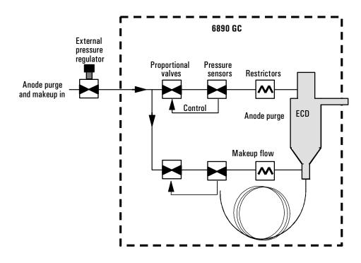
**Figure 9** Internal/external plumbing: ECD *with* EPC For more detail, see <u>"The Micro-Cell Electron Capture Detector"</u>.
