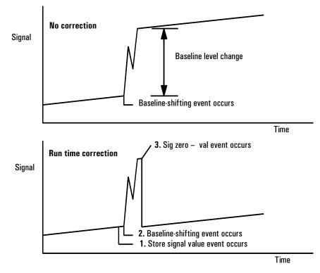
Figure 22 Correcting baseline level shifts in digital signals
