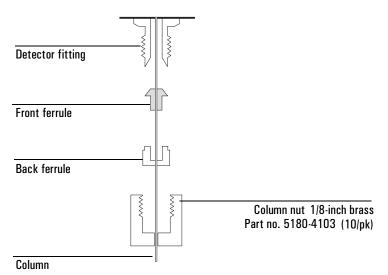
See <u>Table 11</u> for the proper ferrules. Trim off a short piece of column to remove any ferrule fragments inside the column.
