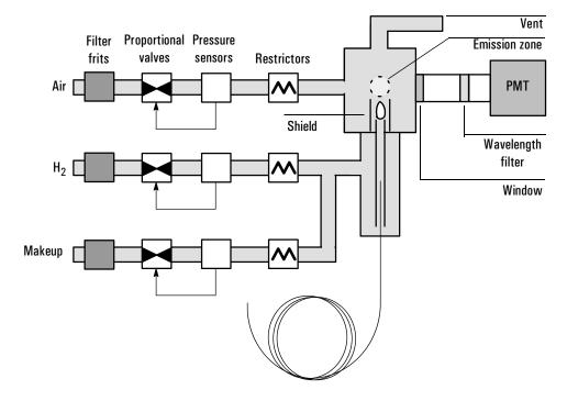
Figure 90. Schematic of a flame photometric detector
