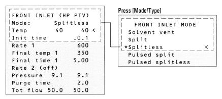
3. Press [Prep Run] (see page <u>285</u>) before manually injecting a sample.
