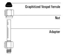
2. Insert the adapter straight into the detector base as far as possible. Hold the adapter in this position and tighten the nut finger tight.
