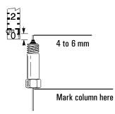
3. Insert the column in the inlet and slide the nut and ferrule up the column to the inlet base. Finger tighten the column nut until it starts to grab the column.
