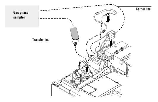
Figure 70 Flow diagram of an external sampling device
