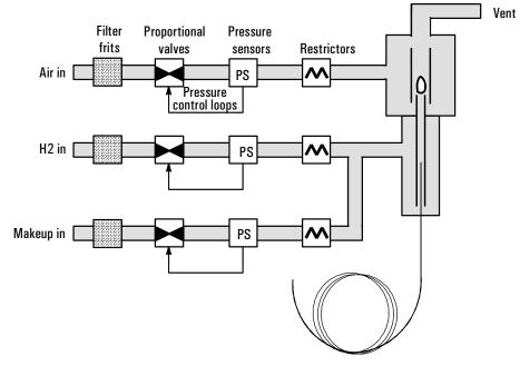
Figure 73 illustrates the pneumatics design for the FID.
