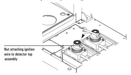
4. The other end of the ignition cable is connected to the detector PC board. Use the figure below to locate the PCB. Make sure to put on the ESD wrist strap at this time and connect it to a proper ground.
