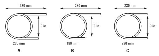
Figure 19. Column Configurations
