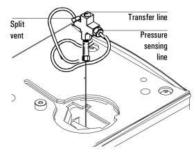
5. Install a blanking nut into the split line port and finger tighten the nut. Tighten the nut an additional 1/4-turn using two wrenches in opposition, the adjustable wrench on the interface and the 1/4-inch wrench on the nut.
