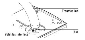
9. After the column is installed at both the interface and the detector, establish a flow of carrier gas through the interface and maintain it for 10 to 15 minutes. Check for leaks. Heat the interface to operating temperatures and retighten the fittings, if necessary.
