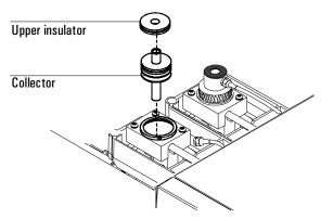
3. Install the upper collector assembly and tighten the knurled nut finger-tight.
