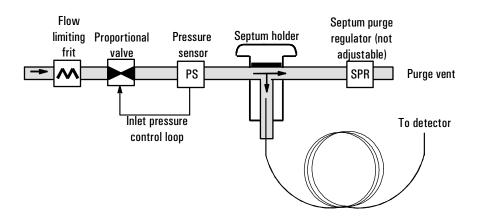
Figure 52 Cool on-column capillary inlet with EPC
