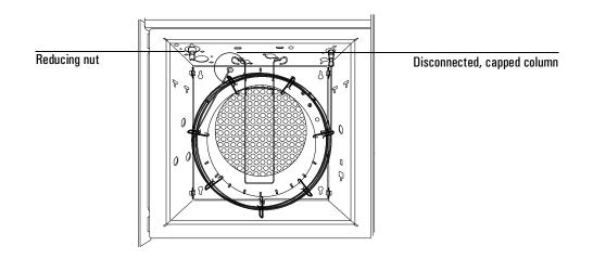
3. Use the 1/2-inch wrench to loosen the reducing nut, and then remove it. The washer and seal are inside the reducing nut. Remove them. You will probably want to replace the washer when you replace the inlet seal.
