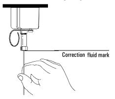
7. Tighten the column nut an additional 1/4 to 1/2 turn so that the column cannot be pulled from the fitting when gentle pressure is applied.
