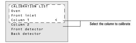
5. The GC displays the current calibration mode for the column. In this example, the column is uncalibrated.
