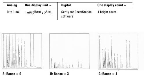
Figure 21 Effect of range setting on chromatogram
