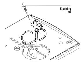
6. Place the interface in the heater block. Replace the clamping plate you removed in Step no. 2 and tighten the screw until snug. Do not overtighten. If you removed the transfer line, replace it.
