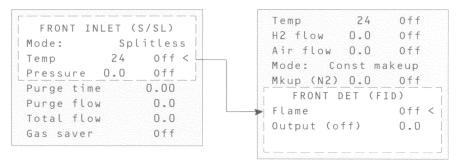
Cursor on Flame, the on/off control for the flame ionization detector
