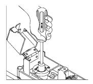
4. Inspect the jet sealing surface for scratches. You should see a small ring around the sealing surface; any other scratches, however, are unacceptable.
