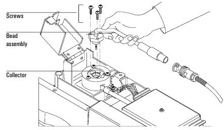
4. Uncap the new bead by pushing the cap off from the cable side. Make sure not to bump the bead on the sides of the cap.
