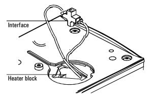
4. From inside the oven, push the column through the opening in the oven top. Grab the column from the oven top.
