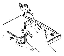
8. Adjust the column position so that the correction fluid mark on the column is even with the bottom of the column nut.
