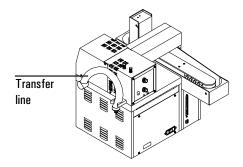
9. Connect the transfer line (with the pre-attached nut and steel ferrule) to the interface. Tighten the nut 1/4-turn past finger tight. Do not overtighten. If the nut leaks, tighten an additional 1/8-turn.
