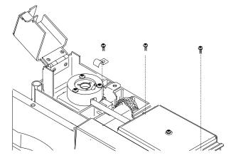
13. Uncap the bead and replace the bead. Replace the three screws. Tighten the first screw only to snugness. Tighten the other screws completely, and then completely tighten the first screw.
