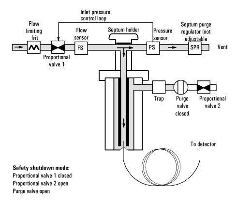
Figure 44 Splitless flow diagram, pre-run to purge time
