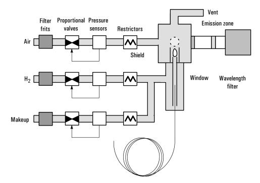
Figure 10 Internal/external plumbing: FPD with EPC
