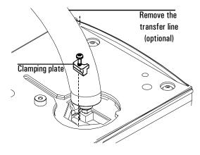
3. Carefully lift the interface out of the heater block.
