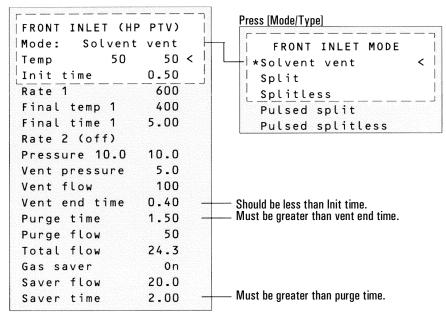
3. Press [Prep Run] (see page <u>285</u>) before manually injecting a sample.
