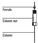
2. Score the column using a glass scribing tool. The score must be square to ensure a clean break.
