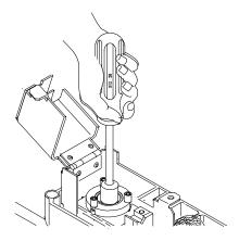
2. Replace the collector assembly. Tighten the three screws securing the collector assembly.
