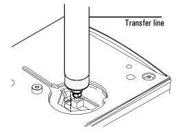
After the column is installed at both interface and detector, establish a flow of carrier gas through the interface and maintain it for 10 to 15 minutes. Check for leaks. Heat the interface to operating temperature and retighten the fittings, if necessary.
