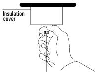
4. Adjust the column position so that the correction fluid mark on the column is even with the bottom of the column nut.
