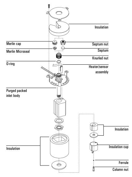
Figure 51 The purged packed inlet
