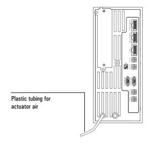
Figure 110. Location of valve actuator air tubing
