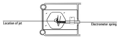
4. Inspect the jet sealing surface for scratches. You should see a ring around the sealing surface; any other scratches, however, are unacceptable.
