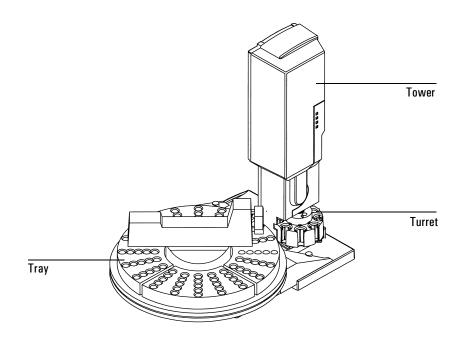
Figure 27 Automatic sampler components
