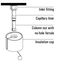
2. Install the insulation cup, if needed. Push the cup spring to the right. Slide the cup over the inlet fitting so that the insulation at the top of the cup is flush against the oven roof.
