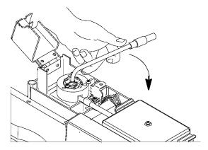
7. Reattach the bead assembly power cable to the NPD power cable and twist the ring to lock the connection.
