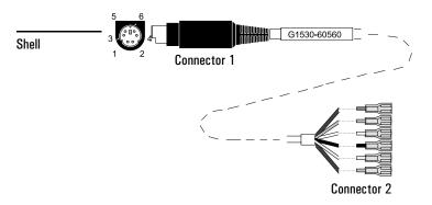
Figure 113. Analog cable, general use (part no. G1530-60560)
