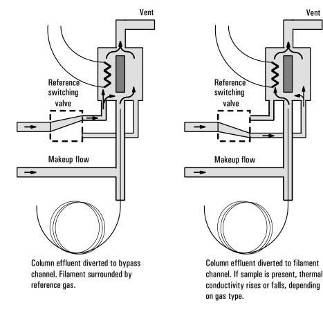
Figure 76. TCD — Conceptual diagram
