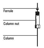
6. Position the column so it extends 6 mm above the end of the ferrule. Mark the column with typewriter correction fluid at a point even with the column nut.
