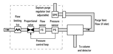
Figure 72 Pneumatics control module
