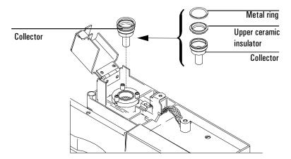
at high temperatures, these parts may stick inside the detector. Push and wiggle them to break the seal.
