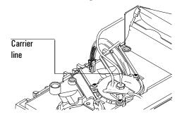
2. Remove the nut and Vespel/graphite ferrule from the carrier line. Keep the parts for later use.
