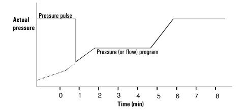
Figure 58 Pressure pulse and column flow or pressure
