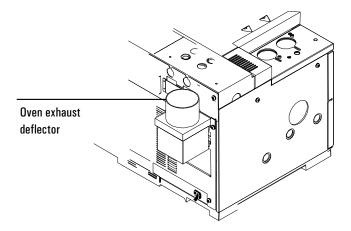
Figure 100. Correct position of the oven exhaust deflector
