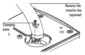
3. Lift the interface out of the heater block.
