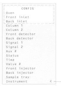
Scroll to the Instrument parameter. Press [Enter] to access the Config Instrument control table. Types shown depend on the installed equipment
