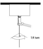
6. After the column is installed at both inlet and detector, establish a flow of carrier gas through the inlet. Heat the oven, inlet, and detector to operating temperature. Allow them to cool, and then retighten the fittings.
