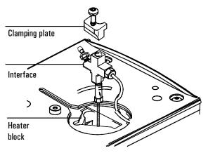
11. After the column is installed at both interface and detector, establish a flow of carrier gas through the interface. Heat the interface to operating temperature. Retighten the fittings, if necessary.
