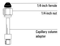
2. Insert the adapter straight into the detector base as far as possible. Hold the adapter in this position and tighten the nut finger tight. Use a wrench to tighten the nut an additional 1/4 turn.
