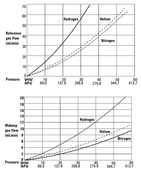
**Figure 79.** Typical pressure/flow relationships, reference and makeup gases (at 25°C and 1 atmosphere of pressure)
