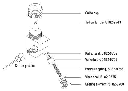
4. Unscrew the guide cap from the head and remove the Teflon ferrule.
