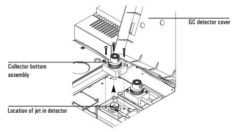
3. Using the nut driver, loosen the jet, and pull it straight out. You may need to use the forceps to grasp the jet.
