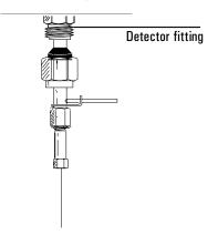
If the adapter is properly installed, the distance between the 1/4-inch nut and the bottom of the adapter will be  $19 \pm 1$  mm. If it is 22–23 mm, reinstall the adapter into the detector fitting.
