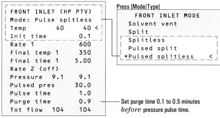
3. Press [Prep Run] (see page <u>285</u>) before manually injecting a sample.
