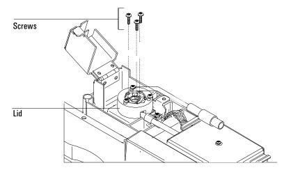
6. Carefully bend the bead assembly cable 90 degrees. You should support the bead as shown below.
