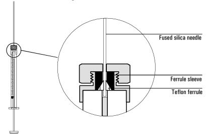
Procedure: Installing a fused silica needle
