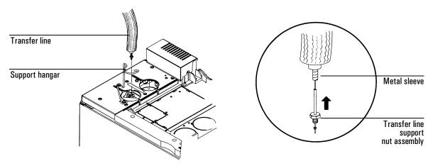
Then, connect the transfer line to the volatiles interface by finger tightening the 1/16-inch male nut while adjusting the transfer line's position so that the correction fluid mark stays aligned with the nut. Using a 1/4-inch wrench,
