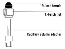
2. Insert the adapter straight into the detector base as far as possible. Hold the adapter in this position and tighten the nut finger tight. Use a wrench to tighten the nut an additional 1/4 turn.
