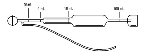
Figure 12 A three-volume bubble meter
