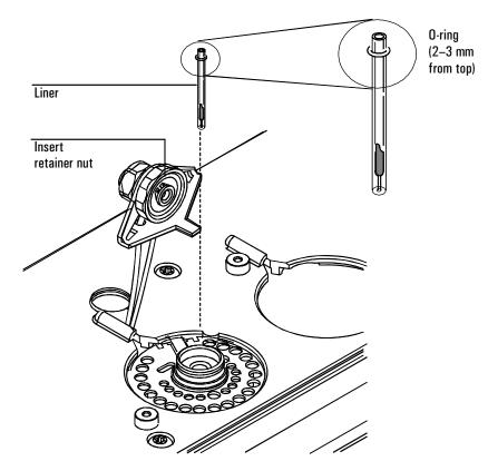
Figure 42 Installing a liner
