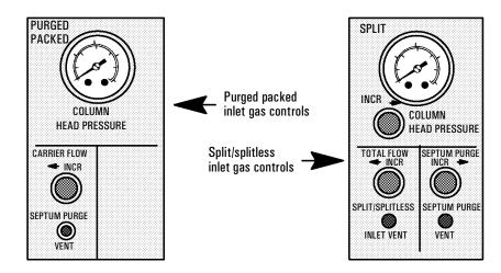
Figure 11 NonEPC inlet gas controls
