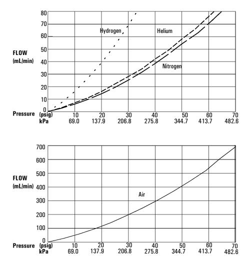
**Figure 74 Typical pressure/flow relationships for FID gases** (at 25°C and 1 atmosphere of pressure)
