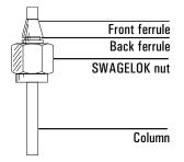
2. Install the Teflon tubing spacer in the male fitting. Fully insert the column with its nut and ferrules into the vise-held fitting. Tighten the nut finger tight.
