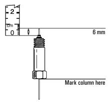
7. Insert the prepared column in the interface and finger tighten the column nut.
