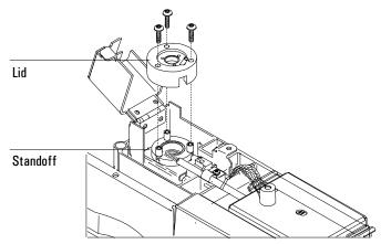
5. Remove the three screws that secure the electrometer and the interconnect. Pull the electrometer away from the detector to free the interconnect. Turn the electrometer to the right to obtain working space.
