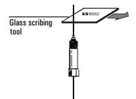
3. Break off the column end by supporting it against the column cutter opposite the scribe. Inspect the end with a magnifying glass to make certain there are no burrs or jagged edges.
