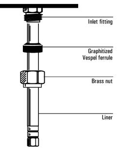
Figure 49 Installing a liner
