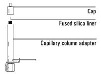
2. Install a 1/4-inch nut and graphitized-Vespel ferrule on the adapter.
