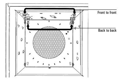
You can install glass packed columns directly in the purged-packed inlet,  $\mu$ -ECD, and adaptable NPD, FID, and FPD fittings. The TCD requires an adapter.
