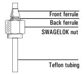
3. Insert the Teflon tubing, ferrules, and nut into the vise-held SWAGELOK fitting. Tighten the nut 3/4 turn past finger tight to set the ferrules on the tubing.
