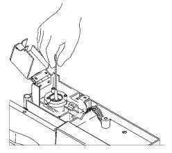
If the collector or the upper ceramic insulator are really dirty, cleaning may not help. Replace with new parts.
