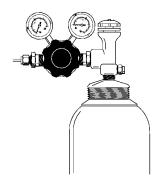
Figure 95. Two-stage pressure regulator
