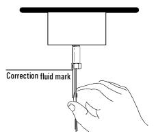
5. Tighten the column nut an additional 1/4 to 1/2 turn so that the column cannot be pulled from the fitting with gentle pressure.
