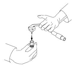
5. Mount the new bead assembly on the NPD lid. Be careful not to bump the bead on the sides of the lid or collector. Replace the three screws. Tighten
