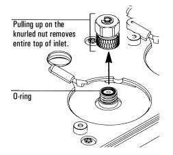
3. Replace the top portion of the inlet and tighten the knurled nut until you cannot tighten it further. Restore the GC to normal operating conditions.
