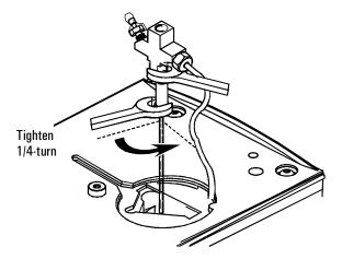
10. Replace the interface in the heater block. Replace the clamping plate and tighten the screw until snug. If you removed the transfer line, reinstall it.
