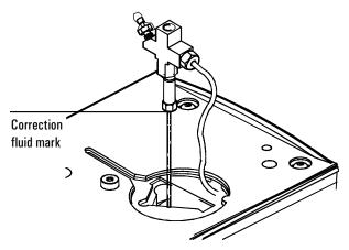
9. Tighten the column nut an additional 1/4- to 1/2-turn. Use the adjustable wrench to hold the interface while you tighten the column nut with the
