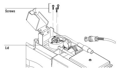
14. Reattach the bead assembly cable to the NPD power cable and twist the ring to lock the connection. Close the NPD cover and the GC detector cover and
