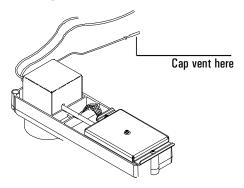
4. Set pressure at the inlet to 15 psi (103 kPa). Monitor the system pressure from the inlet. Allow time for the system to become fully pressurized (at least 1 minute). When the system is fully pressurized turn off the pressure or the gas.
