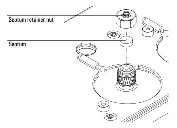
If the septum sticks, use the sharp-tipped tool to remove it. Take care not to gouge the metal around the septum and to remove all pieces of the old septum.
