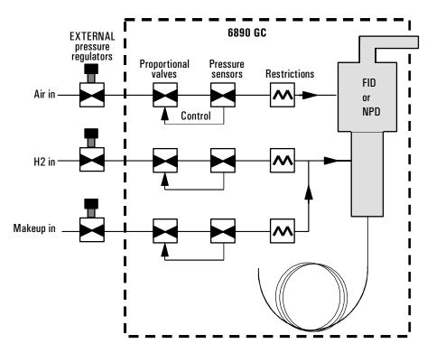
Figure 7Internal/external plumbing: FID and NPD with EPCFor more detail, see "The Flame Ionization Detector", "The Nitrogen-PhosphorusDetector".
