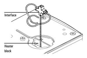
4. If a column is installed, remove it.
