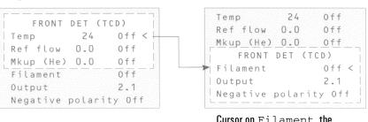
Cursor on Filament, the On/Off line for the thermal conductivity detector With a nondetector control table, [Det Control] opens the front detector control table (or back, if a front detector is not installed). The cursor is at the on/off control for that detector.
