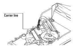
2. Remove the male fitting and Vespel/graphite ferrule from the carrier line. Keep the parts for later use.
