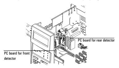
5. To disconnect the cable connection, squeeze the lock and gently pull the connector free. Attach the new ignitor cable by squeezing the lock and sliding the connector into the slot.
