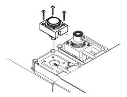
2. Replace the collector and install the upper Teflon insulator.
