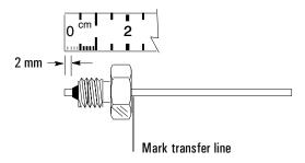
8. To connect the transfer line to the volatiles interface, first install the transfer line support nut assembly up and inside the metal sleeve of the heated transfer line assembly.
