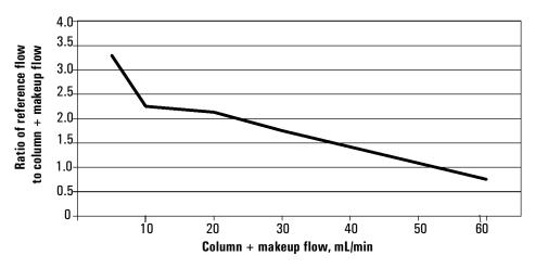
Figure 78. Selecting the reference gas flow
