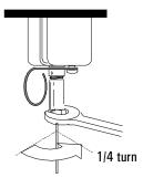
8. After the column is installed at both inlet and detector, establish a flow of carrier gas through the inlet. Heat the oven, inlet, and detector to operating temperatures. Allow these to cool, and then retighten the fittings.
