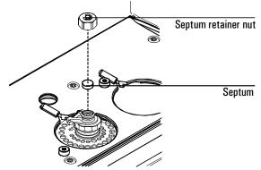
3. If pieces of the septum are sticking, use a small piece of rolled-up steel wool and forceps or tweezers to scrub the residue from the retainer nut and septum
