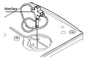
4. Loosen the hex nut connecting the split vent line to the interface until you can remove the line. Put the line aside. You do not need to plug it.
