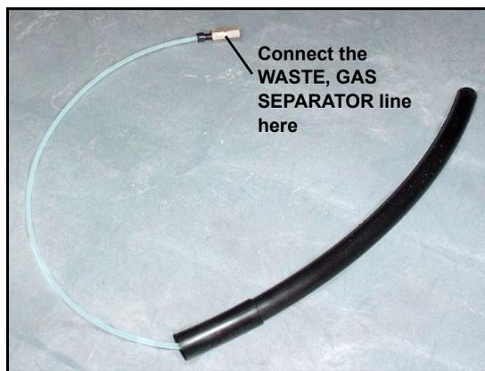
Figure 21. Gas Separator Waste Tube Assembly
