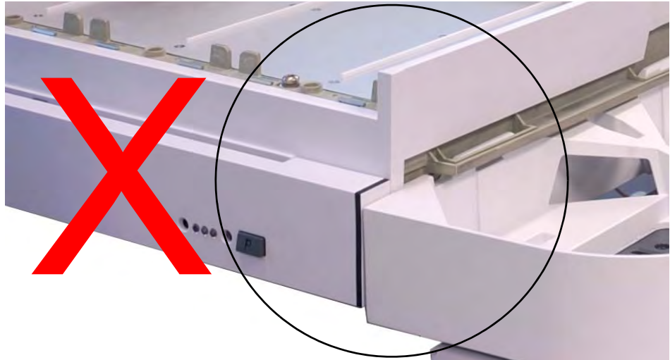
Figure 6 Sample tray incorrectly installed.
