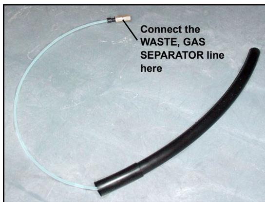
*Figure B-21. Gas Separator Waste Tube Assembly*
