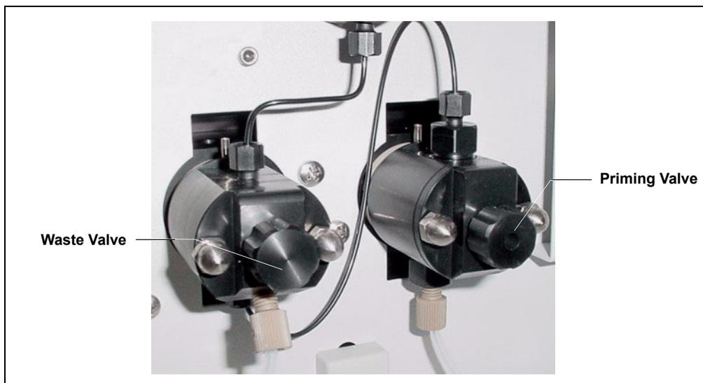
Figure 5-13. Waste and Priming Valves
