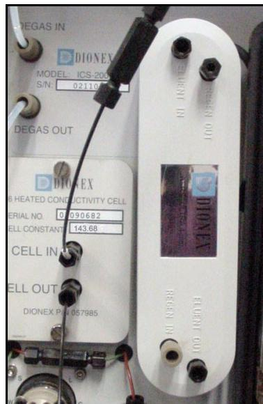
*Figure B-20. Suppressor Installed (SRS Shown)*
