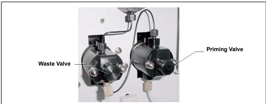
Figure 4-2. Waste and Priming Valves
