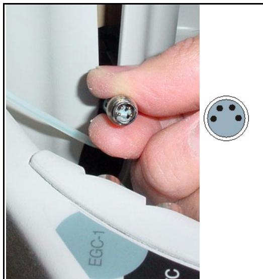
Figure 5-37. Connecting the EGC Cable
