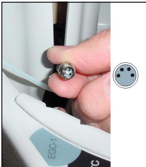
Figure B-40. Connecting the EGC Cable
