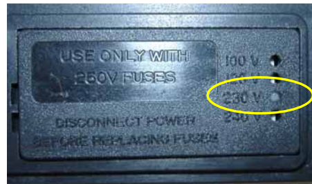
Fig. 3: Factory-set voltage selection, here: 230V
