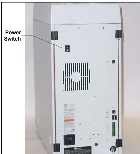
Press the power switch on the ICS-1000 rear panel (see [Figure 3-3](#)) to turn on the system power. [Table 3-2](#) shows the ICS-1000 conditions at power up.
