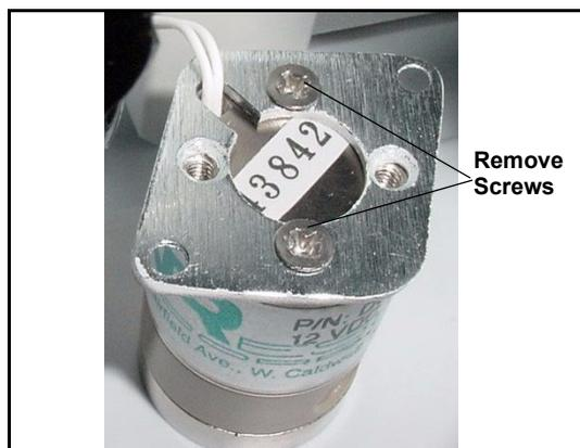
Figure 5-17. Removing the Valve Mounting Plate
