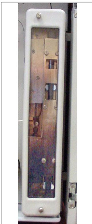
The column heater provides temperature control for the separator and guard column.
