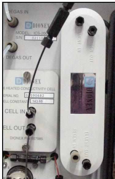
*Figure B-20. Suppressor Installed
