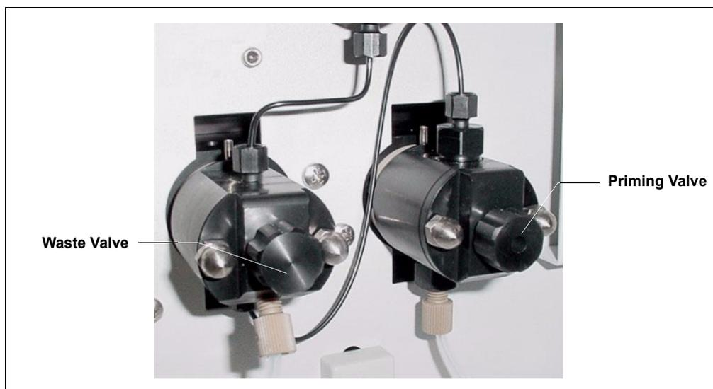
Figure 5-7. Waste and Priming Valves
