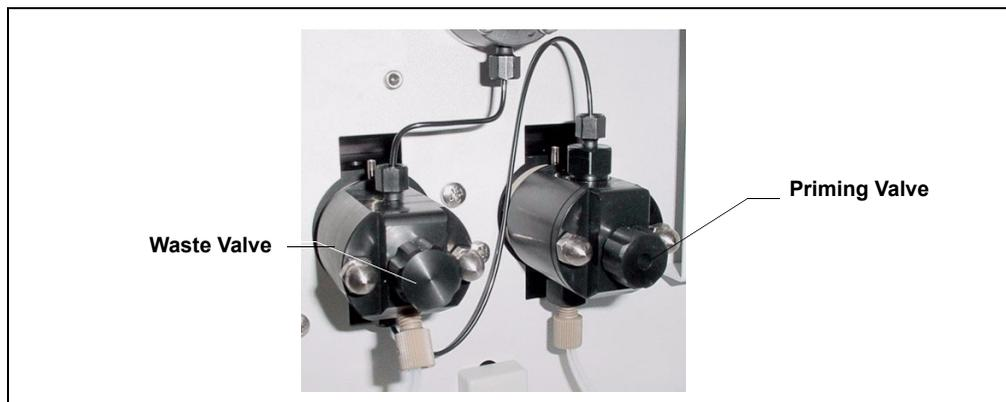
Figure 4-2. Waste and Priming Valves
