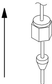
7. Connect the carrier line to the gas supply port by holding the reducer with one 5/16-in. wrench while tightening the 1/16-in. female Swagelok nut with another 5/16-in. wrench. Tighten the fitting 1/4 turn past finger tight. Do not overtighten. If the fitting leaks, tighten an additional 1/8 turn until it seals.
