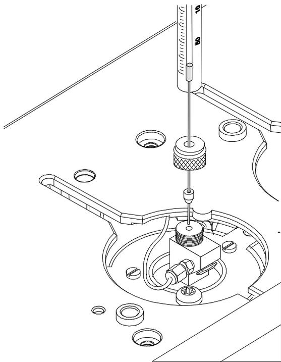
2. Push the guide cap and the new Teflon ferrule over the syringe needle so that at least 10 mm of the needle tip is exposed.
