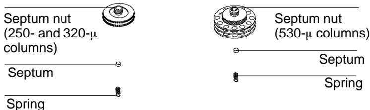
Make sure the spring is in the inlet. Use the tweezers to place a new septum on the bottom of the septum nut, and then reattach the septum nut to the inlet. Tighten the nut firmly.
