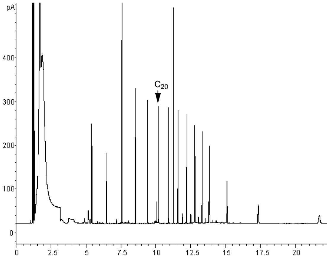
These results were compared with a splitless analysis of the same sample, which should produce 100% recovery of all analytes. The data showed that, under these conditions, compounds above  $C_{20}$  were completely recovered and that the recovery was independent of injection size; Compounds lower than  $C_{20}$  were partially vented with the solvent.
