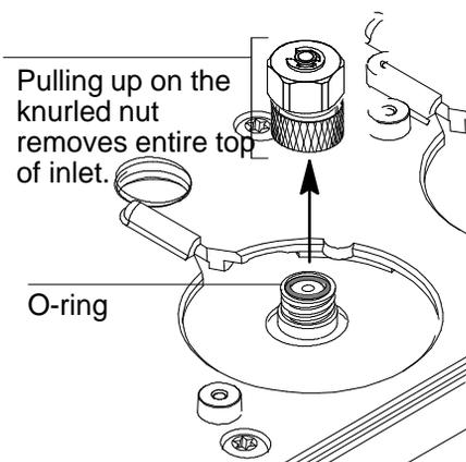
4. Replace the top portion of the inlet and tighten the knurled nut until you cannot tighten it further. Restore the GC to normal operating conditions.
