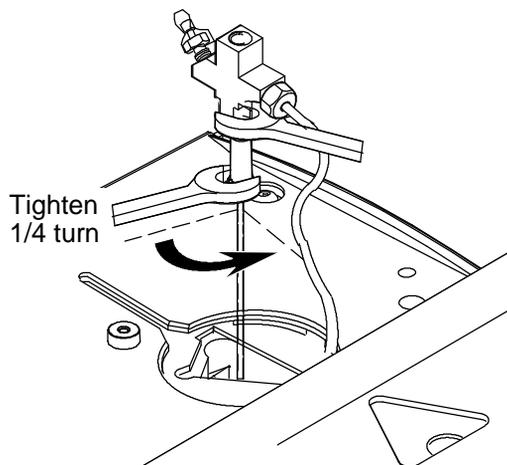
11. Replace the interface in the heater block. Replace the clamping plate and tighten the screw until snug. If you removed the transfer line, reinstall it.
