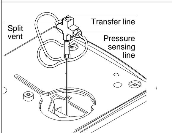
5. Install a blanking nut into the split line port and finger tighten the nut. Tighten the nut an additional 1/4 turn using two wrenches in opposition, the adjustable wrench on the interface and the 1/4-in wrench on the nut.
