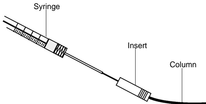
3. Insert the syringe needle through the other end of the insert and into the column. If the needle cannot pass easily into the column, reverse the insert to try the needle and column in the other end.
