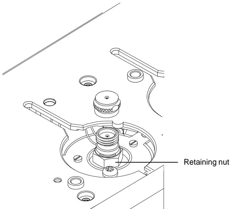
**Procedure: Removing the septum head**
