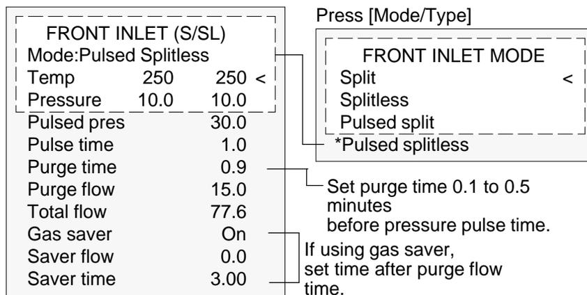
3. Press the [Prep Run] key (see page 13) before injecting a sample manually.
