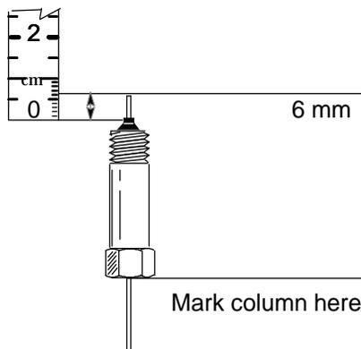
8. Insert the prepared column in the interface and finger tighten the column nut.
