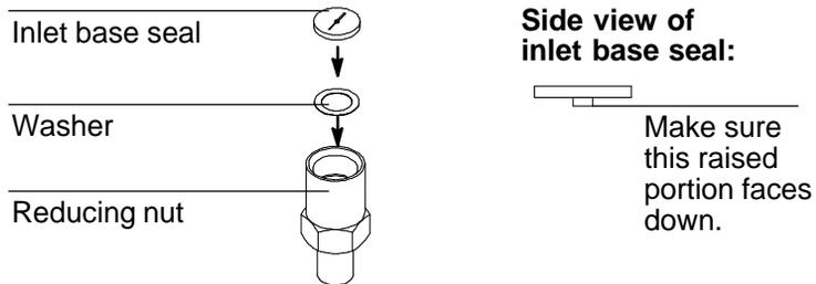
5. Replace the reducing nut. Use the 1/2-in. wrench to tighten the nut. Replace the column and the insulation cup. If you are not sure how to do so, see the General Information volume. After the column is installed, you can restore normal operating conditions.
