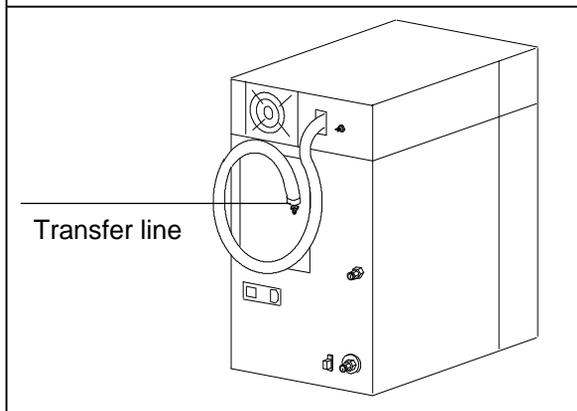
6. Slide the 1/16-in. male nut from step 2 and then an appropriate Vespel/graphite ferrule onto the end of the transfer line.
