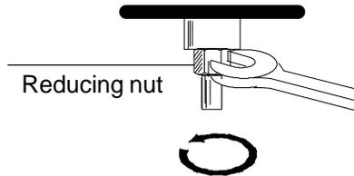
4. Put on the gloves to protect the inlet base seal and washer from contamination. Place the washer in the reducing nut. Place the new inlet base seal on top of it.
