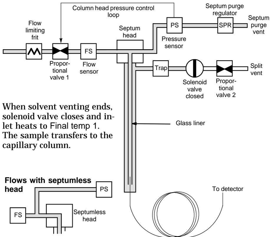
When solvent venting ends, solenoid valve closes and inlet heats to Final temp 1. The sample transfers to the capillary column.
