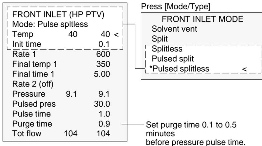
3. Press [Prep Run] (see page 13) before manually injecting a sample.
