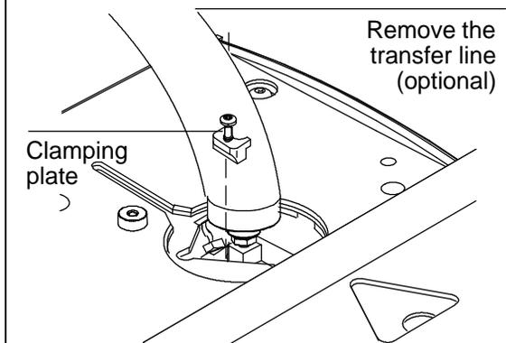
3. Lift the interface out of the heater block.
