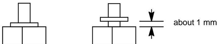
With higher inlet pressures, tighten the septum retainer until the C-ring stops turning, indicating that the retainer is in firm contact with the septum. Then tighten one additional full turn.
