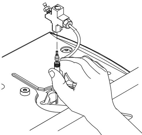
9. Adjust the column position so that the correction fluid mark on the column is even with the bottom of the column nut.
