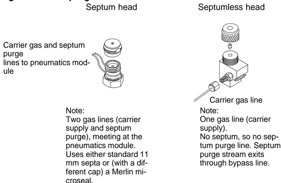
The flow diagrams in the rest of this book show the septum head in place with a separate drawing for the septumless head plumbing.
