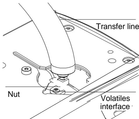
**Procedure: Connecting the HP 7695 purge and trap concentrator**
