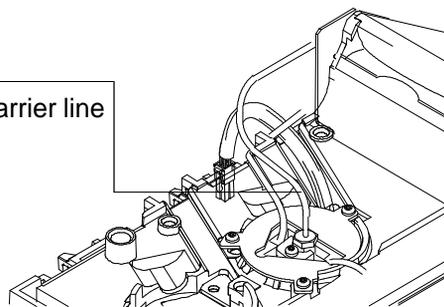
2. Remove the male fitting and Vespel/graphite ferrule from the carrier line. Keep the ferrule in a safe place.
