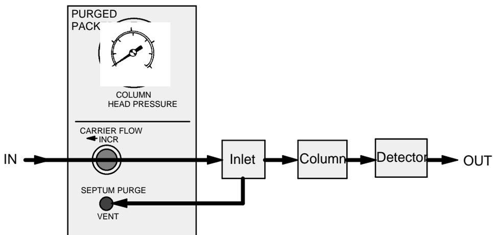
1. Locate the knob labeled CARRIER FLOW. Turn it clockwise as far as it will go. Do not force the knob; when it closes it comes to a slightly “soft” stop.
