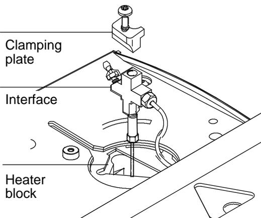
After the column is installed at both interface and detector, establish a flow of carrier gas through the interface. Heat the interface to operating temperature. Retighten the fittings, if necessary.
