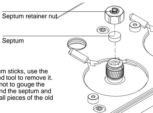
3. If pieces of the septum are sticking, grasp a small piece of rolled-up 0- or 00-grade steel wool with the forceps (or tweezers), and scrub the residue from the retainer nut and septum holder. Use the compressed air or nitrogen to blow away the pieces of steel wool and septum.
