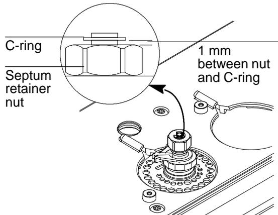
Do not overtighten the nut! Over-tightening over-compresses the septum, which causes premature failure and pieces of septum to fall in the inlet.
