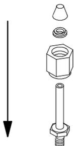
5. Connect the reducer to the gas supply port labeled "Carrier" on the back of the headspace sampler by tightening the 1/8-in. female Swagelok nut using a 7/16-in. wrench. Tighten the nut 1/4 turn past finger tight.
