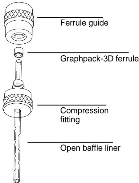
4. Slide the compression fitting onto the longer straight end of the new liner with the threads pointing toward the end of the liner.
