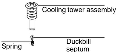
Insert the duckbill septum into the spring and place them in the inlet. Reattach the cooling tower assembly. Tighten it finger-tight.
