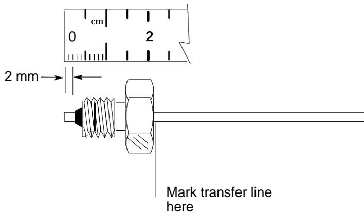
7. Connect the transfer line to the volatiles interface by finger tightening the 1/16-in. male nut while adjusting the transfer line's position so that the correction fluid mark stays aligned with the nut. Using a 1/4-in. wrench, tighten the nut 1/4 turn past finger tight. Do not overtighten. If the fitting leaks, tighten an additional 1/8 turn until it seals.
