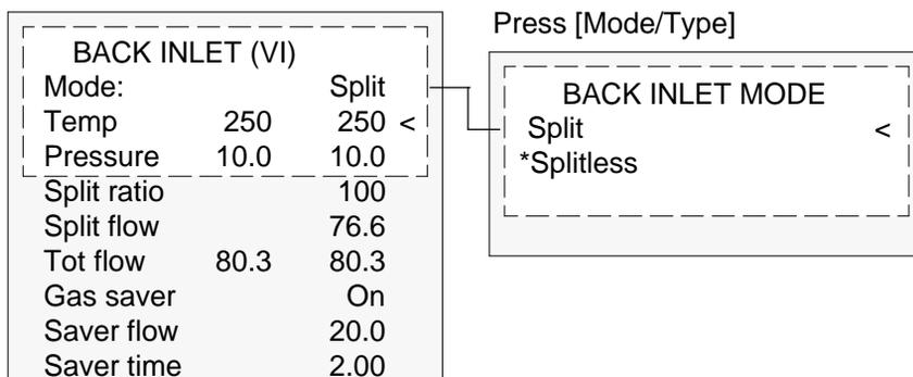
$$\text{Split ratio} = \frac{\text{Split flow}}{\text{Column flow}}$$
