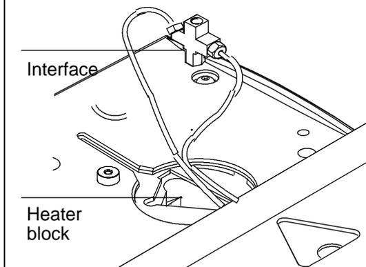
4. From inside the oven, push the column through the opening in the oven top.
