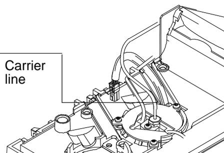
2. Remove the male nut and Vespel/graphite ferrule from the carrier line. Keep the male nut and ferrule in a safe place.
