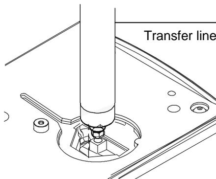
After the column is installed at both interface and detector, establish a flow of carrier gas through the interface and maintain it for 10 to 15 minutes. Check for leaks. Heat the interface to operating temperature and retighten the fittings, if necessary.
