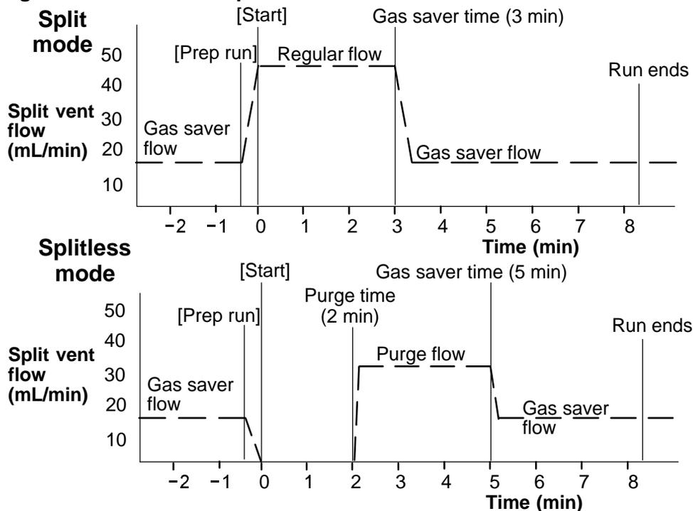
The pulsed modes of the split/splitless and PTV inlets are similar except for the pressure pulse starting at [Prep Run] and ending at Pulse time. The solvent vent mode of the PTV is more complex; see chapter 5 for details.
