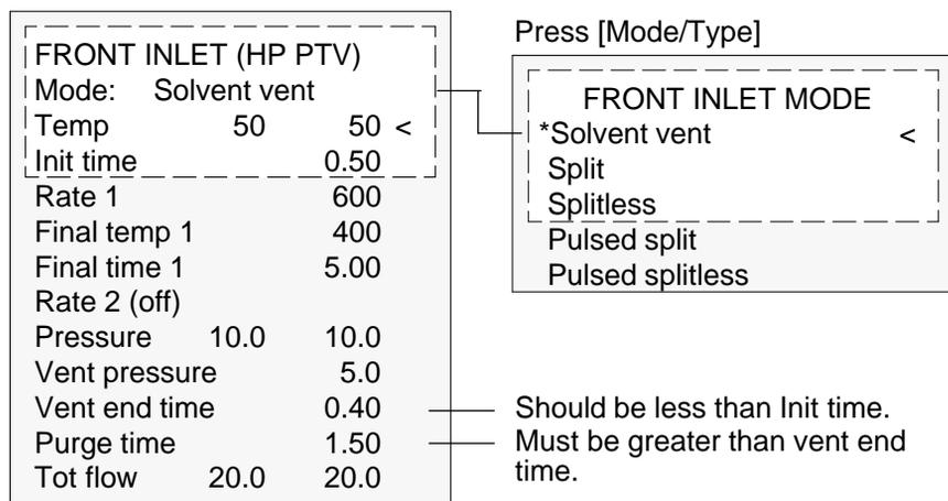
3. Press [Prep Run] (see page 13) before manually injecting a sample.
