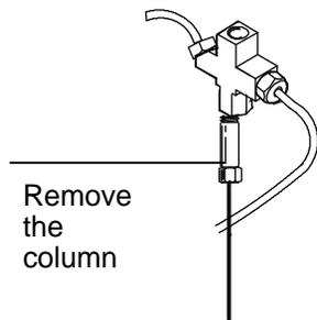
4. Remove the split and pressure sensing lines by loosening the hex nuts with the wrench.
