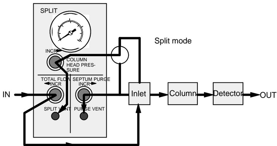
1. Locate the knob labeled TOTAL FLOW. Turn it clockwise as far as it will go. Do not force the knob; when it closes it comes to a slightly “soft” stop.
