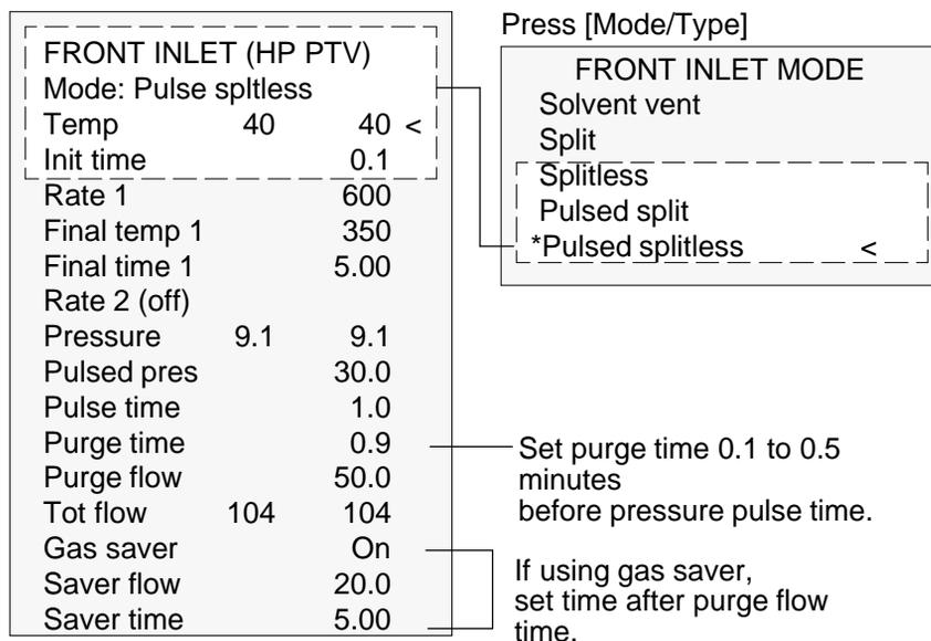
3. Press [Prep Run] (see page 13) before manually injecting a sample.
