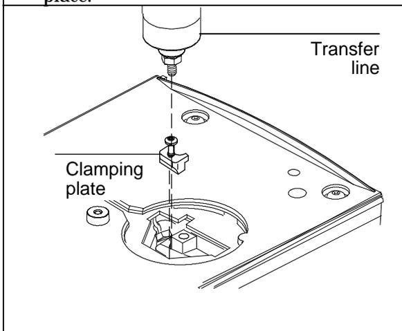
2. Lift the interface out of the heater block.
