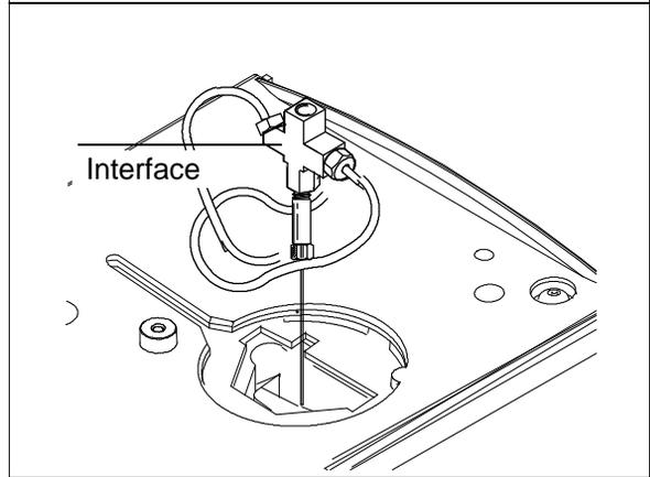
4. Loosen the the hex nut connecting the split vent line to the interface until you can remove the line. Put the line aside. You do not need to plug it.
