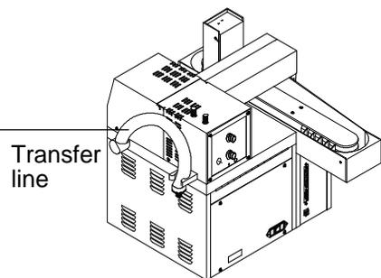
9. Connect the transfer line (with the preattached M5 nut and steel ferrule) to the interface using a 7-mm wrench. Tighten the M5 nut 1/4 turn past finger tight. Do not overtighten. If the nut leaks, tighten an additional 1/8 turn until it seals.
