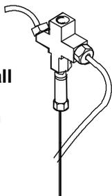
8. Place the interface in the heater block. Replace the clamping plate you removed in step no. 1 and tighten the screw until snug. Do not overtighten.
