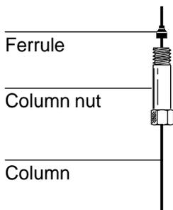
7. Position the column so it extends 6 mm above the end of the ferrule. Mark the column with typewriter correction fluid at a point even with the column nut.
