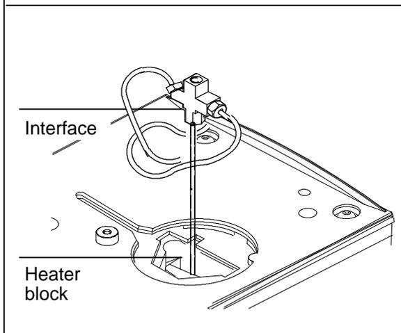
**Replacing or cleaning the interface**
