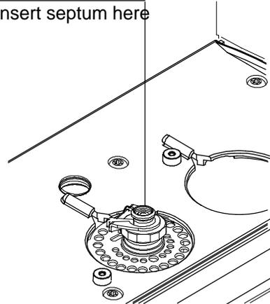
5. Replace the septum retainer nut, tightening it finger-tight until the C-ring is approximately 1 mm above the nut. When the nut is replaced, you can restore normal operating conditions.
