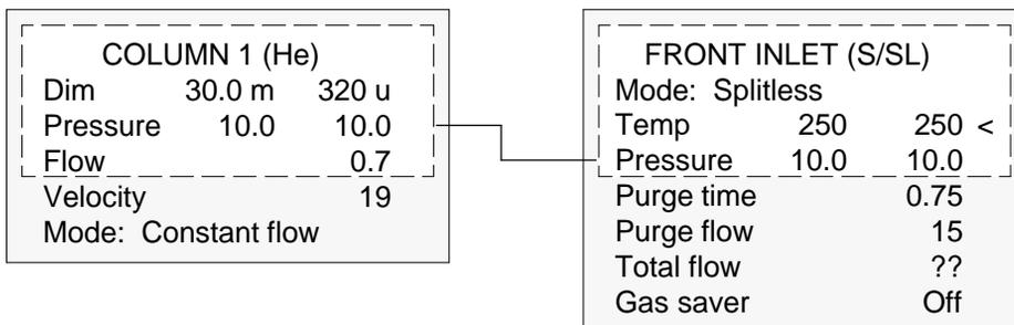
The pressure readings—both setpoint and actual—are identical on the column and inlet control tables.
