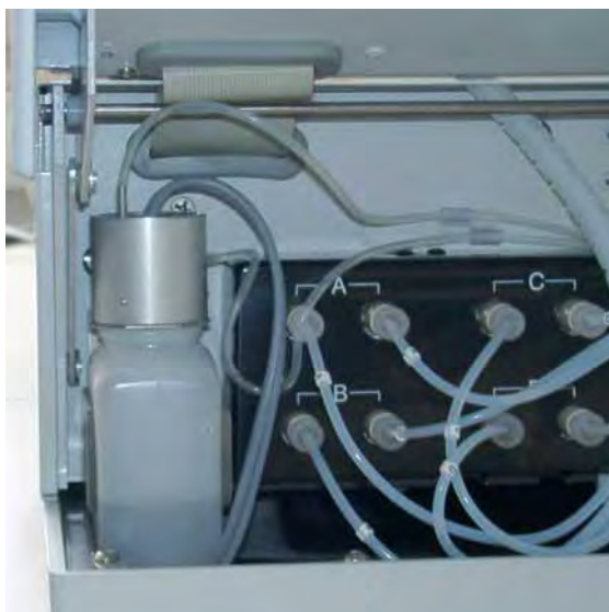
Re-insert the rear-seal wash solution reservoir.
