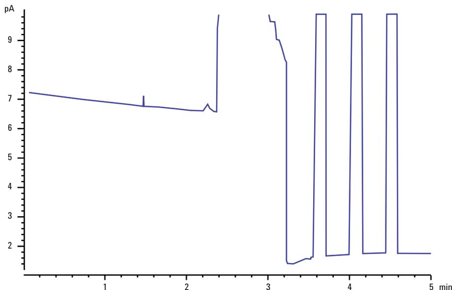
After a flameout, the GC will try to ignite the flame three times.
