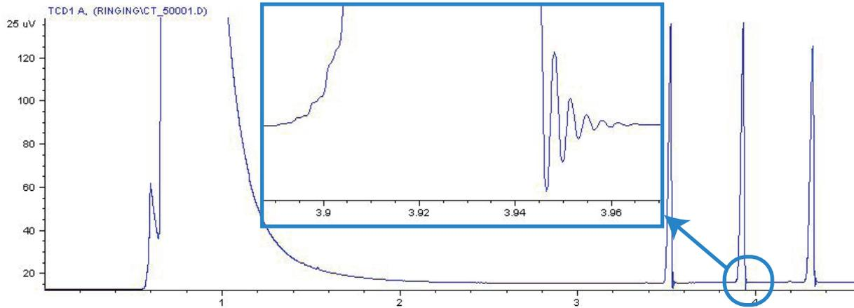
Wrong data rate is selected in the data system. For TCD, the data rate should be  $\leq 5$  Hz.
