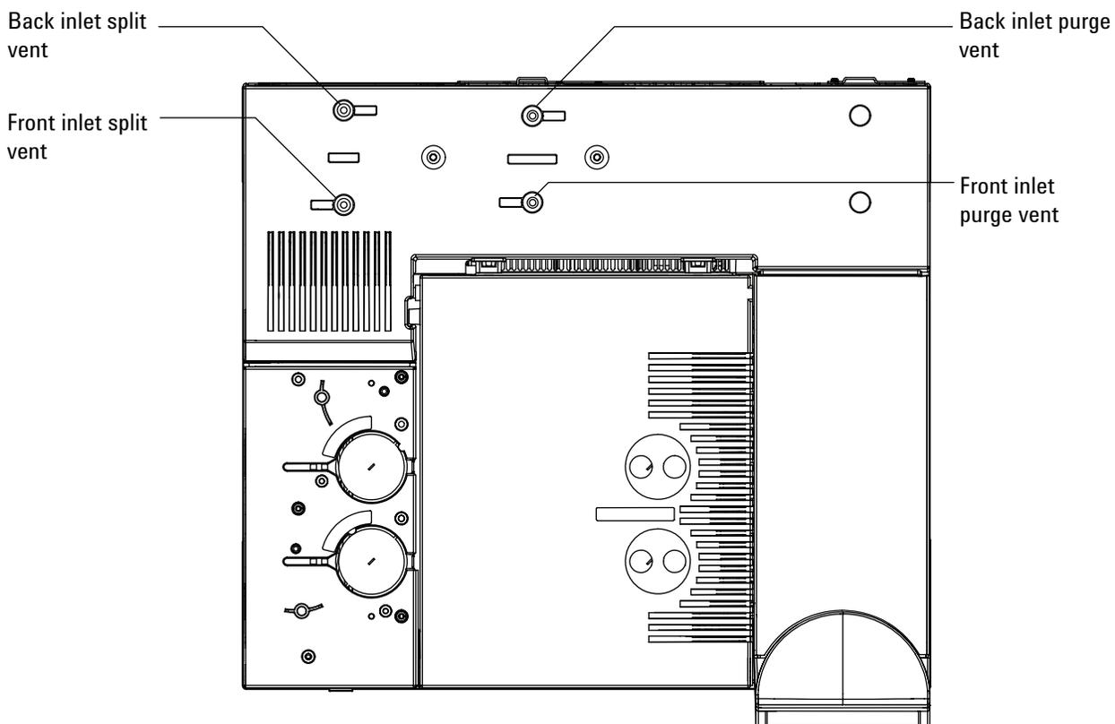
To measure split vent or septum purge flows, attach the flowmeter to the appropriate tube. Remove the GC pneumatics cover to access the back inlet exhausts.
