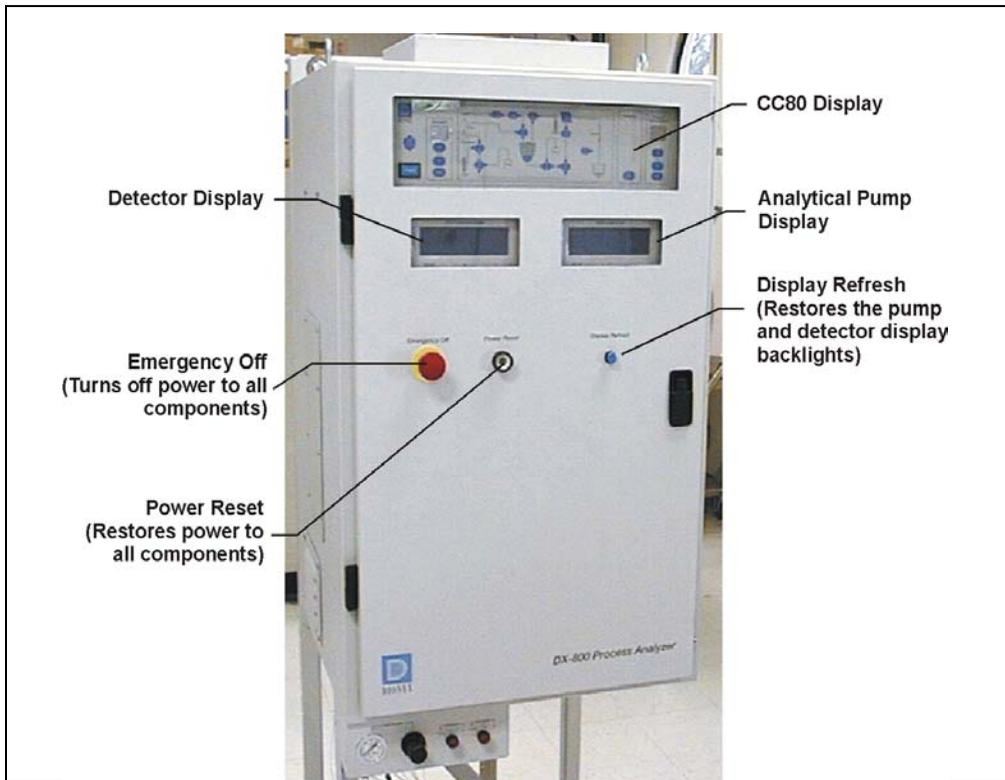
Figure 2-1. AE80 Enclosure Door
