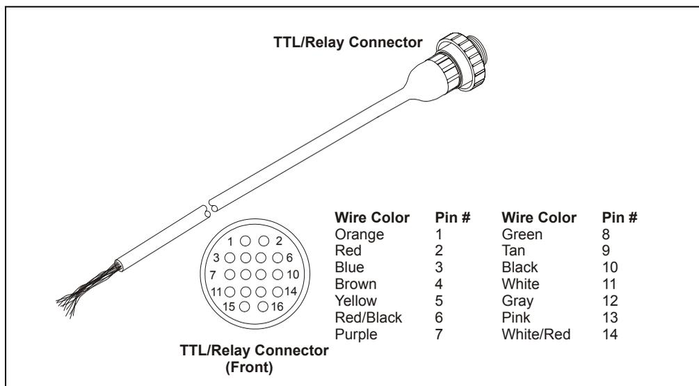
Figure 12-3. TTL/Relay Cable and Connector Pinout
