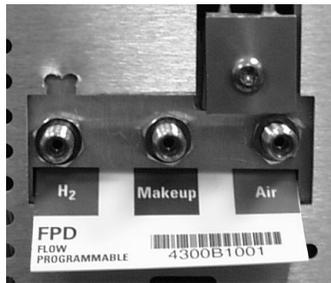
**Figure 350-19 Gas line connections**
