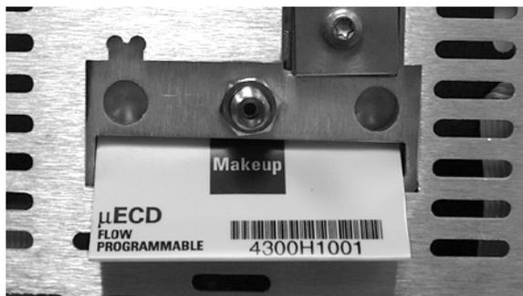
**Figure 341-14 Gas line connection**
