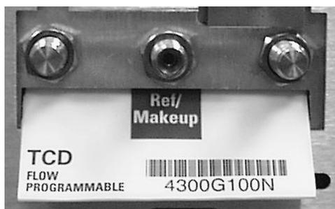
**Figure 330-18 Gas line connections**
