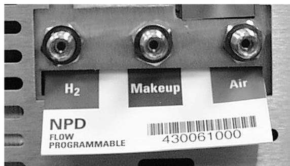
**Figure 320-16 Gas line connections**
