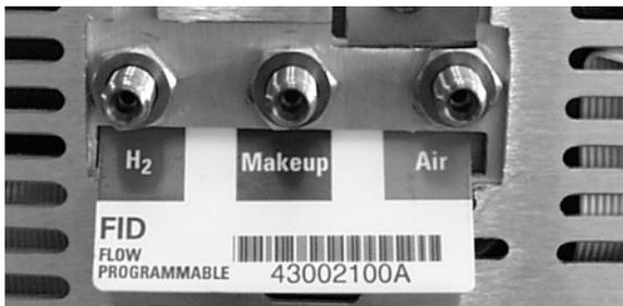
**Figure 310-17 Gas line connections**
