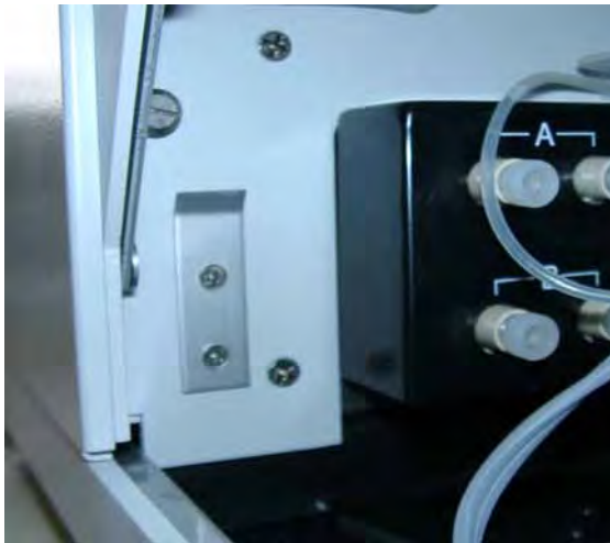
Engaging mechanism of the rear-seal wash solution reservoir.
