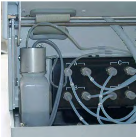
Re-insert the rear-seal wash solution reservoir.
