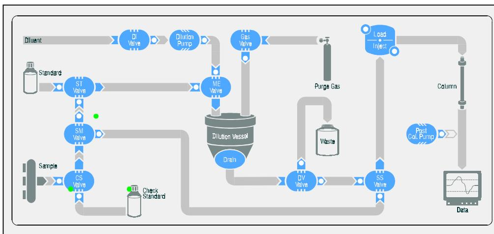
*Figure 4-2. CC82 Front Panel: SP82 for Dilution or Direct Injection*
