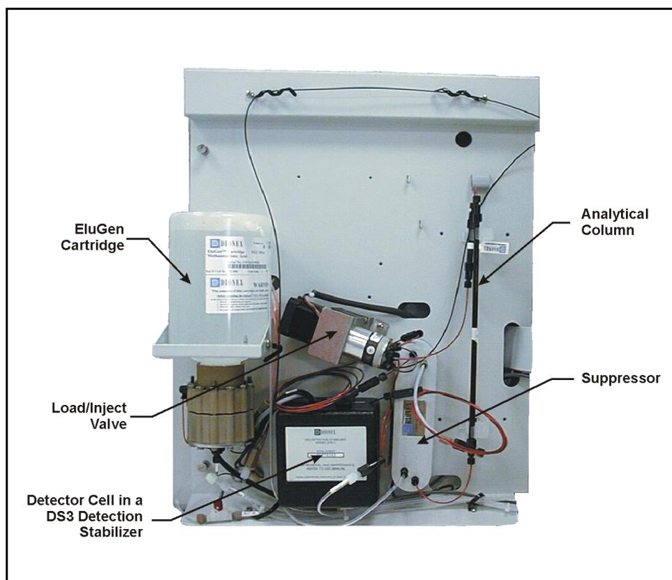
*Figure 5-1. Example LC80 Component Layout*
