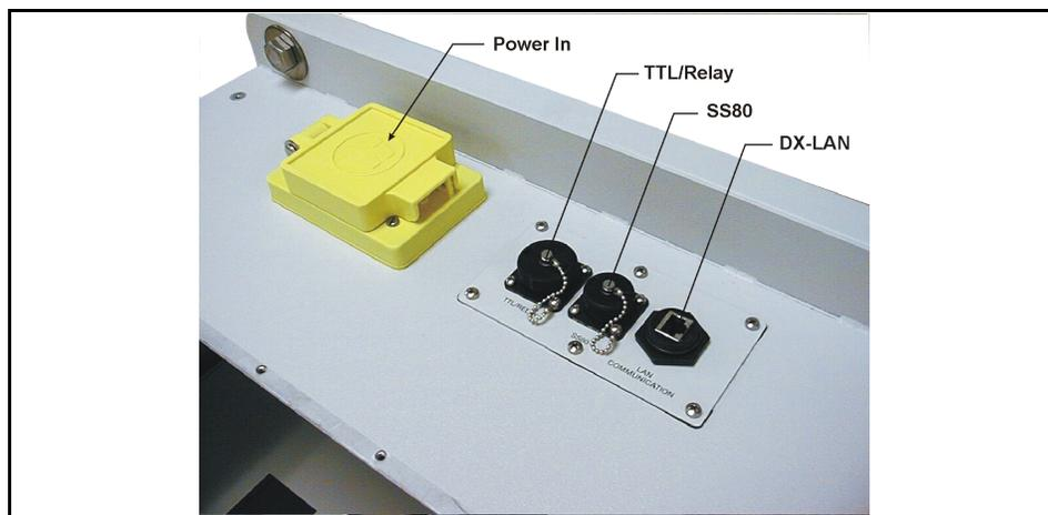
*Figure 12-3. Top View of AE80 Enclosure Electrical I/O Panel with RJ-45 Connector*
