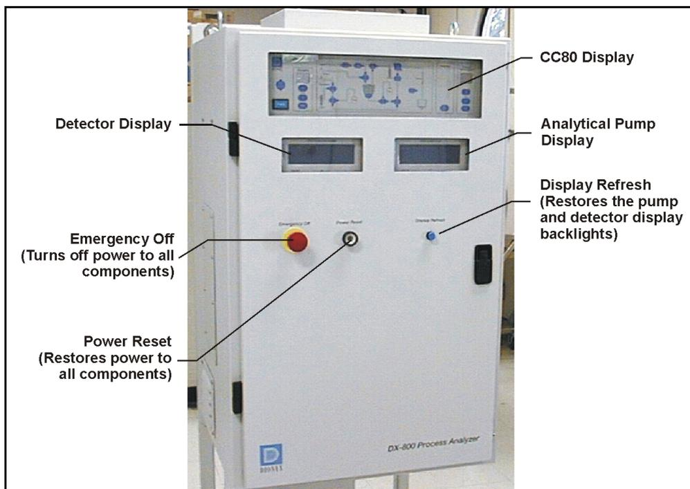
*Figure 2-1. AE80 Enclosure Door*
