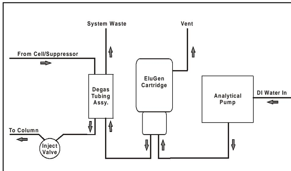
Figure 6-1. EG40-PA System Flow Diagram
