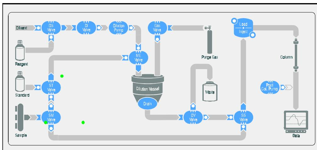
*Figure 4-3. CC83 Front Panel: SP83 for Dilution with Reagent Addition*
