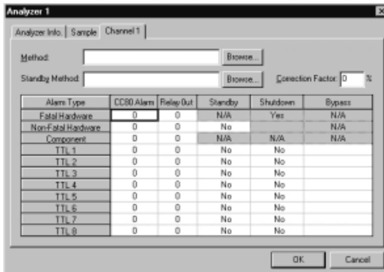
4. On the channel tab page, enter the desired action(s) for each connected TTL input. **Note:** Cells that are gray cannot be edited.
