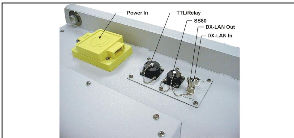
*Figure 12-2. Top View of AE80 Enclosure Electrical I/O Panel with BNC Connectors*
