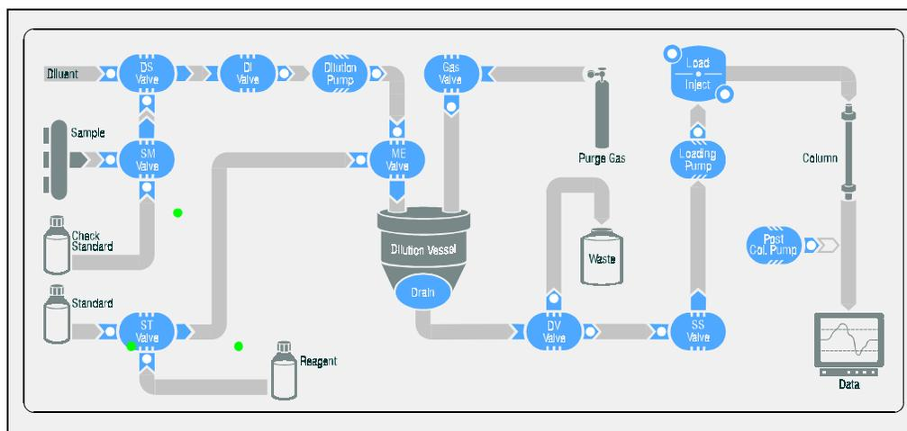
*Figure 4-4. CC84 Front Panel: SP84 for Concentration with Reagent Addition*
