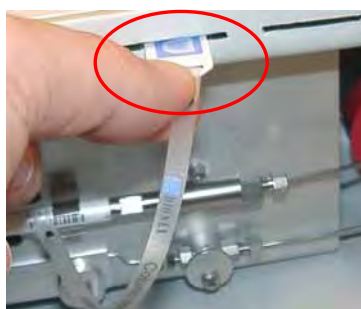
Fig. 39: Inserting the memory chip card into a column ID slot
