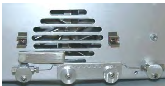
Fig. 15: Installed eluent preconditioner
