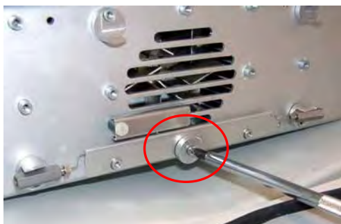
Fig. 19: Tightening the retaining screws (1)
