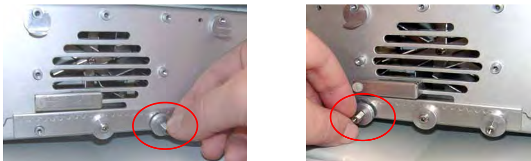
Fig. 20: Tightening the retaining screws (2)
