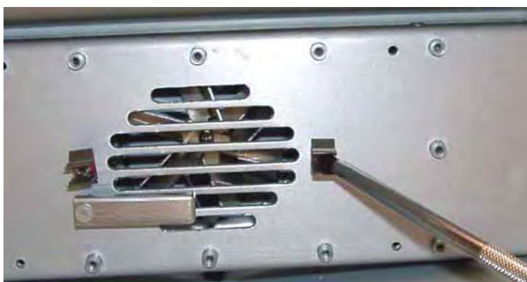
Fig. 10: Installing the column clip
