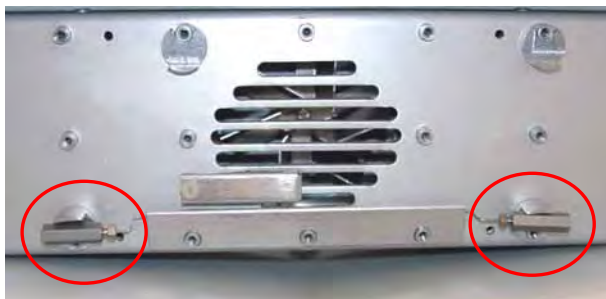
Fig. 18: Eluent preconditioner (here: 26 cm unit) inserted in the holders (bottom parts)
