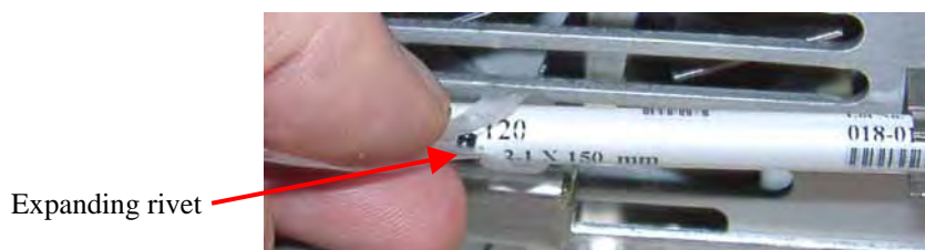
Fig. 38: Clipping the memory chip card onto the column
