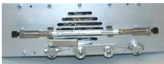
Fig. 16: Column and eluent preconditioner installed
