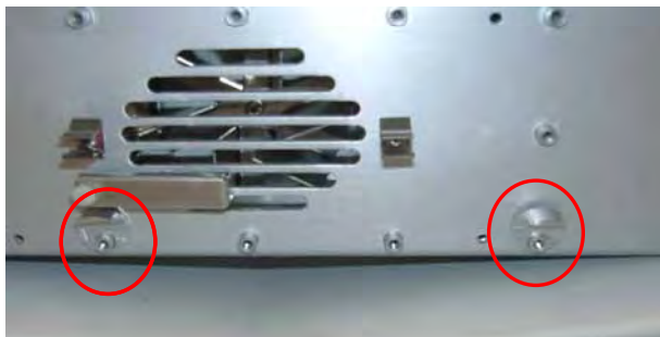
Fig. 12: Holders (bottom parts) for the eluent preconditioners
