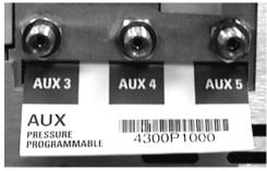
Figure 11 Gas line connections
