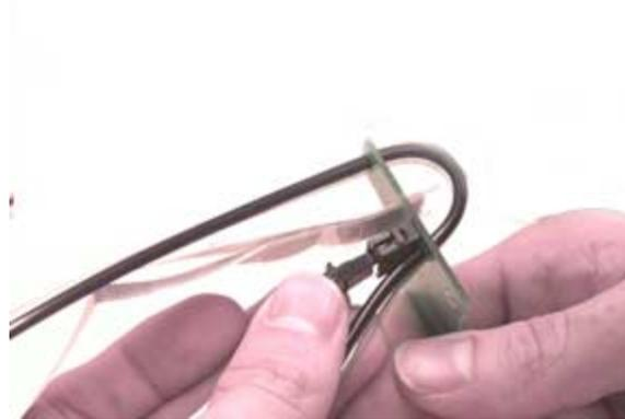
1.2.14 Press the connector on the cable not threaded through the board into J5. Tug on the cable to make sure it is latched correctly.
