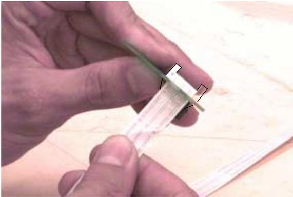
1.1.7 Pull the flex cable back so that the stop comes in contact with the board.
