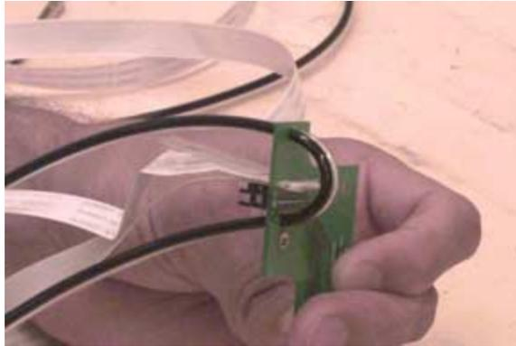
1.2.13 Now push the end of the tubing, being careful to insure that it's not twisted, through the top slot on the board. Pull 27½" through.
