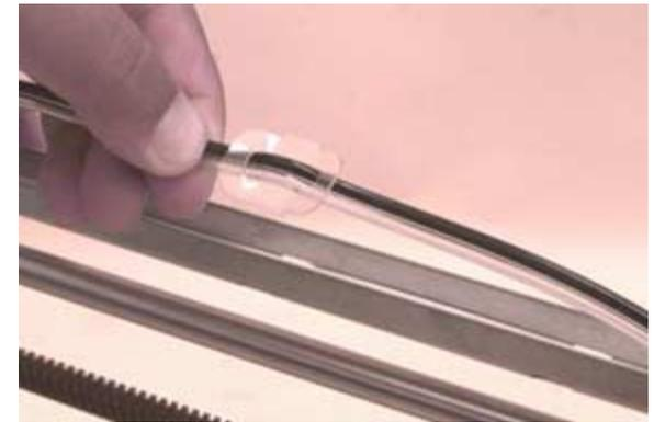
1.1.9 Install three Cable Retainers (DY-700117-01) onto the tubing and attach to slotted holes on the Cable Support.
