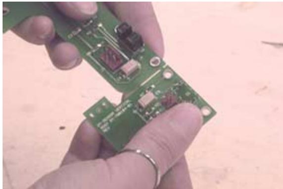
1.2.1 Break the Sensor Board, DY-700104-01, in half.
