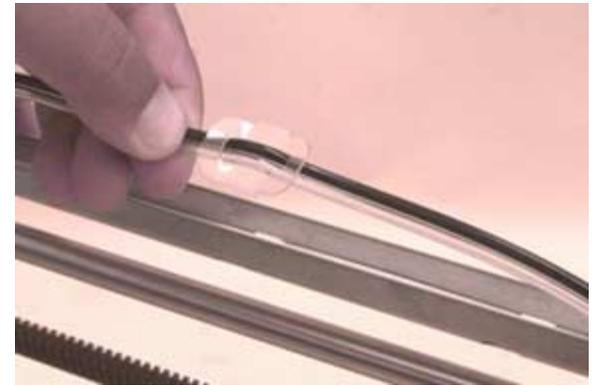
1.2.9 Install three Cable Retainers (DY-700117-01) onto the tubing and attach to slotted holes on the Cable Support.
