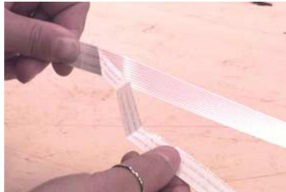
1.2.2a Stretch out the ribbon cable, DY-700109-00, in the region where it's folded, so that it is flat.
