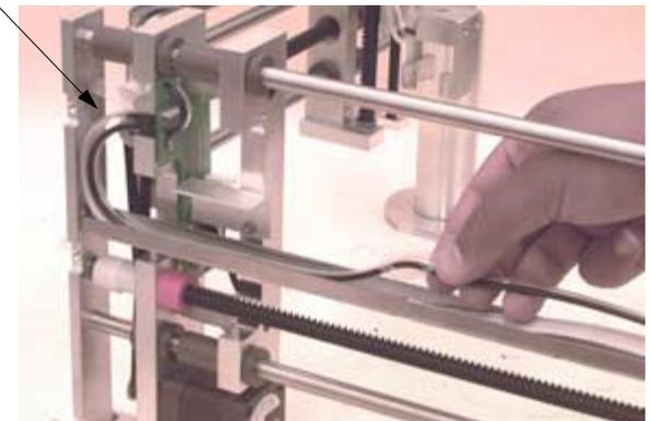
1.1.21 Disconnect connector from *J-1* and install another tie wrap from bottom of the pc board. Reattach connector to *J-1*.
