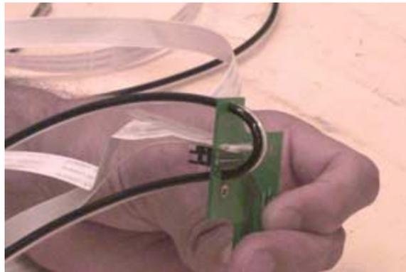
1.1.4 Now push the end of the tubing, being careful to insure that it's not twisted, through the top slot on the board. Pull 27½" through.
