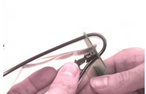
1.1.4b Press the connector on the cable not threaded through the board into J5. Tug on the cable to make sure it is latched correctly.
