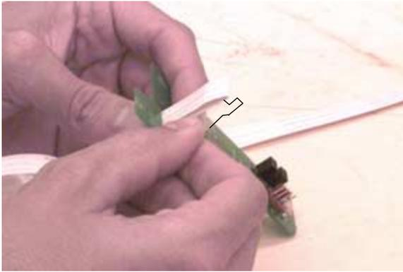
1.1.6 Break the Cable Anchor, DY-700132-01, in half.
