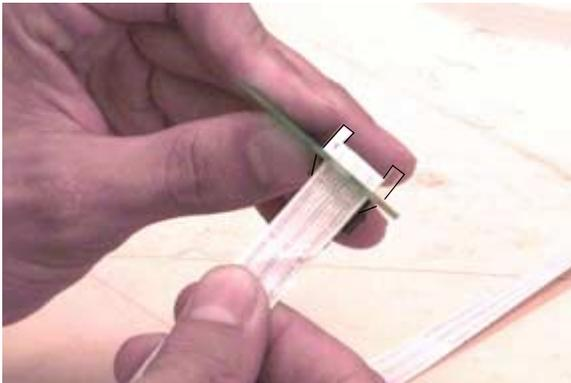
1.2.6 Pull the flex cable back so that the stop comes in contact with the board.
