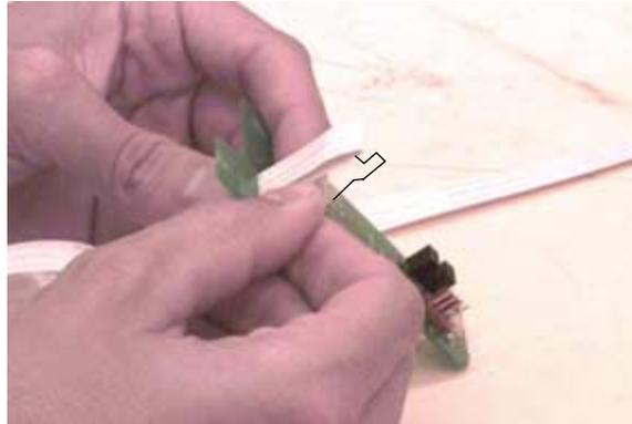
1.2.4 Break the Cable Anchor, DY-700132-01, in half.
