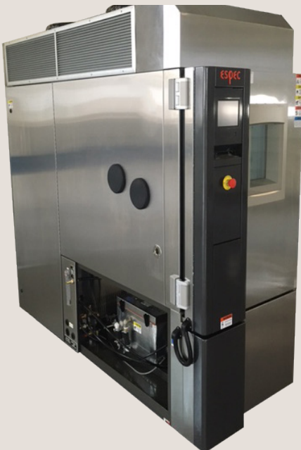
Espec Environmental Chamber -70 to 180°C ; 10-95% RH
