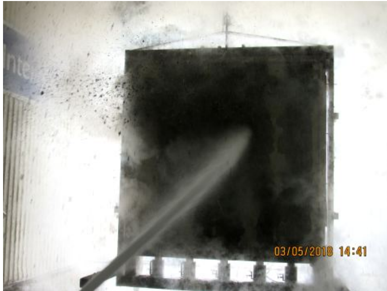
Photo No. 36 Hose Stream Test
