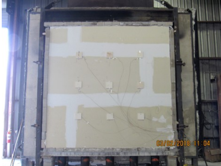
Photo No. 18 Start of Test (Stucco Exposed)
