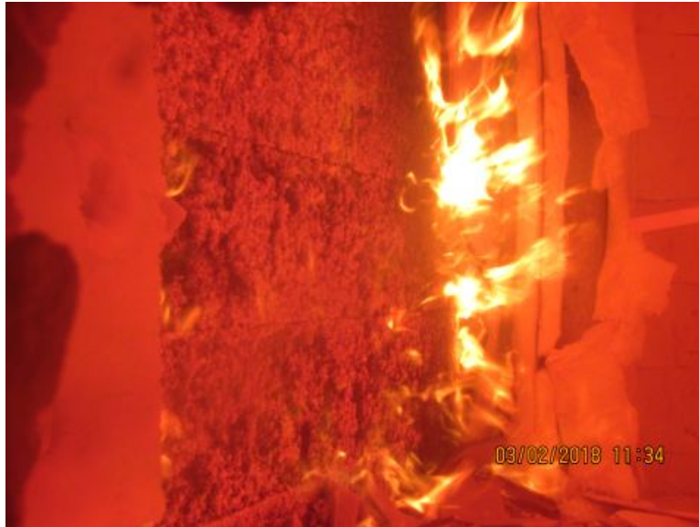
Photo No. 20 Flaming of Wall After Stucco Falls (Exposed Side)
