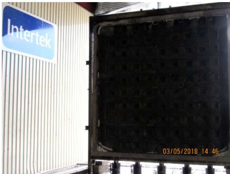
Photo No 37 Post Hose Stream Test
