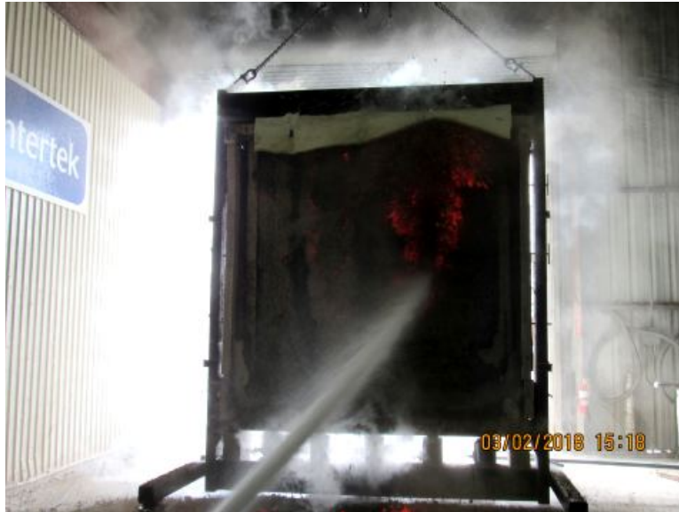
Photo No. 24 Hose Stream Test
