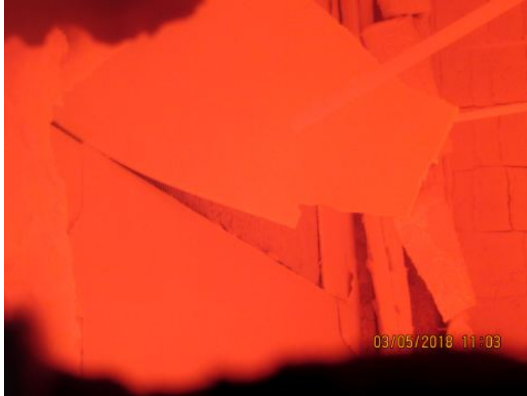
Photo No. 28 Exposed Side View of Gypsum Board Falling Off
