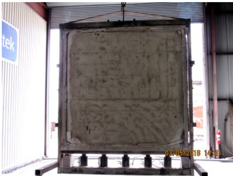
Photo No. 35 Pre Hose Stream Test
