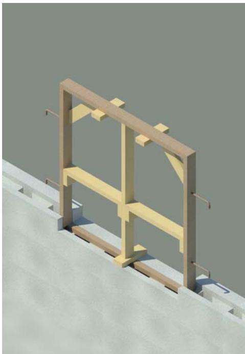
After placing the third course, the third course is a good place to begin to set the door and window bucks. Note that the 4040 window sill is at 32", and the top of the third course block must be cut down 4" to have the door and window head heights align.
