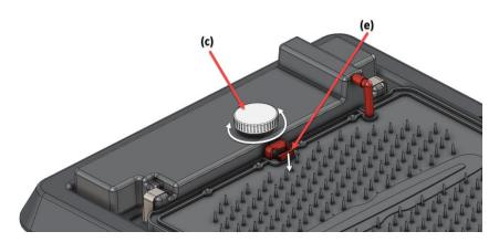
Step 4. Open/lift up red shut off valve (e) and allow tray to fill with IPA (fill takes 1 to 2 minutes) then close red valve (down position). The recommendation is to leave red valve (e) closed until after many uses and alcohol no longer comes through the holes onto your soles. Repeat step 4 to fill again. This will keep the alcohol preserved in the reservoir until it is needed and will reduce evaporation.
